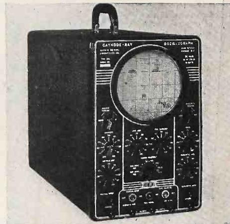
range from 20 to 50,000 cycles uniformly within 20%. There is provision for intensity modulation. The input impedance of the vertical plates are 5 megohms at 50 mmf direct, and 1 megohm at 40 mmf through the amplifier, while the horizontal impedances are 5 megohms at 60 mmf direct, and 5 megohms at 40 mmf amplified. Allen B. DuMont Laboratories Inc., 2 Main Ave., Passaic, N.J.—RADIO & Television RETAILING
