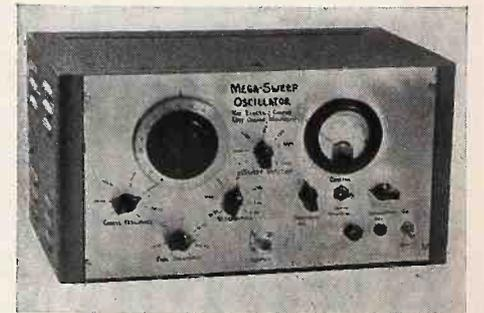
The Mega-Sweep oscillator has a carrier frequency range from 50 kc to 500 mc, with an adjustable sweep from 30 kc to 30 mc broad. An output of .1 volt at a 50-ohm level is controlled by a continuously variable attenuator. The amplitude modulation while sweeping is kept to .15 db per megacycle. Kay Electric Co., East Orange, N. J.—RADIO & Television RETAILING
