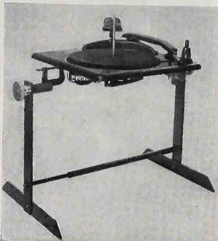
Any record changer, and most radio chassis, can be supported at any angle for work at the service bench, as well as on outside calls. Weighing 11½ lbs., the new rack is made to assemble and disassemble quickly. Friend's Radio Co., 9 N. Seventh St., Philadelphia 6, Pa.—RADIO & Television RETAILING
