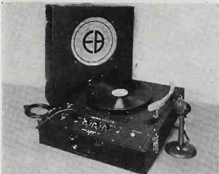
stand and 25' of mike cable, all of which are included in the set. The bottom part of the case contains a dual-speed turntable for playing up to 16" records, and a 12-watt amplifier having mike and phono input mixer controls. An automatic changer may be ordered instead of a manual player. Riggs & Jeffries Inc., 73 Winthrop St., Newark 4, N. J.—RADIO & Television RETAILING
