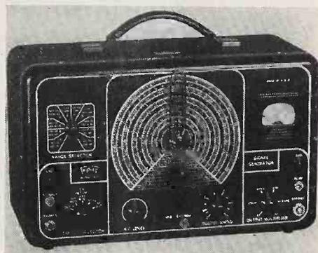
Model 1632 is an amplitude modulated signal generator covering from 100 kc to 120 mc in 10 ranges. The panel meter indicates the output of the multiplier and attenuator. Provision is made for internal mounting of a 1000 kc crystal, for heterodyne frequency calibration. Air trimmers, permeability tuned coils and a voltage regulator tube are included for stability. Triplett Electrical Instrument Co., Bluffton, Ohio—RADIO & Television RETAILING
