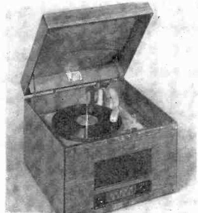
Model 202 radio-phonograph table unit, ac-dc superhet, 6 tubes including rectifier, automatic record changer playing twelve 10" or ten 12" discs. Tunes 550 to 1700 kc, built-in loop antenna, automatic volume control, slide rule dial, Alnico 5 PM speaker. Cabinet of walnut veneers measures 12" by 15 1/2" by 16 1/2". Weighs 27 lbs. Apex Radio & Television Corp., 192 Lexington Ave., New York 16, N. Y.—RADIO & Television RETAILING
