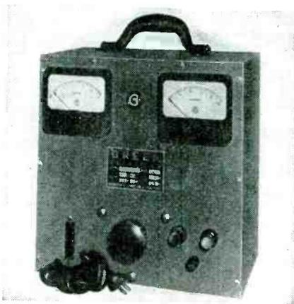
A new portable rectifier has an adjustable output from zero to 6 volts dc, with a continuous current capacity of 25 amperes. This 150-watt bench unit, model 72S1C, uses a full wave selenium rectifier, a magnetic circuit breaker on-off switch in the input, a variable voltage-control transformer, and output current and voltage meters. W. Green Electric Co., Inc., 130 Cedar St., New York, N. Y.—RADIO & Television RETAILING
