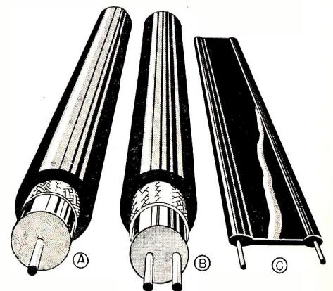
Fig. 3. Three common types of transmission lines. At A, RG-8/U coax; at B, RG-22/U coax; at C, 300 ohm twinlead. Text explains use.
