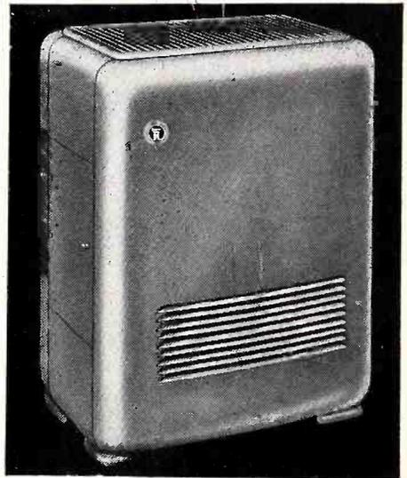
**Oil Console**—welded aluminum cabinet finished in neutral baked enamel. Lights easily as a candle. Produces 50,000 to 65,000 B. T. U. Radiant flame, high-low, vaporizing type burner. Combustion chamber of high tensile steel, seam-welded. Two sizes, largest 31" wide, 39" high, 23" deep. Burns light fuels up to No. 2. Shipped completely assembled. Available as extras are pan-type humidifier, rear-mount fan with switch, 5½-gallon attachable fuel tank. Approved by Commercial Standards and U. L.
