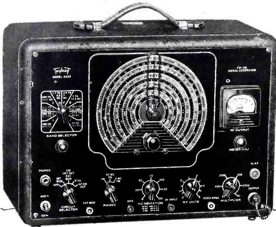
For Ranges from 165 K.C. to 120 M.C. Select the Signal Generator
