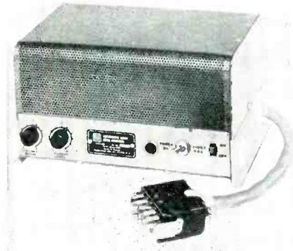
With the ALC a constant, high-definition picture is assured regardless of any sharp or sudden changes in the light source. It is especially suited for use out of doors. Blonder-Tongue Laboratories, Inc., Westfield, N.J. (ELECTRONIC TECHNICIAN 1-31)
