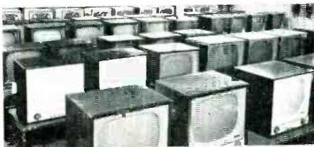
Sylvania deflection tubes are testing in stock models of representative TV manufacturers. Tests are conducted at accelerated line voltages so that tubes are operated at a considerably high level. These
