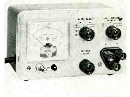
30 volts output. A line voltage change of ±10% causes output change of less than ±0.2% or ±15 mv, whichever is greater. The output voltage temperature coefficient is approximately 0.2% per °C, 24°C to 50°C. Hewlett-Packard Co., 275 Page Mill Rd., Palo Alto, Calif. (ELECTRONIC TECHNICIAN 5-30)
