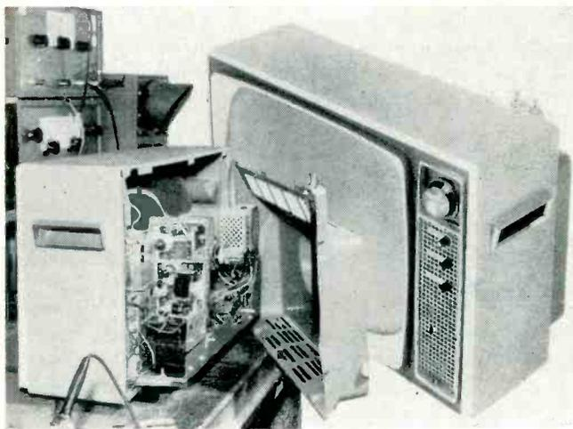
New GE "Designer Series" TV gives shallow appearance, while providing increased service accessibility. The 21" set is 15 $\frac{3}{4}$ " deep, including 7 $\frac{3}{4}$ " cabinet. The conventional flat back has been replaced with a formed steel back, which exposes the vertical chassis sides.
