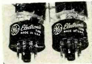
Tapered Pins on octal-base receiving tubes save time and avoid socket damage when inserting in hard-to-reach spots.
