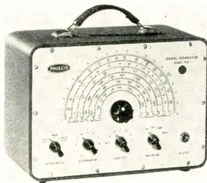
mitting an accurate adjustment to all frequencies, high r-f output making possible extreme accuracy in checking single stages, and uniform modulation for checking gain and distortion. Philco Accessory Div., "C" and Westmoreland St., Philadelphia 34, Pa. (ELECTRONIC TECHNICIAN 9-13)
