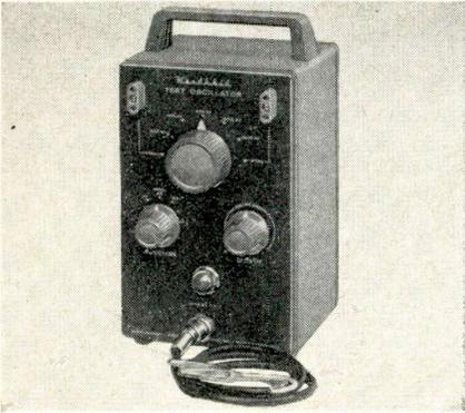
modulated, 400 cps modulated, or audio used separately. Output level is adjusted by continuously variable control. Construction is simplified through use of a pre-assembled and aligned frequency selector switch. \$16.95. Heath Co., Benton Harbor, Mich. (ELECTRONIC TECHNICIAN 9-15)
