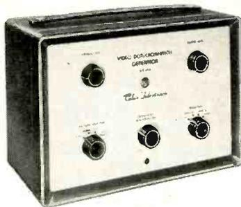
**WR-46A VIDEO/DOT CROSSHATCH GENERATOR** for making static and dynamic convergence adjustments in color-TV sets.
