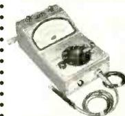
**208VTVM**—" Fool-proof"—many new features! Easy-to-read 4½" 200 microamp meter mounted on sloping panel—7 DC, 7 AC, 7 ordinary Ohm ranges, plus RETMA (EIA) Ohm scale to check standard color-coded resistance values and tolerance limits. Specially designed "shift-lever" type function switch identifies and automatically connects proper probe. With stand, 40" leads, and common lead with clip.
