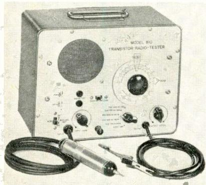
tor covers same ranges. Transistor tester checks leakage and gain. Loud-speaker is an indicator for signal tracing. This Model 810 in portable steel case. 105-125 v. ac. Hickok Electrical Instrument Co., 10523 Dupont Ave., Cleveland 8, Ohio. (ELECTRONIC TECHNICIAN 9-10)
