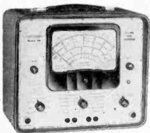
**the Model 98** Laboratory VTVM with 7" Meter
