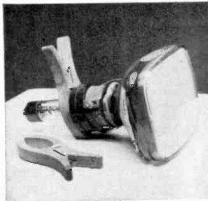
Large wooden clothespins, such as used by electricians and linemen may be modified to support both the yoke and test CRT.
