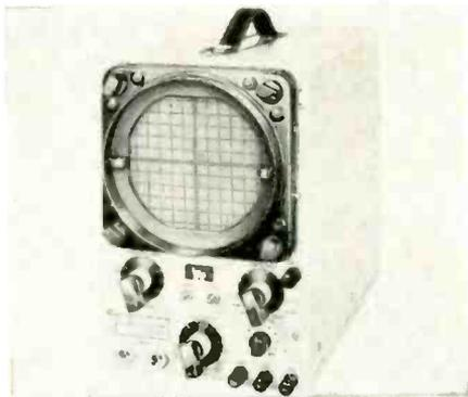
scopes. Features d-c to 7 mc response, wide range repetitive sweep and ease of operation. Conveniences for the technician include: "Two line-Two Frame" positions on the horizontal sweep, trace inversion, direct vertical calibration and hi-sensitivity vertical amplifier. \$245. Waterman Products Co., 2445 Emerald St., Philadelphia 25, Pa. (ELECTRONIC TECHNICIAN 8-28)
