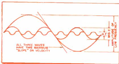
Fig. 1—At a constant voltage, signal amplitude increases as frequency decreases.
