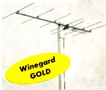
**TRANSCOULER YAGIS — NEW SUPER EFFICIENT TRANSCOULER YAGIS 3, 6, 12 ELEMENT.** Absolutely the most efficient cut-to-channel and broad band yagis ever built. Use a three element where a five was used, a six for a ten, and a twelve for really tough reception problems. Unique Transcoupler bars swing into position for perfect 300 ohm match and simplest stacking ever devised. In stacking, 100% of power is delivered from both bays. Bright Gold Anodized, wide spaced design. 42 different models.
