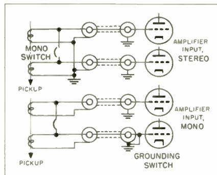
Fig. 1—It is possible to place a dead short across the phono input being used if the preamp's selector switch grounds all unused inputs and a changer or turntable has a paralleling cartridge terminal switch for playing monophonic discs. If both the preamp and changer or turntable can be switched to a monophonic position, it is advisable to render one switch inoperative.
