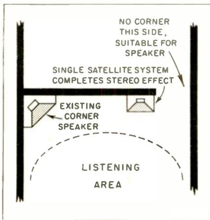
Fig. 4—An original monophonic speaker system is converted for stereo use by adding two satellite speakers. The center speaker carries bass frequencies of both channels.
