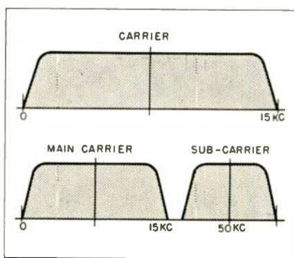
Fig. 3—Restricting the deviation of the main programs leaves room for one or more sub-carriers to carry additional programs.
