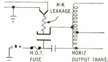
H-K leakage in a damper tube which has its heater grounded may cause the H.O.T. fuse to blow.
