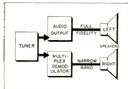
Fig. 4—The Halstead stereo receiver proposal includes a wide-band and low-band channel.
