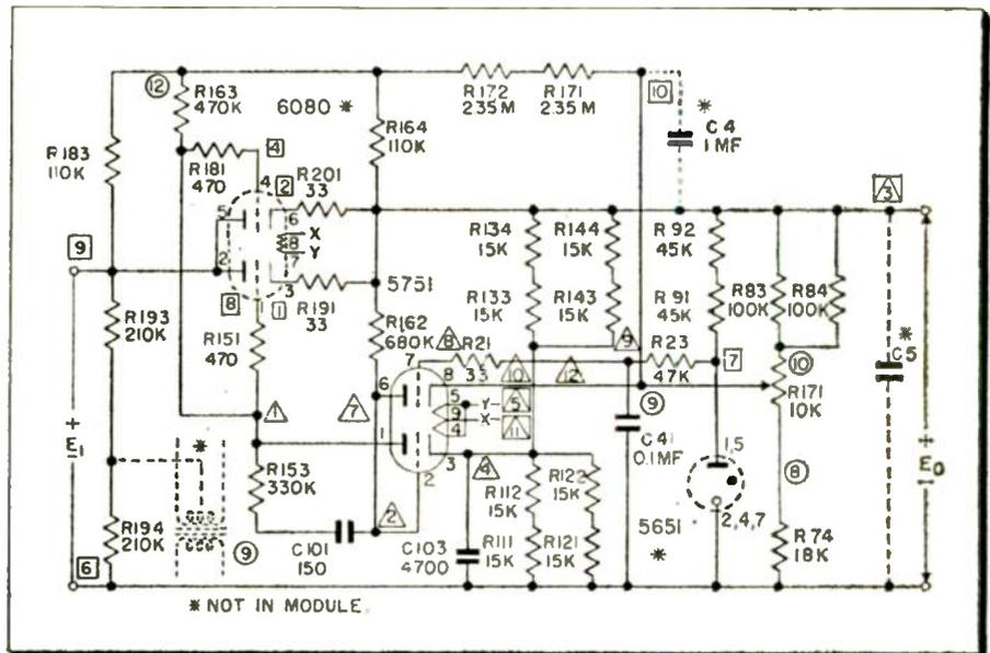
Fig. 4—The voltage regulator circuit illustrated has a 300 v d-c input between terminals 6 and 9. The tube socket and most of the components are on the module shown in Fig. 2B.
