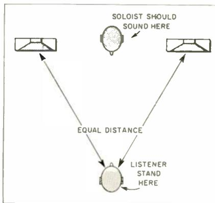
Fig. 2—A soloist's voice should appear to come from the center when the speaker outputs are properly phased and balanced.
