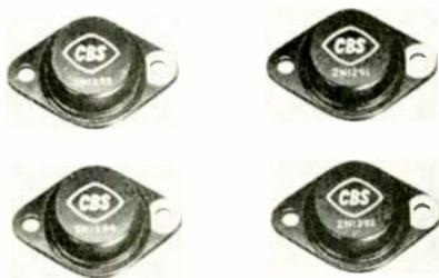
Negative feedback can be more easily applied using them. The pairs feature high voltages—up to 100 v., and proven reliability (exceeding MIL-T-19500A) for audio, control, voltage-regulation, servo and computer applications. CBS Electronics, Semiconductor Operations, 900 Chelmsford St., Lowell, Mass. (ELECTRONIC TECHNICIAN 9-10)
