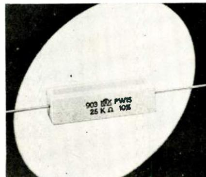
soldering, secured to a resistance element, wound on a glass fibre core and sealed in a rectangular case. Materials are inorganic for fullest protection against flame or decomposition at overload conditions. International Resistance Co., 401 N. Broad St., Philadelphia 8, Pa. (ELECTRONIC TECHNICIAN 9-7)
