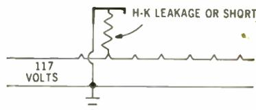
An H-K short circuit, or low-resistance leakage, in a series-string tube, short-circuits part of the heater circuit. The resulting higher voltage across the remaining heaters may cause heater burnout.
