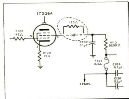
Fig. 3—Inserting a 120 ohm resistor in the 17DQ6A's screen grid of RCA series 800 TV sets will remedy parasitic oscillations.
