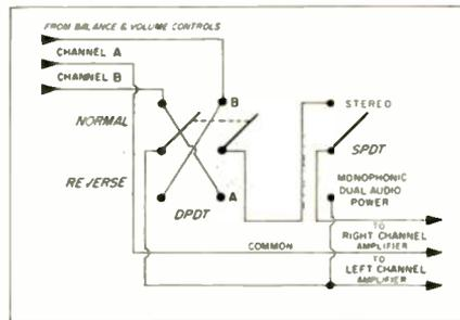
Fig. 3—A SPDT switch offers versatility for stereo control. The listener can change from stereo to mono and can feed either channel into both amplifiers and speaker systems.
