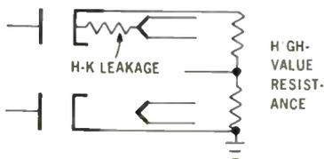
In detector, discriminator, and AFC stages, which usually have relatively high values of resistance in the cathode circuit, even a slight amount of H-K leakage current can easily cause visible and/or audible 60-cycle "hum" symptoms.
