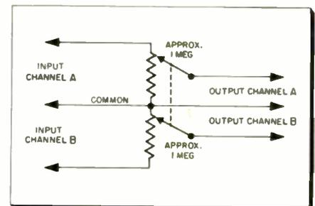
Fig. 4—A balance control is needed when playing stereo material in order to equalize the sound from both channels. The dual linear control is wired in reverse order so that when one level goes up, the other goes down.
