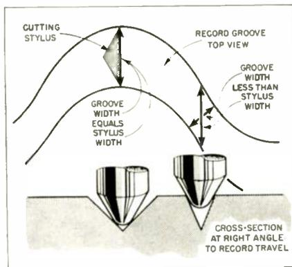
Fig. 4—The sidewise motion of the cutter results in a narrower groove with respect to the playback stylus whenever the groove is laterally modulated. The narrower groove pinches the stylus, causing it to rise and fall. Since stereo cartridges reproduce the vertical component as well as the horizontal one, lateral modulation increases distortion in the vertical component.
