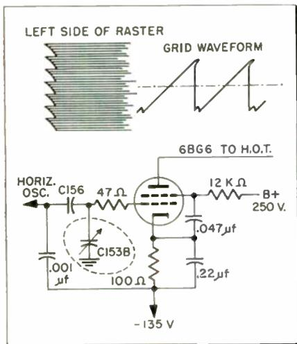
Fig. 1—A partially shorted drive capacitor produced a strange raster pattern that concentrated on the left side of the screen.
