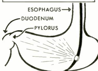
Lamp located at end of gastroscop, has a flexible rubber finger that guides end of instrument across floor of stomach while the lamp illuminates wall of stomach for viewing through gastroscop. Even color pictures can be taken through the instrument!
