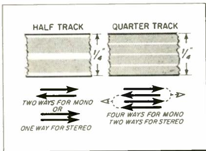
Fig. 1—The development of quarter-track tape doubles playing time offered by half-track tape and brings pre-recorded tape prices into closer competition with records.
