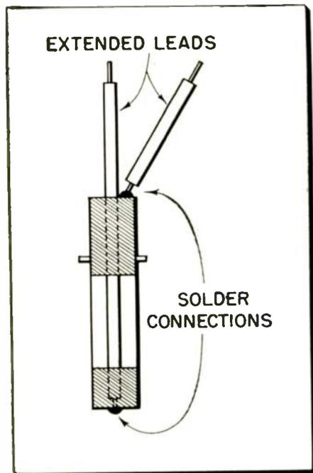
Fig. 1—Modified "twist-lock" fuses, as shown, will enable the technician to measure current without removing the TV chassis.
