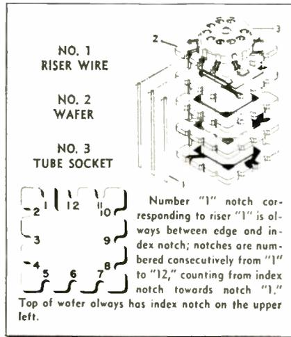
Fig. 1—Correct module mounting is simplified by a notch between risers 1 and 12.
