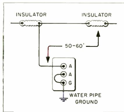
Fig. 2—A low-directivity antenna is usually satisfactory for reception on all bands.
