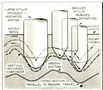
large to trace complex stereo record grooves. The RIAA recommends a 0.5 mil stylus for best stereo reproduction. However, a 0.7 mil stylus is the currently popular radius size, chosen as a necessary compromise due to some unsurmountable problems at the present time.
