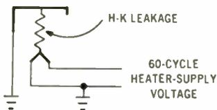
H-K leakage provides a path for 60-cycle current to flow from the heater to the cathode. If there is no resistance or impedance in the cathode circuit, this leakage current usually causes no difficulty.
