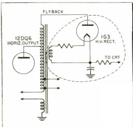
before the output transformer, if for no other reason than that they are easier to check than the flyback itself. Red hot plates in the horizontal output tube may indicate an absence of drive, or an excessive cur-
