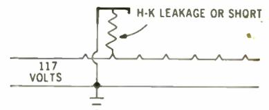
An H-K short circuit, or low-resistance leakage, in a series-string tube, short-circuits part of the heater circuit. The resulting higher voltage across the remaining heaters may cause heater burnout.
