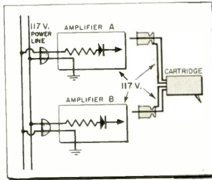
Fig. 3—Some a-c/d-c equipment and cartridges may present a possible shock hazard.
