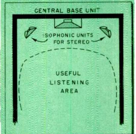
Fig. 6—System shown takes advantage of open-back, satellite-type speaker enclosures to provide increased sound dispersion.
