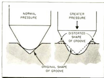
Fig. 2—A larger stylus is liable to bounce out of the groove because it is riding on the upper portion of the disc's sidewalls.
