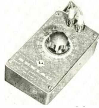
decade-type substitution box contains a selector switch enabling interchange of any one of the 11 component diodes. The original Model A, 1-watt Zeniac and the new 10-watt Model B Zeniac are now available. International Rectifier Corp., 1521 E. Grand Ave., El Segundo, Calif. (ELECTRONIC TECHNICIAN 9-26)
