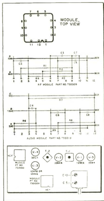
Fig. 11—Most of the resistors and capacitors in an Emerson radio Model 851B are contained in just two modules. The a-f module has three decks and the r-f two decks.
