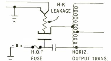
H-K leakage in a damper tube which has its heater grounded may cause the H.O.T. fuse to blow.
