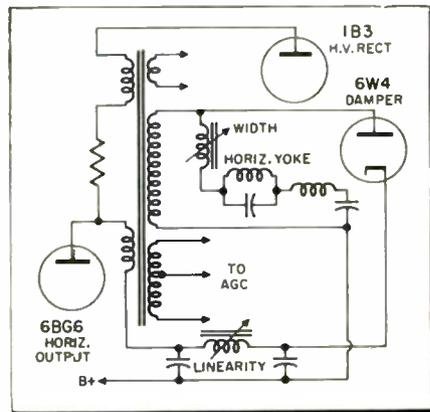
Fig. 3—A defective external circuit such as the damper, yoke, width, etc., can load down the circuit and kill the high voltage.
