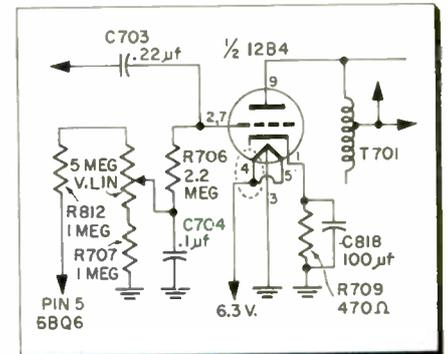
Fig. 2—Missing filament socket pin No. 4 cut the heater voltage in half and resulted in insufficient current flow. The inadequate current affected the TV set's height.
