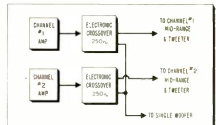
Fig. 5—Crossover networks inserted between the amplifiers and speakers removes the bass component from each channel and directs it to the system containing the woofer.
