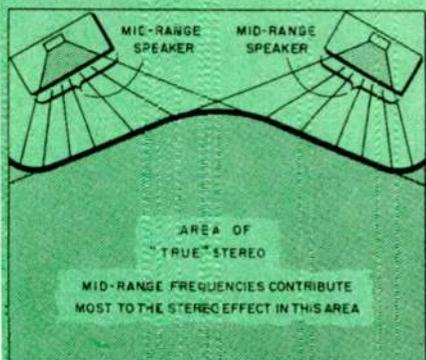
Fig. 1—This basic speaker placement approach provides a wide stereo listening area in large rooms. Placing speakers parallel to the listener would necessitate closer spacing to achieve the proper effect.
