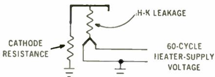
When there is resistance in the cathode circuit, the H-K leakage current develops a 60-cycle voltage across the cathode resistor. This voltage may produce visible and/or audible 60-cycle "hum".
