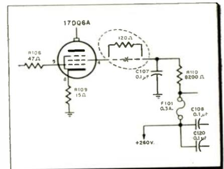
Fig. 3—Inserting a 120 ohm resistor in the 17DQ6A's screen grid of RCA series 800 TV sets will remedy parasitic oscillations.
