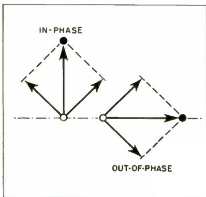
Fig. 2—In-phase mechanical forces result in out-of-phase electrical signals. Conversely, out-of-phase mechanical forces cause in-phase electrical signals. This conforms with the RIAA requirement of deriving an in-phase signal from a horizontal motion. Bass frequencies are essentially in-phase signals and therefore will be found mostly in the horizontal component of the disc.
