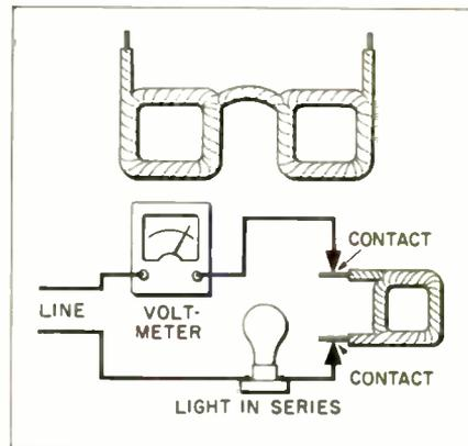
Fig. 2—Field coils may be accurately tested under operating conditions as illustrated.
