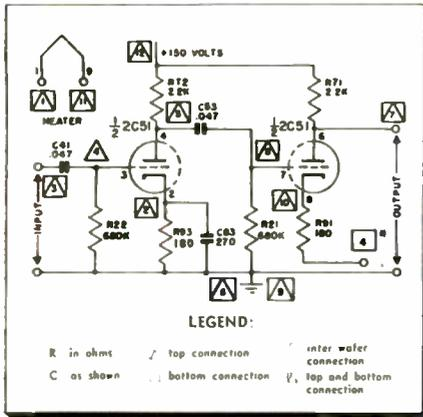
Fig. 3—The legend accompanying the intermediate video amp module (Fig. 2A) circuit aids in identification of riser terminals.
