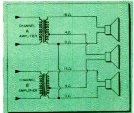
Fig. 5—Establishing a third channel. While this doesn't add anything to bass response, it does improve directional sense with respect to the center of the program source.
