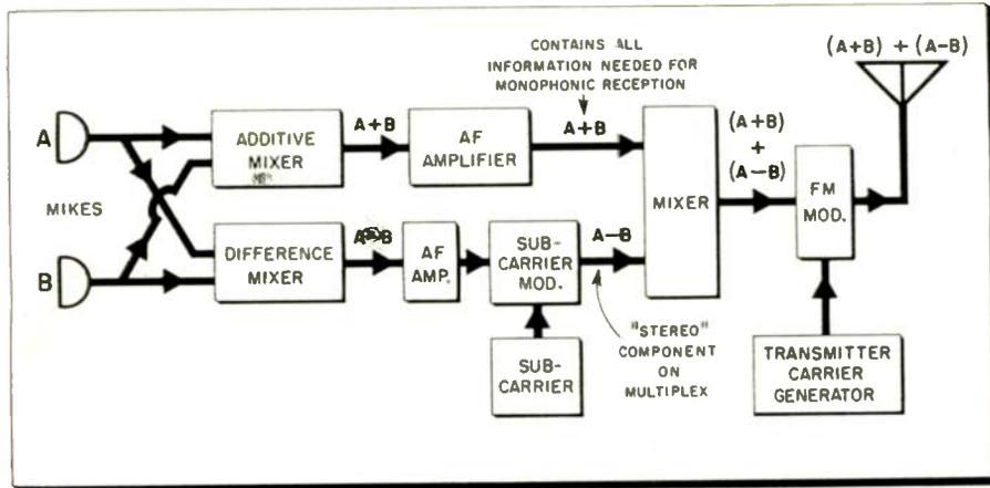
Fig. 1—The sum and difference technique supplies all the information needed for monophonic listening to the main carrier. The sum signals modulate the main carrier, while the difference signals, with one signal reversed in phase, is impressed on the subcarrier.
