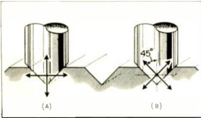
Fig. 1—An early proposed single groove stereo system, shown in A, had a vertical and horizontal axis. The 45/45 Westrex, in B, was chosen by the RIAA as the standard stereo disc system. It maintains the same relative position between the two axes in A, but both are rotated 45°.
