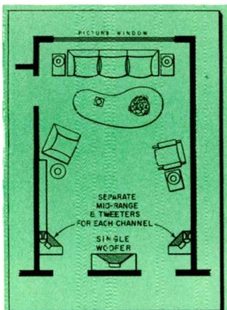
A very large room using widely spaced speakers may require a third speaker to avoid a "hole in the middle" effect.
