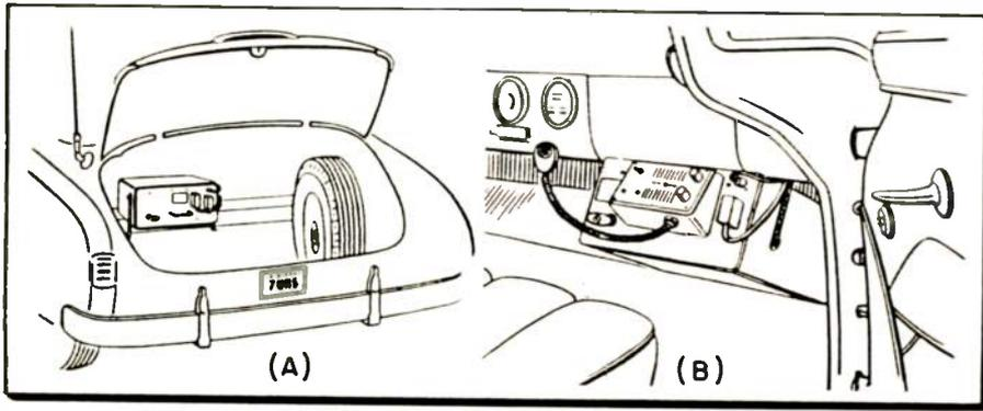
Fig. 2 (A)—Trunk installation of two-way mobile system with location of antenna providing short lead to equipment. (B)—Two-way radio mounted under dash board of mobile vehicle.
