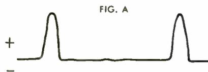
Waveform at flyback pulse at the plate of horizontal-output tube in a typical transformer-coupled circuit.
