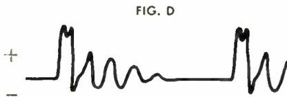
Waveform at the plate of horizontal-output tube in a typical direct-drive circuit with added 5,000-ohm 5-watt resistor. The resistor lowers the "Q" of the transformer to reduce the amplitude of the "ringing" voltage.
