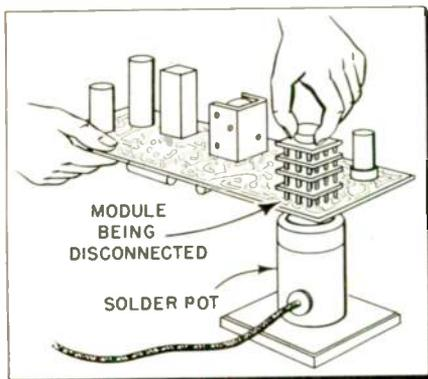
Fig. 10—Soldering pot employed to remove module or any multi-connection component.
