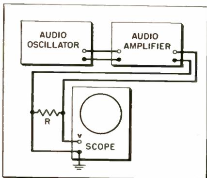
to avoid ground loops and other spurious effects. Oscillator impedance is usually of a low order and can be plugged into a tuner jack, available on most amplifier control units. It is important to match the amplifier's output impedance with a resistor load having the proper ohmage and wattage in order to replace the speaker. When multiple output taps are available, it is desirable, though not imperative, to use the highest impedance tap.
