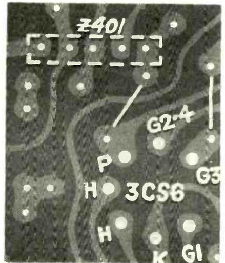
Fig. 5—Easy to check tube pins are identified by Westinghouse "See-Matic" board.
