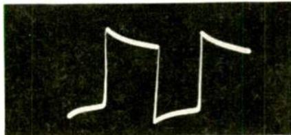
Fig. 10—Tilt in video amplifier causes a shading with a picture smear impression.
