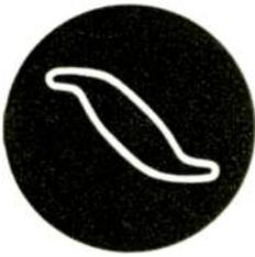
This pattern indicates the presence of phase shift and odd-harmonic generation. Un-symmetrical bending of the ellipse indicates the generation of both even and odd harmonics. Harmonic generation usually ceases when the signal input to the amplifier is reduced.
