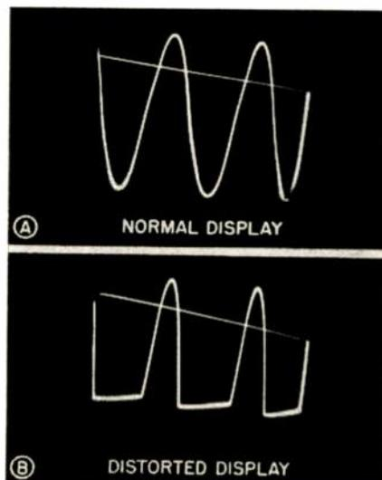
cated by sharp clipping of the output waveform. This fault can be localized to a single stage in the amplifier by injecting the audio-oscillator signal into successive grids through a 0.25  $\mu$ f isolating capacitor. However, when an excessive input signal is applied, any amplifier can be driven into overload. Clipping seen on overload should be symmetrical, occurring simultaneously on both positive and negative peaks.
