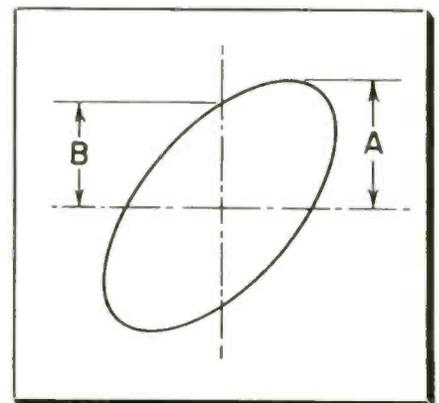
Fig. 7—Phase angle is measured by counting squares on scope graticule to obtain the ratio B/A. Sine of angle is equal to B/A.
