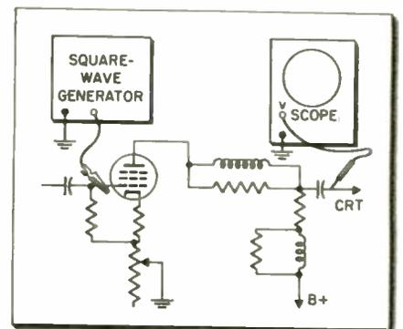
Fig. 2—Simple square-wave generator and scope set-up for identifying TV ringing.
