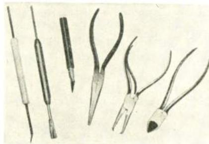
Fig. 8—Assortment of helpful tools aids in making proper printed circuit repairs.
