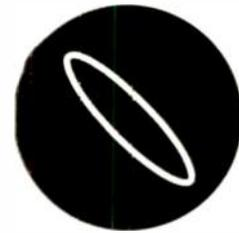
The presence of even-harmonic distortion and phase shift is indicated here. The harmonic distortion is usually a result of overload in one or more stages, and the phase shift is caused by reactive elements in the signal path. At low frequencies, coupling, decoupling and by-pass capacitors whose values are too small usually cause the phase shift. At high frequencies it is generally a result of stray shunt-capacitances across high-value load resistors.
