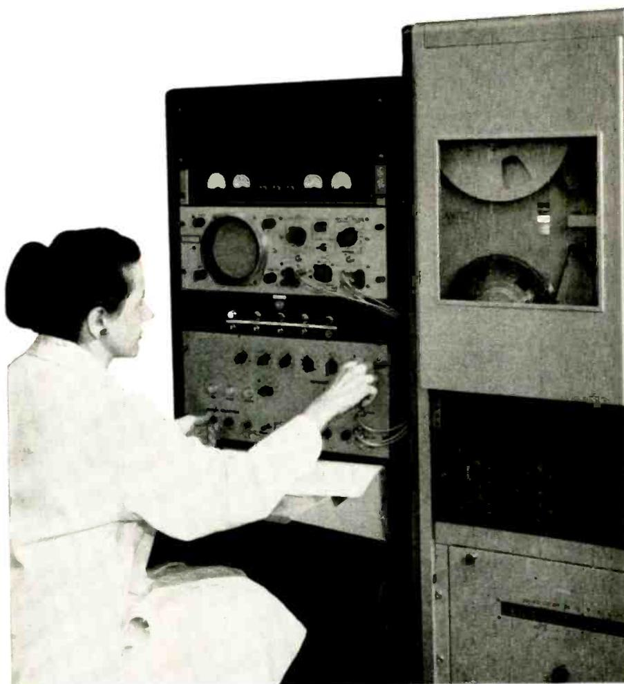
Fig. 1—Aiding in a medical diagnosis of heart disease, the analog-digital converter changes heartbeat data to a form suitable for use in a high-speed computer. Part of the computer equipment is shown with a medical technician at monitor and control position.
