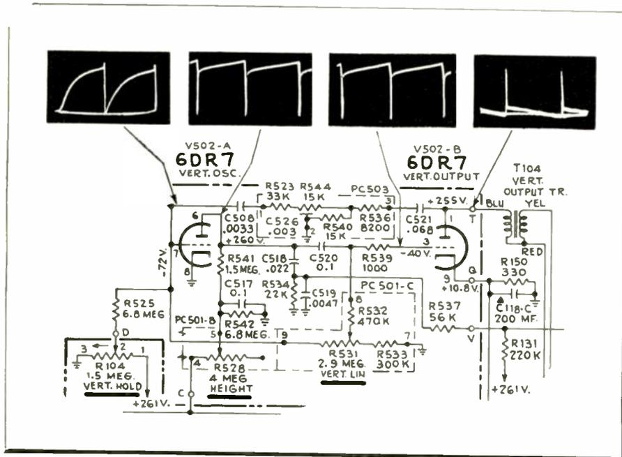
Fig. 1—Schematic of an RCA KCS-128A vertical multivibrator and sweep output circuit.
