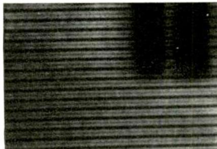
Fig. 6—"Soft" indefinite outlines of two dark areas indicates corner rounding fault.
