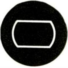
Here, the 90° phase shift is accompanied by odd-harmonic distortion. A double-clipped circle in which the clipping is unsymmetrical on top and bottom indicates a 90° phase shift with both even and odd harmonics.
