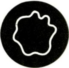
When the circle is not round and displays irregularities, the signal source is not a pure sine wave. The desired phase shift between the signals to the vertical and horizontal amplifiers of the scope can easily be obtained by inserting a variable or suitable value capacitance in series with the lead to the vertical amplifier.
