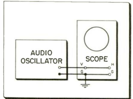
Fig. 5—Set-up with oscillator to check frequency response of the scope amplifiers.
