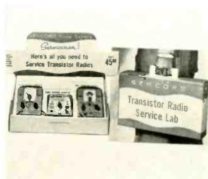
PS103 power supply furnishes power to radios during repair and the HG104 1000 cycle generator is for signal tracing and other purposes. \$45.85 net. Service Instruments Corp., 121 Official Road, Addison, Ill. (ELECTRONIC TECHNICIAN 11-19)
