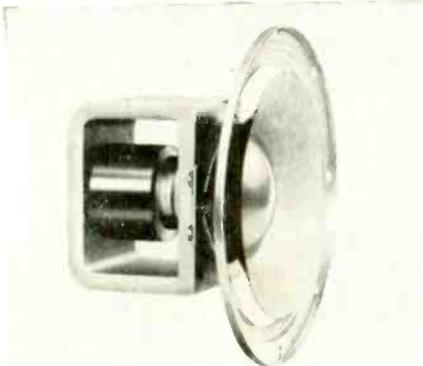
to eliminate the need for an expensive crossover network. The tweeter is rated at 14 watts and has an 8 ohm voice coil. Magnet weight is .45 lb. Altec Lansing Corp., 1515 S. Manchester Ave., Anaheim, Calif. (ELECTRONIC TECHNICIAN 11-23)
