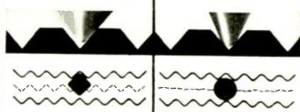
It's here! The new Pyramid Point Diamond — the only needle shaped to simulate the original recording stylus. This exclusive new pyramid shape reduces distortions as much as 85%! Now, for the first time, the full pure tones of all the original recorded sound — stereo and monophonic — are faithfully reproduced. And the greater surface contact area between needle and record prolongs your needle and record life.
