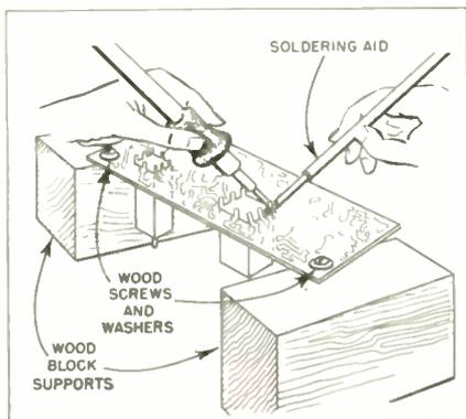
of various components while soldering.
