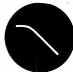
This pattern indicates that the input signal is overdriving the amplifier into both plate and grid-current cut-off—or, that successive stages are being overdriven in one or the other direction. Odd harmonics are indicated when the bending is the same at both ends of the oblique line. Both odd and even harmonics are present when the bends at each end of the line are different.
