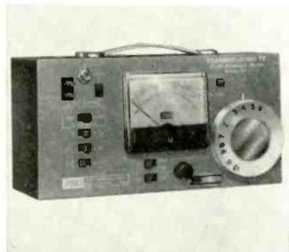
pounds, and has ranges from 100 to 2,000,000 μv. The instrument is reported to respond only to the sync signal of the channel being observed and is immune to noise. Jerrold Electronics Corp., 15th and Lehigh Ave., Philadelphia 32, Pa. (ELECTRONIC TECHNICIAN 11-36)
