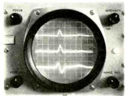
Fig. 2—A scope display of 3 simultaneous signals of the patient's heartbeat is monitored when converting to digital form.
