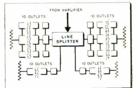
Fig. 2—Typical 40 set distribution system for use in motel or similar applications.
