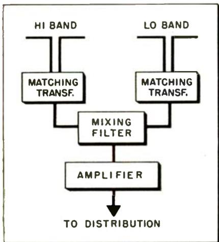
Fig. 1—Signals from high and low band VHF antennas are fed through matching network, combining filter, and then to amplifier.
