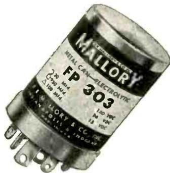
**FP Electrolytics**—The Mallory FP—the original 85°C capacitor—now has improved shock-resistant construction and leakproof seal. Its etched cathode construction—standard in all FP’s—assures hum-free performance.
