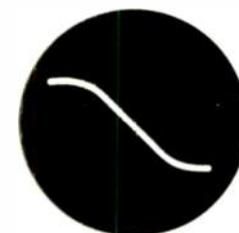
This display indicates some phase shift. Make certain, though, that it isn't being caused by distortion in the scope amplifiers. Although phase shift is not usually detrimental in an audio amplifier unless a negative feedback loop is utilized. In this case phase shift may produce some positive as well as negative feedback, causing distortion of the amplified signal.
