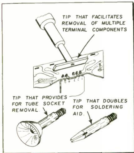
Fig. 7—Special soldering iron tips speed replacement of printed circuit components.
