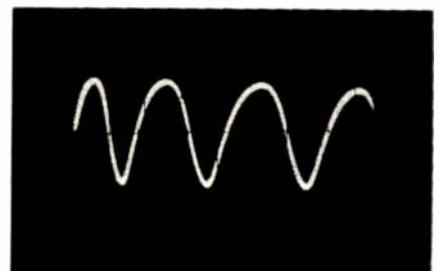
minals of the scope, and the output waveform from the audio amplifier is applied to the vertical-input terminals of the scope.
