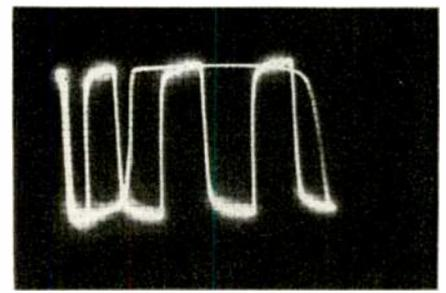
Fig. 7—Cause of "soft" edges is revealed by rounded edges of square waves on scope.
