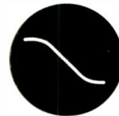
This display indicates some phase shift. Make certain, though, that it isn't being caused by distortion in the scope amplifiers. Although phase shift is not usually detrimental in an audio amplifier unless a negative feedback loop is utilized. In this case phase shift may produce some positive as well as negative feedback, causing distortion of the amplified signal.
