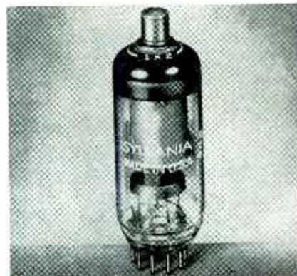
ating from a plate supply of 250 volts or less in which tube plate voltage is supplied partly by the circuit and partly by the low-voltage DC receiver supply. One 6AU5GT, in a suitable circuit, will fully deflect 10BP4, 12LP4, or other picture tubes having up to 60° deflection and with anode voltages up to 12 kilovolts.
