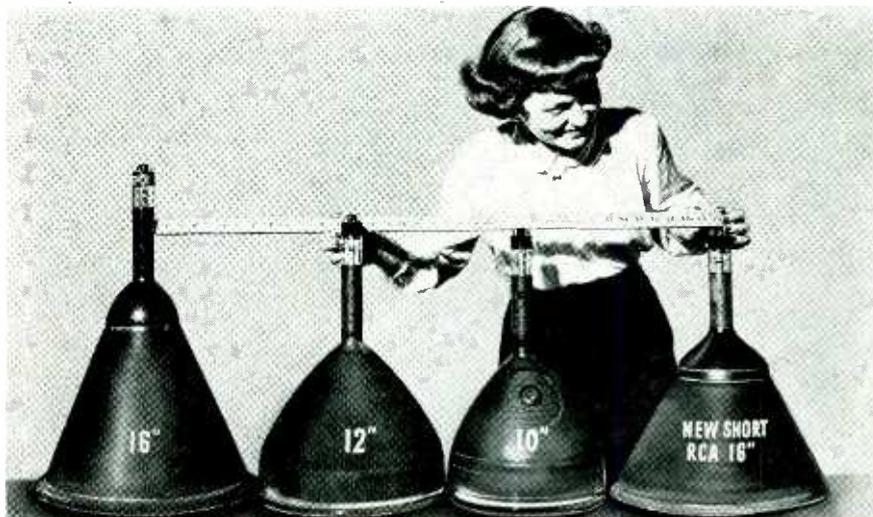
As shown above, the new 16GP4 16-inch metal kinescope is 5 $\frac{3}{8}$  inches shorter than the previous 16-inch tube (16AP4) and is actually shorter than 10- and 12-inch tubes. Shortened length was made possible by the use of 70 degree deflection. The RCA "Filterglass" face plate provides improved contrast.
