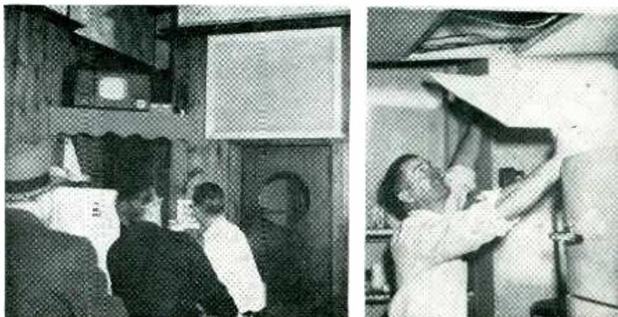
Fig. 3—(left) Large screen built into the wall over the kitchen door in the Anchor Club, Derby, Conn. The "converted" direct-view set is at the left. The projection unit is in a "tunnel" in the kitchen, 70 in. behind the screen. At right, Steve Kabilis is removing the panel which gives access to the projection unit.
