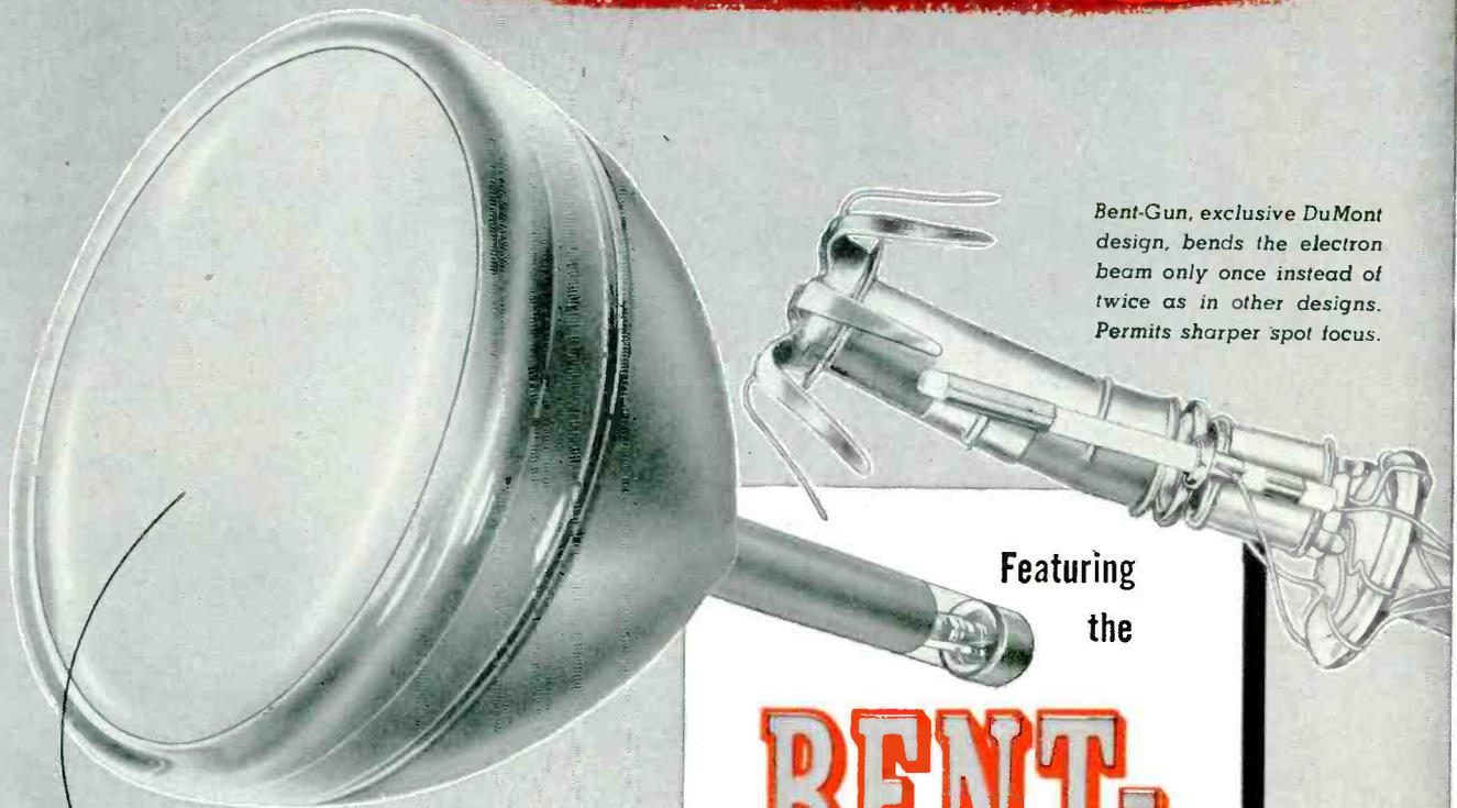
*Bent-Gun, exclusive DuMont design, bends the electron beam only once instead of twice as in other designs. Permits sharper spot focus.*
