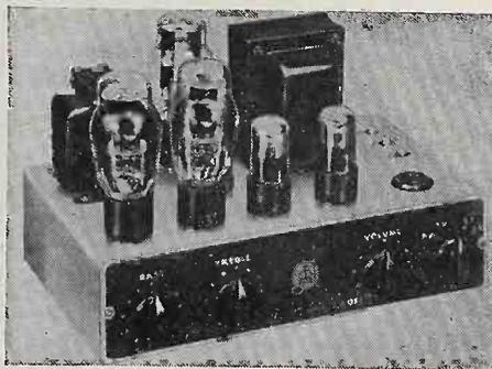
channels, and voice coil and line impedances on a selector switch. 5 tubes, including 2-6L6's in push-pull with stabilized degenerative feedback, provide ample reserve power. Minnesota Electronics Corp., St. Paul 1, Minn.—RADIO & TELEVISION RETAILING.
