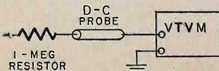
sources of the trouble are the same as those cited for a partially-operative oscillator. The grid-leak voltage, incidentally, will be below normal when the condition just described exists.
