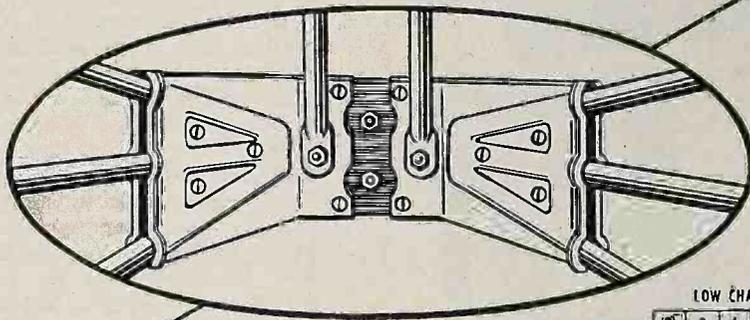
The new apex design used in the Taco Tri-X eliminates the inherent weak point of X type antennas. Heavy aluminum fans, ribbed for extra strength, are bell-mouthed on ends of grooves thus leaving no sharp edges in contact with element rods. Special Taco noise-snubber eliminates bothersome wind-whistle effect. Jiffy-Rig construction provides the fastest, most practical assembly.
