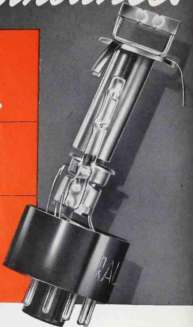
Rauland is happy to announce its newest advancement in Electron Gun design—the fifth Rauland development in a year to benefit both set makers and service men. Effective at once, Rauland is incorporating in all its picture tubes a new "Tilted Offset" Electron Gun which requires only a single ion trap magnet (although a double magnet can be used)—and bends the electron beam only once—and gives the sharpest possible beam focus.
