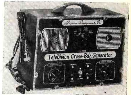
use of a station signal off the air. The generator is connected to the set at the antenna terminals and may be tuned in by using the regular channel selector. Sold through jobbers for \$39.95 by Superior Inst. Co., 227 Fulton St., N. Y. 7.—RADIO & TELEVISION RETAILING.
