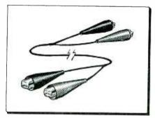
several minutes every day always having two or three double patch cords around. These cords require four small battery clamps, four rubber or plastic clamp covers (two black and two red), and about five
