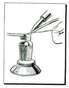
letting the lead (or solder) solidify while the end of the battery clamp is held in it. This "third hand" is a good item to carry along in the tool kit for those outside calls, too. M. Quisenberry, Bucks Radio & Appliance Co., Lexington, Va.
