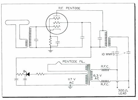
Above, typical circuit showing how transmission line is used to supply power to booster on top of antenna. Below, power unit at TV set supplies 6.3 volts to booster, and takes off TV signal for tuner imput.
