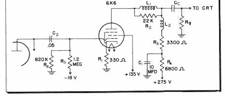
Fig. 4. Video amplifier circuit showing low frequency and high frequency compensation details.
