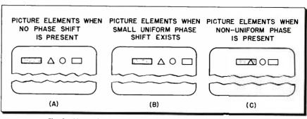
Fig. 2. Above picture screens represent various conditions of phase shift.
