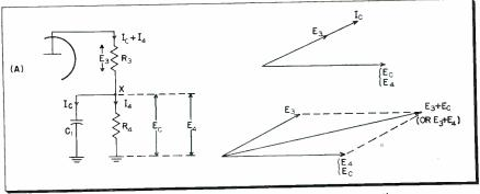
Fig. 5. Video amplifier showing low frequency compensation.
