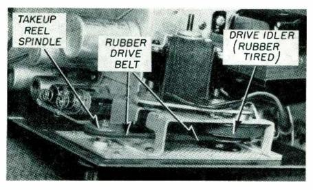
wheel is driven by an electric motor, either coupled to its shaft through a pulley-and-idler combination, or by means of a rubber belt.
