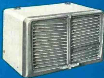
MODEL ACD-33. For rooms up to 230 sq. ft.,\* at the rate of 140 cu. ft. per minute. ½-horsepower hermetically sealed compressor. Controls for ventilation, circulation and cooling. 13½" high, 23½" wide, 27" deep.
