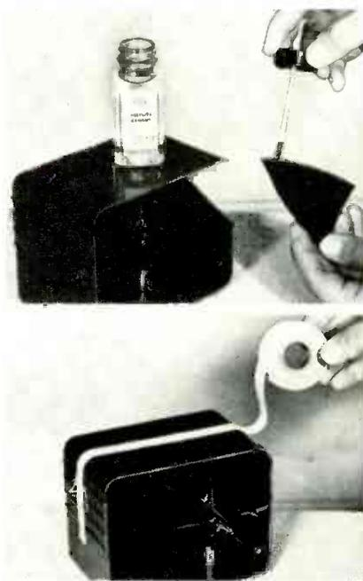
Cement Co.) and then it was firmly placed in original position. Adhesive tape was then used around the entire case to hold the broken piece in place until the cement had set.—*H. Leeper, 1346 Barrett Ct., NW., Canton 3, Ohio.*
