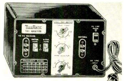
knobs. The wave traps and filters can be used either singly or in any combination, as required. The unit is housed in a compact steel case measuring 5½ by 7-in. Net price to servicemen is \$19.95. Tele-Matic Industries, Inc., 1 Joralemon St., Brooklyn 1, N.Y.—TECHNICIAN.
