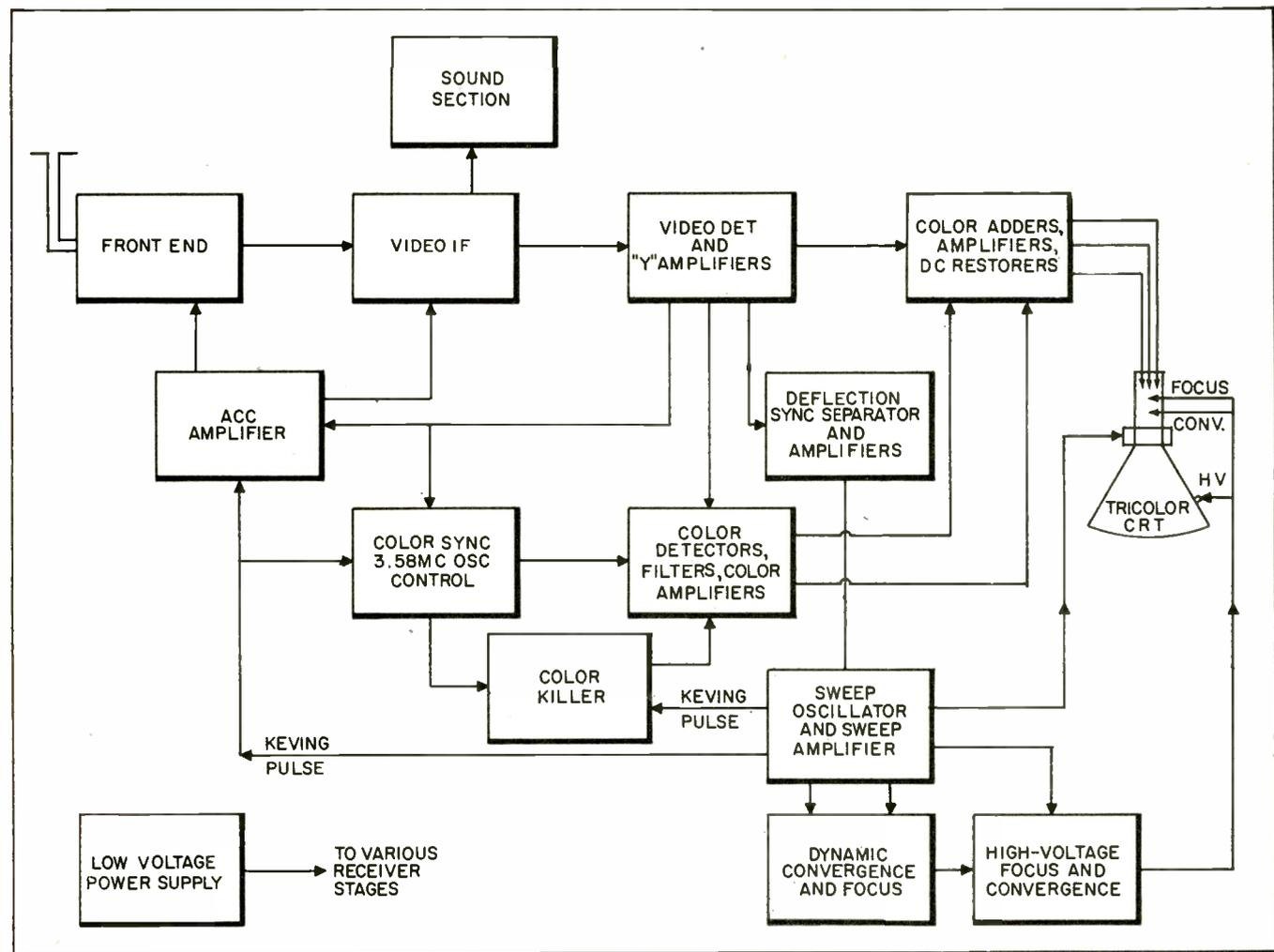
"Y" signal is the luminance information of the color signal—that is, it contains information regarding the brightness of each pictorial unit. This "Y" signal is, incidentally, the only one of the several video signals present in the color transmission that a monochrome set will also respond to, and is equivalent to a monochrome video signal.
