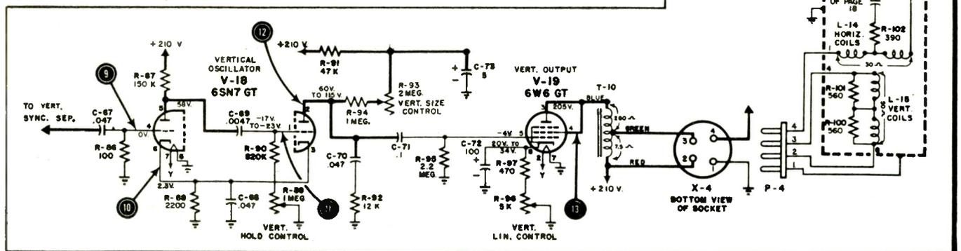
in size from the other, look no further; replace the yoke. (It would seem wise to check components in parallel with yoke windings, before condemning the yoke—Ed.)
