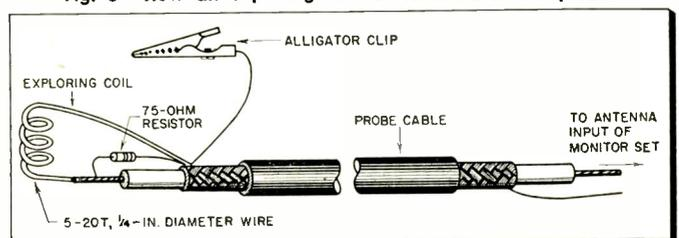
plate of a condenser, the metallic parts of the circuit near it comprise the other plate. Capacitive coupling is thus used to transfer the TVI from the circuit (or several circuits) being tested, to the probe.
