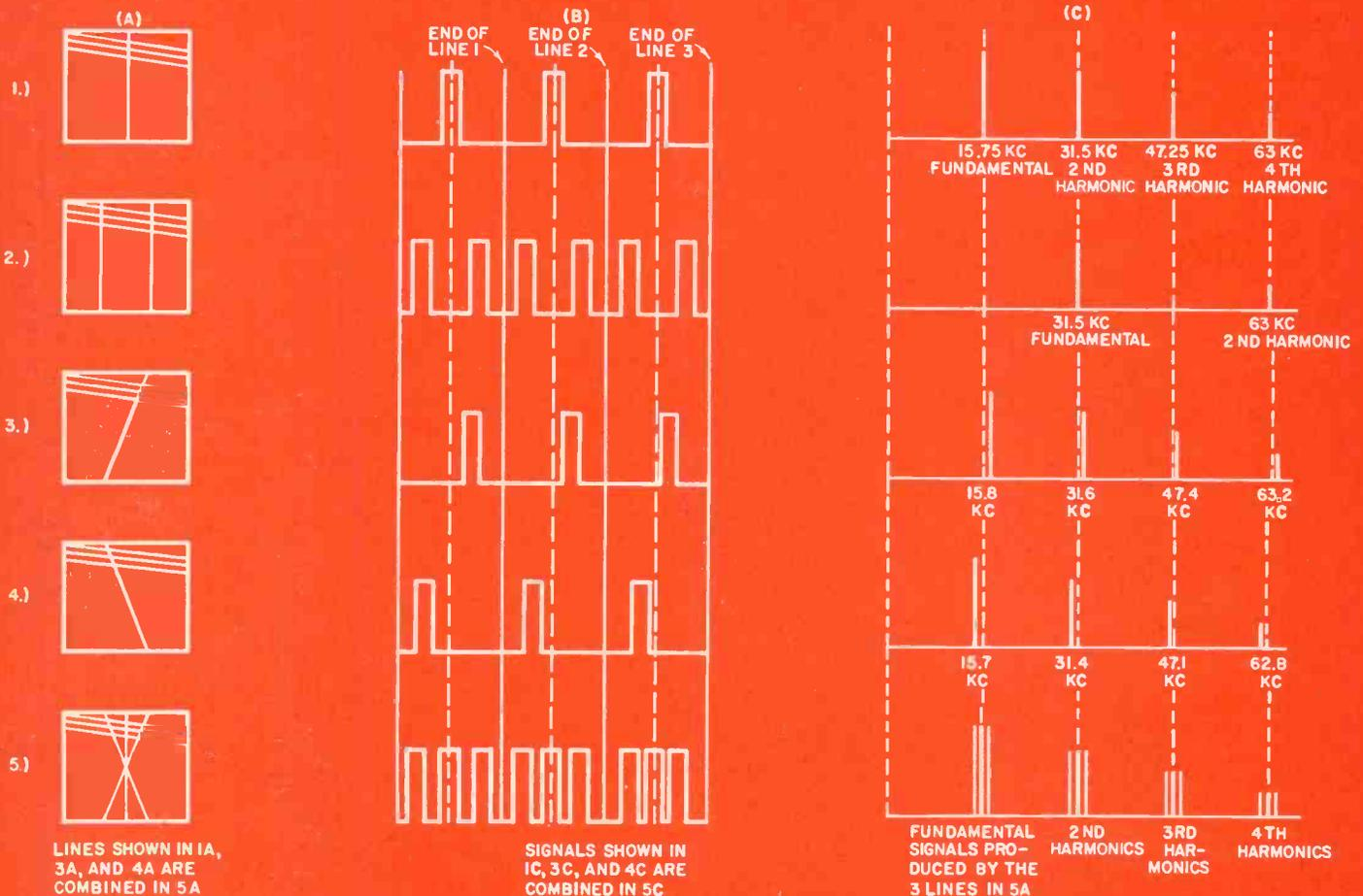
Figs. 1 to 5—Pictures discussed in text are shown in column A (three scanning lines are assumed); video signal waveshapes they produce are drawn beside them in column B (sync signals are omitted); the frequency spectrum produced by the video signals is shown in column C. Note that in all cases illustrated in (C), the video information clusters around line-frequency signals or harmonics of line-frequency signals.
