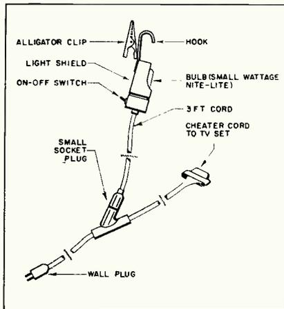
cheater cord is necessary for inspection of the set during operation. I parallel the cheater cord with another AC line, about three feet long, fixing a small light bulb at the other end of the added line (see sketch). On the small light I fasten an alligator clip and a hook, by either of which the bulb can be attached to any safe and convenient part inside the cabinet or on the chassis.—Alvin Diedricksen, New Britain, Conn.
