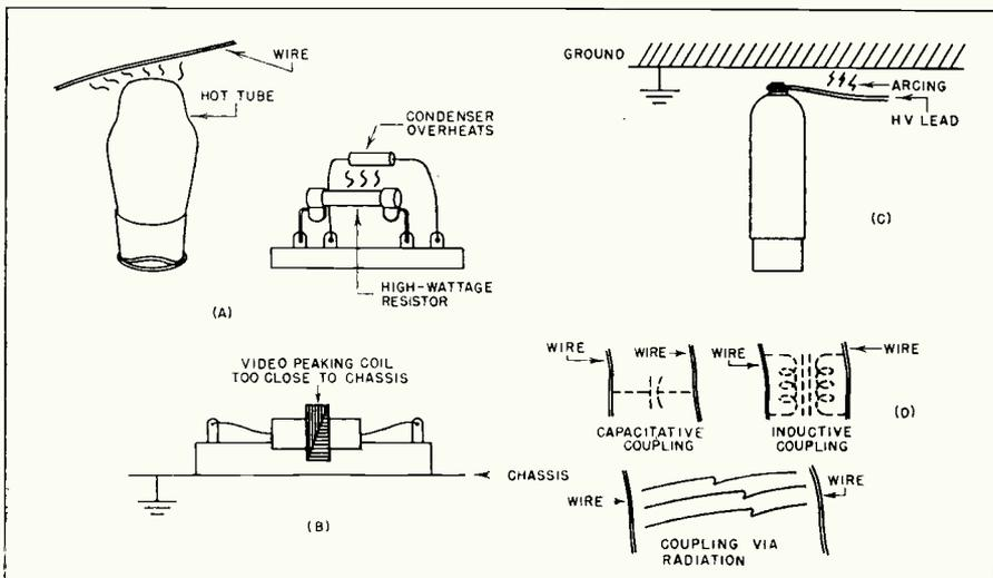
buzz include sync pulse pickup, intercarrier buzz, vertical sawtooth pickup, and mechanical vibration of laminations in a vertical sweep or power transformer. To determine whether the buzz is caused by the vertical circuit, vary the vertical hold control. If a change in the pitch of the sound is now heard, then the buzz is originating in the vertical circuit.
