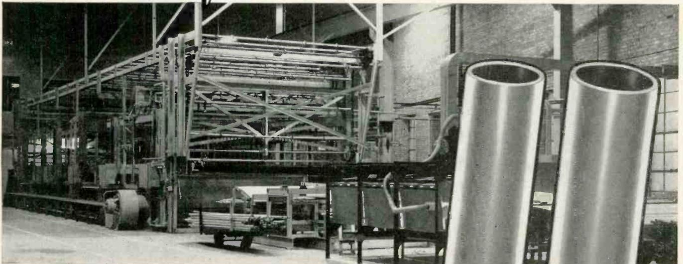
Admiral's huge production brings you these 5 and 10 foot masts at the industry's lowest prices. Finest quality, too . . . made of cold-rolled seamless steel tubing, heavily electrogalvanized. For added rust resistance the inside of each tube is plastic coated throughout its entire length. Both 5 and 10 foot masts are available with one end flared to take extensions . . . eliminates the need for separate mast couplers.
