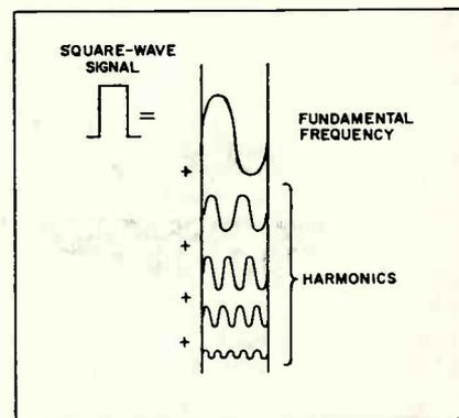
Fig. 6—If a square wave signal is analyzed, it is found to consist of fundamental and harmonic frequencies. The higher the harmonic, the smaller its amplitude.
