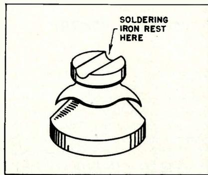
insulator of the type used on telephone poles (see sketch). The depression in the top serves to hold the iron in a natural cradle, and the flanges serve to make an efficient radiator. The porcelain types seem to work the best, although a glass unit may be used. The insulators can be obtained anywhere the telephone company is replacing chipped insulators, or they may be purchased at any electrical wholesale store for a few cents each.—John A. Cooley, Washington, D.C.
