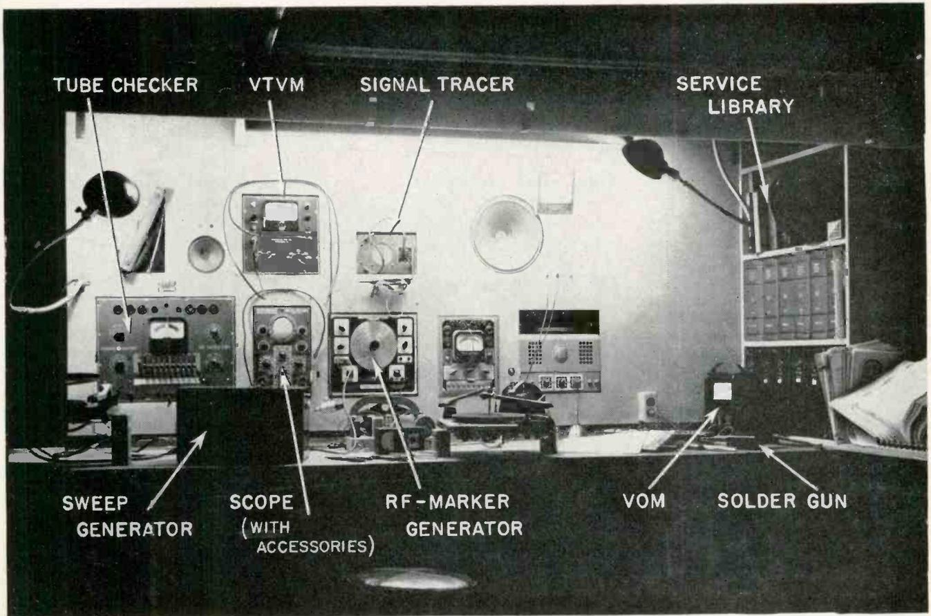
One version of a service bench. Basic equipment and other shop gear discussed in the article are illustrated. Added requirements may vary. In the set-up shown, for example, a second tube checker, test speakers, and a test record player-amplifier combination have been incorporated.
