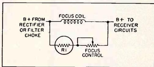
Typical Focus Coil Circuit
