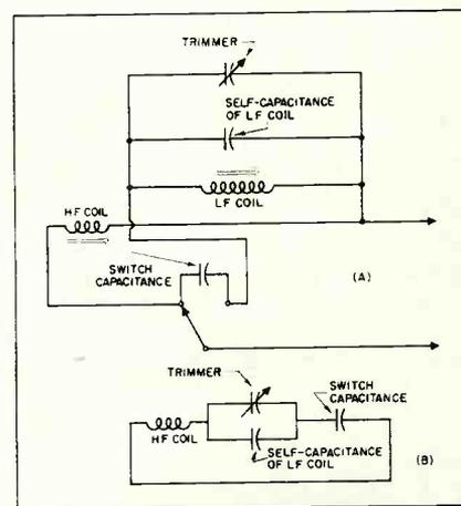
Fig. 8A—Schematic of section of tuner circuit. B—Parasitic circuit of tuner shown in (A).
