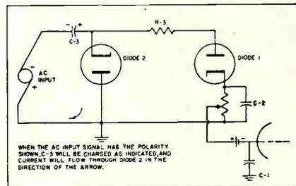
Fig. 4—Audible alarm input circuit, redrawn and simplified to clarify the circuit action of the condensers and crystals.
