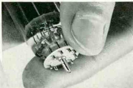
During January and February, Order 20 CBS-Hytron miniature tubes. Your distributor will *give* you this package of 10 new CBS-Hytron Socket Locators. With them, plugging miniatures into hard-to-locate sockets is easy. Socket Locator slips over pins of tube (7-pin or 9-pin). Key of Locator finds socket . . . guides tube into it, quickly. Save time and temper . . . take advantage of this limited offer. See your CBS-Hytron distributor.
