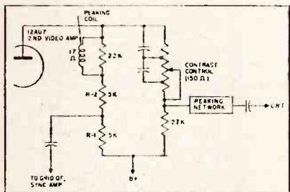
Video amplifier plate circuit in Zenith 24H20. Note parallel networks between plate and B+.
