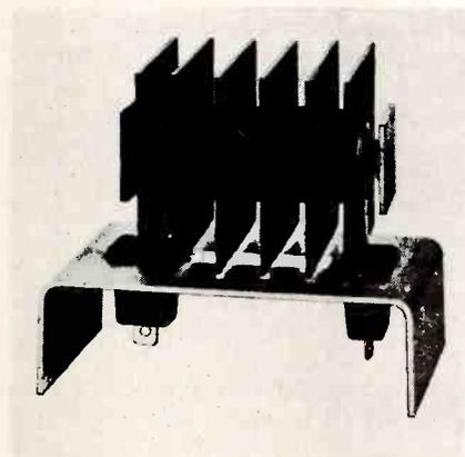
The rectifier lugs are polarized for proper circuit connection and are so designed that vibration or shock will not cause the rectifiers to fall out of the socket. It is possible to mount the plug-in rectifier in a conventional manner and solder to the lugs. Sockets are available from the Cinch Manufacturing Company, Chicago, Ill.—TECHNICIAN
