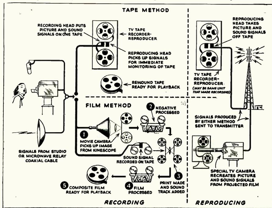
New RCA developments in 3-megacycle magnetic recording, open way to reproduce TV and color-TV pictures from magnetic tape, like sound.
