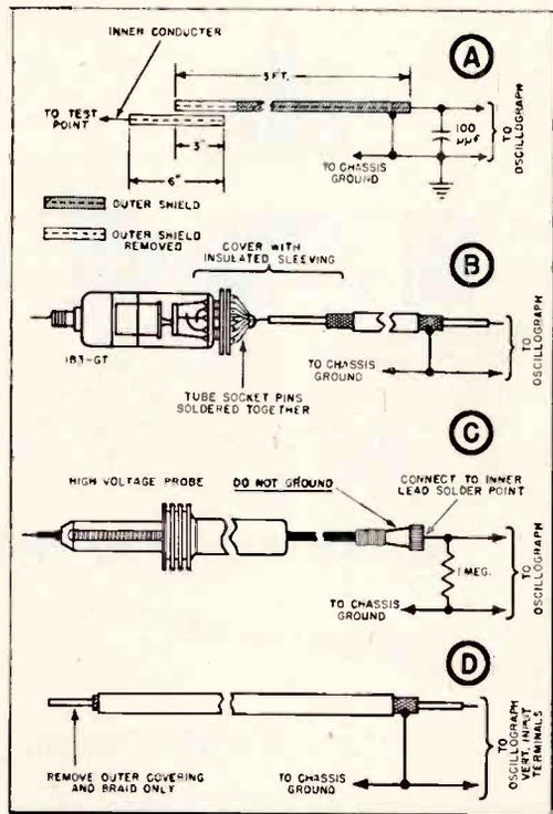
Figure 1. A—Capacitance divider probe to be used with oscillograph when examining waveforms in horizontal output and high-voltage circuits. Stepdown ratio is approximately 100:1. B—Capacitance divider probe which uses a 1X2A rectifier as a high-voltage capacitor. C—Resistance divider probe for use with oscillograph. A regular vtvm high-voltage probe and a 1 meg resistor are employed. D—Gimmick which permits examination of horizontal-sweep waveforms without removing chassis from cabinet.
