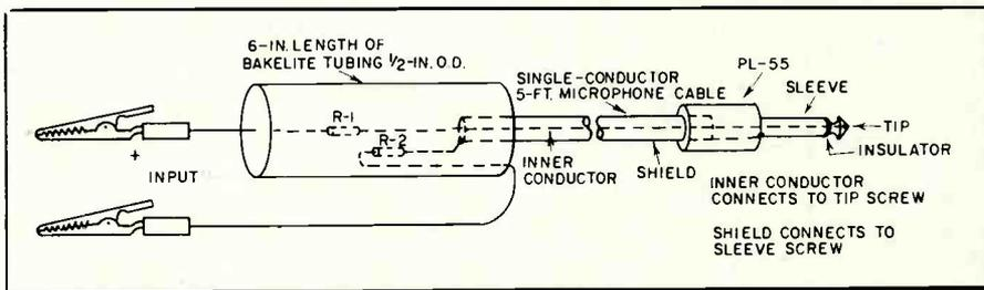
Fig. 2 (Above)—DC probe used with monitor. Fig. 3 (Below)—AC probe used with monitor.
