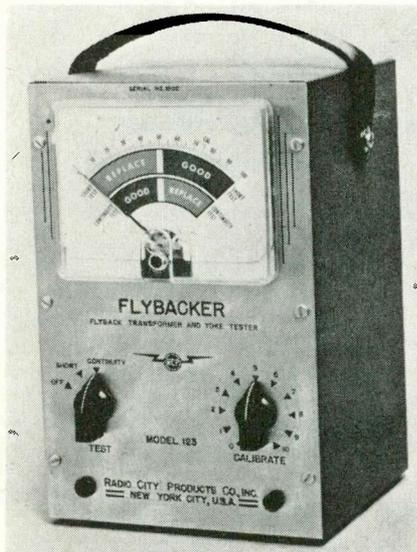
transformers or yokes still connected in the receiver. Radio City Products Co., 152 W. 25th St., N. Y.—TECHNICIAN
