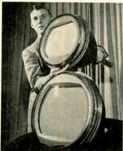
pared with the company's 15-in. tube, which is now in production. Based on the earlier tube, the 19 incorporates some design changes: new gun assembly, improved phosphors, modification of the shadow mask and a wider deflection angle. The latter makes possible an overall length no greater than that of the 15-in. crt.
