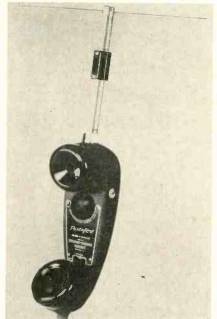
weighs less than 2 pounds. With carrying case and battery, weight is about 5½ pounds. Set to transmit on 465 mc, the Portafone is said to have unusual stability in the face of wide changes in temperature, humidity and operating voltages.
