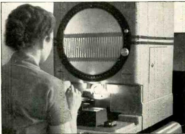
● A General Electric plant employee, using a comparator, checks a greatly magnified tube grid.
