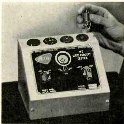
tester uses an electronic eye to reveal control-grid emission, also to indicate high resistance grid-cathode or cathode-heater shorts. Maker recommends it for checking tubes in the audio, i-f, and sync sections, where trial-and-error, wait-and-see substitutions are normally used. List price, \$24.95. Available in kit form as model GCT-2, \$19.95. Seco Mfg. Co., 5015 Penn Ave. S., Minneapolis, Minn.—TECHNICIAN
