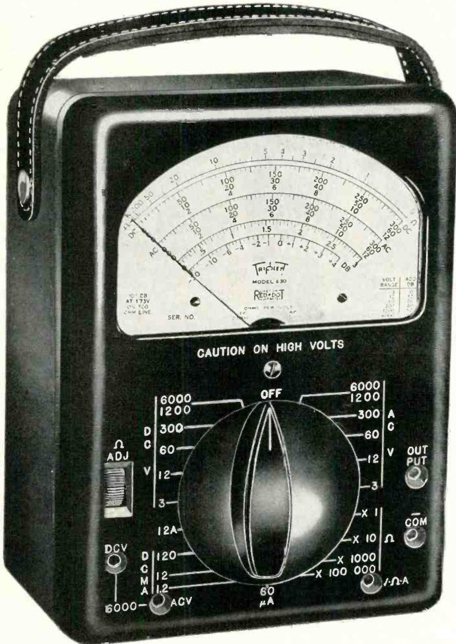
ing to desired circuit thru a single 2½" knob flush with the face panel. The molded switch itself embodies the most advanced engineering practices. Fully enclosed, the silvered contacts are kept permanently clean. Its rugged construction means stronger performance and longer life.
