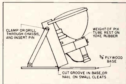
base of the crt does not contact the mounting board.—*F. C. Hoffman, Kewaunee, Wisconsin.*
