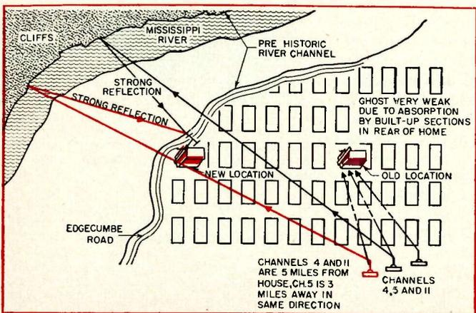
Fig. 3—Sketch indicating why shop antenna worked well only at the site indicated. Lines with arrows represent incoming signals.
