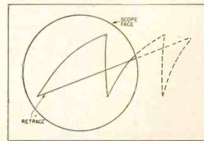
Fig. 4—Display adjusted so that only the left-hand or most linear part of the signal is left on the screen for inspection purposes.
