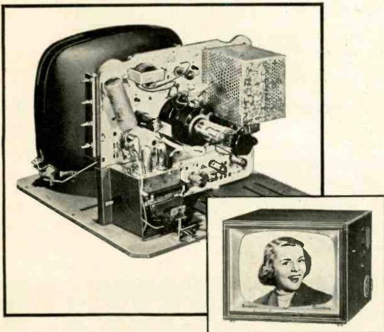
"The Crosley Super-V is a service man's dream; the new vertical plane chassis allows the changing of any tubes in a very few minutes. When service of a more complicated nature is required, the entire cabinet can be removed by loosening 6 screws; this leaves the entire chassis accessible for service. Another wonderful feature is that the picture-tube chassis and bracket are incorporated in one common mounting board along with the points wired on terminal strips for easier circuit tracing."
