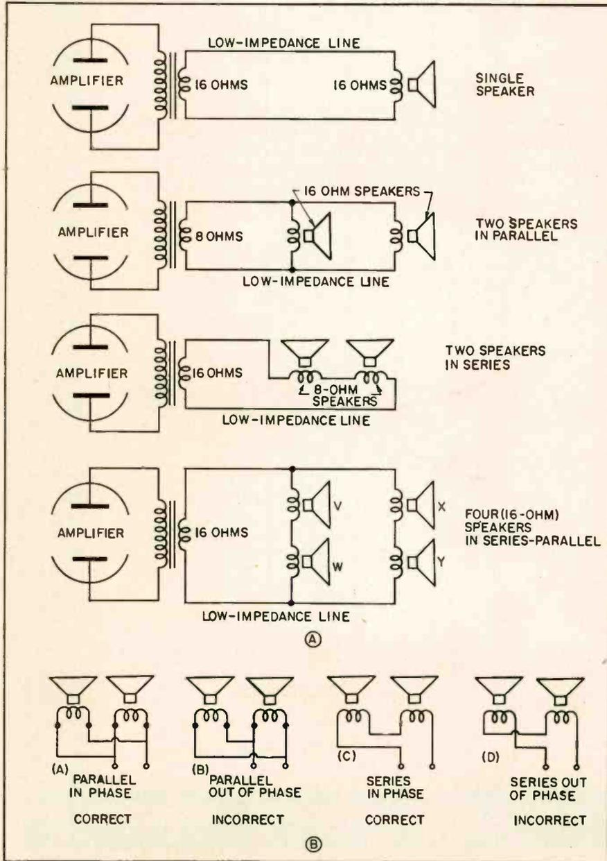
The last sketch shows four speakers in series-parallel. The 32 ohm impedance produced by the series connection of speakers V and W, is in parallel with the 32-ohm impedance of speakers X and Y in series. The overall load therefore equals 16 ohms, and properly matches the 16-ohm secondary of the output transformer.
