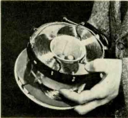
the planar mask type, the monconvergence shadow-mask type, and the type in which the color phosphors are applied directly to the curved face. The complete yoke with plastic case removed is being held by Edgar Messing, General Instrument exec.
