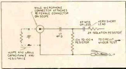
Fig. 6—Schematic of low-capacitance probe.
