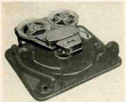
ers, is available in 2 models. Frequency response for model 375 (3¾ in. per sec.) goes from 50 to 6500 cps; response for model 750 (7½ ips) ranges from 50 to 10,000 cps. Either unit accommodates 5-in. reels with dual-track tapes and feeds its output directly into equipment designed for standard magnetic phono cartridges. Where a magnetic input is not part of the equipment, the model 2246 pre-amp may be used. The units are only 10 in. square, sell for \$29.95 each.
