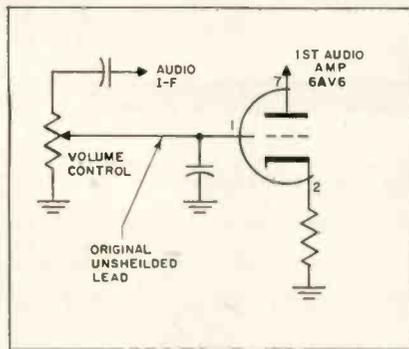
time checking the sync or other circuits; the trouble is in the audio. The trouble spot is an unshielded lead going from the tap on the volume control to the grid (pin 1) of the 1st audio amplifier, 6AV6. We replaced this lead with a length of coaxial cable, which was grounded at both ends of the shield; however, ordinary shielded audio wire can be used.—Paul Leichter, Philadelphia, Penna.
