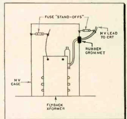
fuses can be used as anchors. Since the fuse is blown, the glass envelope provides effective high voltage insulation. As with cellulose tape, the applications for these fuse "stand-offs" are only limited by the technician's ingenuity. The pigtailed are used for tying purposes. Some possibilities are illustrated. B. O. Riis, Little River, Miami, Fla.
