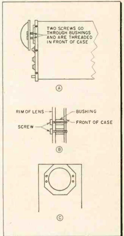
Fig. 3A—Side view of enlarger mounting. B—Mounting detail. C—Front view of unit.
