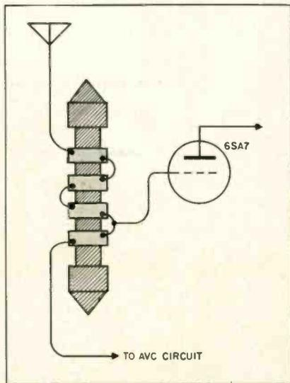
The grid of the 6SA7 tube was connected between the first and second "pie," (counting from bottom). The lead at the top end of the uppermost "pie" went to the antenna. The remaining (bottom) lead was connected to the AVC circuit, as shown. After completion of the repair, the set was given a thorough test. It performed perfectly.
