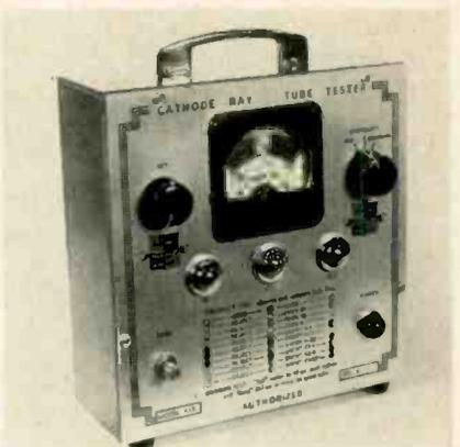
emission and indication of gaseous tubes. Tests can be made with crt in carton, TV set, cabinet or on the bench. Weight: 5 1/2 lbs. Authorized Manufacturers Service Co., 919 Wyckoff Avenue, Brooklyn, New York—TECHNICIAN
