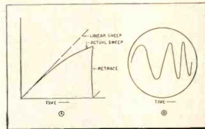
Fig. 3A—Non-linear sweep. B—Effect of non-linearity shown in (A) on a sine-wave signal.
