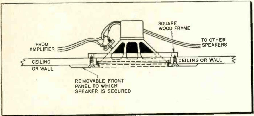
Fig. 3—Method of connecting ceiling or wall speakers to permit access to speakers and cables.
