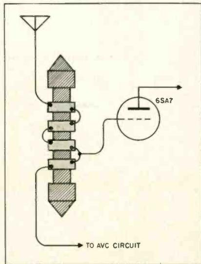
The grid of the 6SA7 tube was connected between the first and second "pie," (counting from bottom). The lead at the top end of the uppermost "pie" went to the antenna. The remaining (bottom) lead was connected to the AVC circuit, as shown. After completion of the repair, the set was given a thorough test. It performed perfectly.
