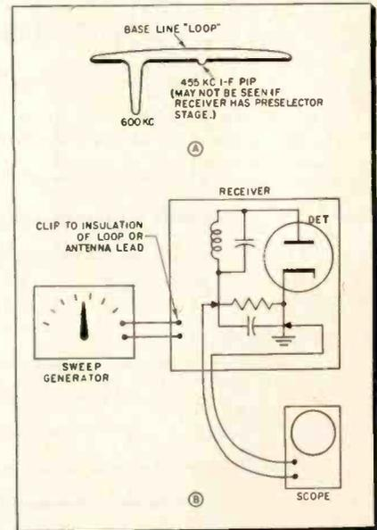
Fig. 2A—Connection of sweep generator and oscilloscope for oscillator alignment at the low-frequency end of the band. B—Response obtained on scope. To minimize “looping” of the base line, reverse line plug to the sweep generator, scope or the radio.
