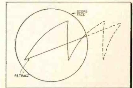
Fig. 4—Display adjusted so that only the left-hand or most linear part of the signal is left on the screen for inspection purposes.
