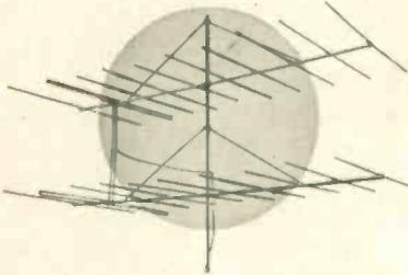
**PHILCO TWO-BAY VHF LOW BAND YAGI ANTENNA:** 10 elements . . . all-aluminum . . . factory pre-assembled. Top performance on channels 2 through 6 . . . 13 db to 15 db gain on various channels. Single bay Part No. 45-3112-2 through 6. Stacked version uses stack-harness Part No. 45-3267.
