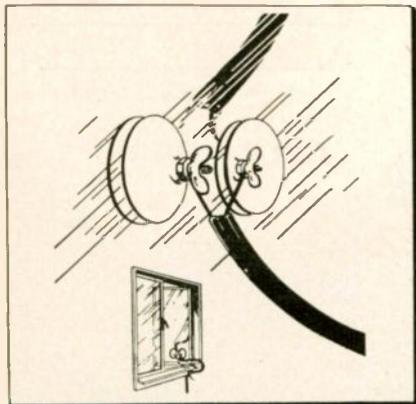
any window in a few minutes, is effective for VHF and UHF. Weatherproof capacitor discs attach to the window pane; windows can be
