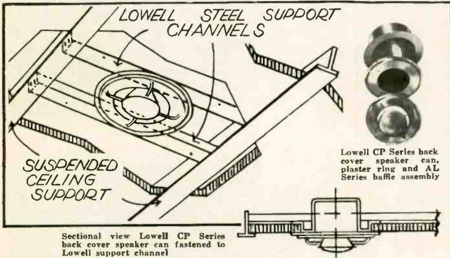
Sectional view Lowell CP Series back cover speaker can fastened to Lowell support channel
