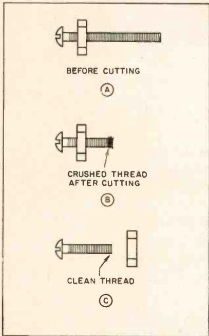
vent this, thread a nut of the right size on the screw *before* cutting, as shown in A. After cutting, when the starting thread has been crushed by the hacksaw blade (see B), the nut is simply threaded off the screw. In coming off, the nut will clean the thread, as shown in C.—M. G. Goldberg, St. Paul, Minn.
