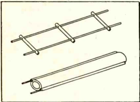
450-ohm open-wire vs 300-ohm tubular line. courtesy Du Mont
