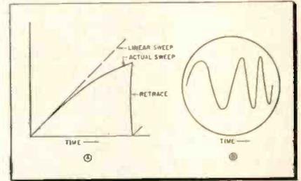
Fig. 3A—Non-linear sweep. B—Effect of non-linearity shown in (A) on a sine-wave signal.
