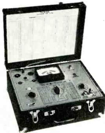
testing of tubes by non-technical clerical help when the checker is used on the counter. Only 5 sockets are used. Tube types are printed on 12-position selector switch; only 2 other controls must be adjusted. Tests for emission, interelectrode shorts or leakage, and gas. Price, \$99.50. Television Engineers, Inc., 311 East 79th Street, Chicago 19, Ill.—TECHNICIAN
