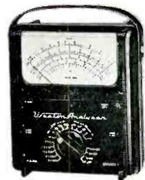
—highly versatile, accurate and rugged volt-ohm-milliammeter with a combination of functional ranges which provide a wide range of test measurement applications in the electronic field. D-c sensitivity of 20,000 ohms/volt, a-c sensitivity 1000 ohms/volt. Accuracy 2% d-c, 3% a-c. Range and functional switching greatly simplified by use of a single dial for all ranges and functions.
