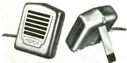
Ceramic model M101 and crystal model M102 hand microphones are compact units housed in plastic cases, designed for prolonged stability. Output of the crystal M102 is -46 db and that of the ceramic M101 is -53 db. Frequency range of the former is 30 to 10,000 cps with flat response, while range of the M101 is 30 to 8000, with slightly rising characteristics in the high range. The M102 lists at \$7.25; the M101 at \$7.00. Astatic Corp., Conneaut, Ohio.—TECHNICIAN
