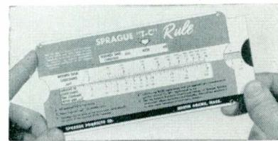
Use this handy pocket-size Sprague Temperature Coefficient Rule to find quickly the values of stock N750 and NPO type ceramic capacitors to connect in parallel to equal a capacitor of desired intermediate temperature coefficient of the required capacitance.
