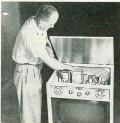
1955 line of Satchell Carlson receivers should make a big hit with TV techs. Chassis—all plug-in units—is mounted under hinged lid. Units are individually removed for servicing. Tube replacements are made from standing position.
