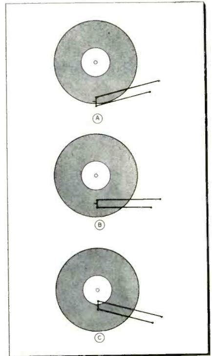
Fig. 2—How arm tracks across surface of disc.
