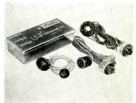
handy extension for many late type TV receivers; CRT Socket Extension, model SE-3—6-wire, for use with all picture tubes. The transparent C-thru case is silk-screened with extension "data" for instant selectivity. Vidaire Electronics Mfg. Corp., 576 W. Merrick Rd., Lynbrook, N. Y.—TECHNICIAN (Ask for No. 4-94)
