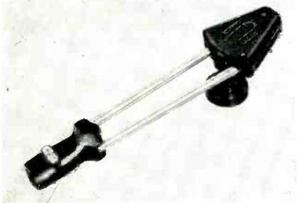
there are four pivot points instead of one. The action of the arms while they swing an arc across the disc automatically corrects the position of the pickup. Fig. 2 shows how such a device would operate. At the beginning of the record side (part A), the head is swung around to counter the angle of the arm, and tracking remains tangential. This relationship is maintained throughout the play (Fig. 2B, C).
