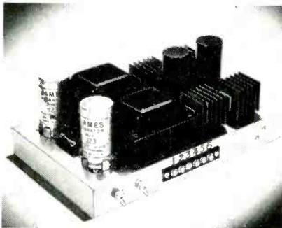
low voltage transmitter and a reserve voltage tap, and has an incorporated receiver muting relay. Supply will operate on either 6 or 12 v. by minor tap changes. The same standard heavy duty 4 prong vibrators are used for either input voltage. Completely wired and tested, \$49.95; in kit form, \$39.95. James Vibrapower Co., 4036 N. Rockwell St., Chicago 18, Illinois.—TECHNICIAN (Ask for No. 4-23)
