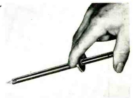
Fig. 2—Thumb pressure exposes the hook tip.
