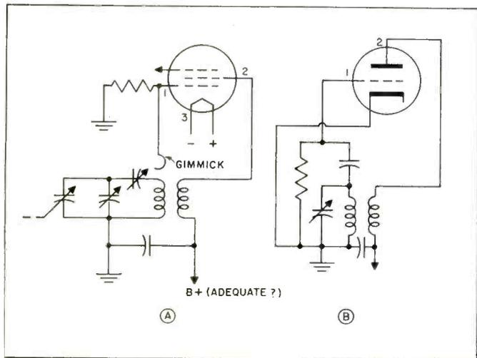
Fig. 4—The grid bias for the oscillator may also be employed as the minimum bias for a stage that is also controlled by avc.
