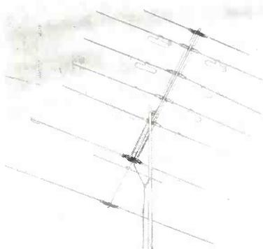
low band channels. All elements are in the same plane, providing extremely rigid construction; no boom braces are required on the 1½-in. crossarm. The antenna was designed for fringe area reception. Elements are completely factory assembled by means of a spring-loaded quick rig design. Technical Appliance Corp., Sherburn, N. Y.—TECHNICIAN (Ask for No. 4-20)
