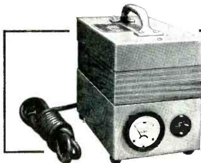
Regardless of line voltage supply, the Automatic Voltrol corrects voltage fluctuation over a range from 95 to 130 volts. The voltmeter supplied indicates secondary voltage while unit is in operation. A built-in relay automatically disconnects circuit when set is turned off.
