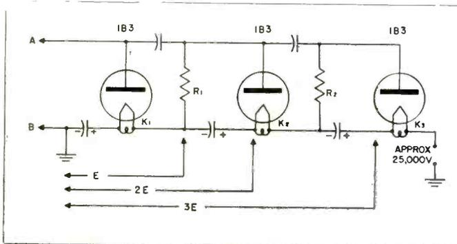
Fig. 5—Novel high-voltage tripler uses r-f tanks for efficiency.
