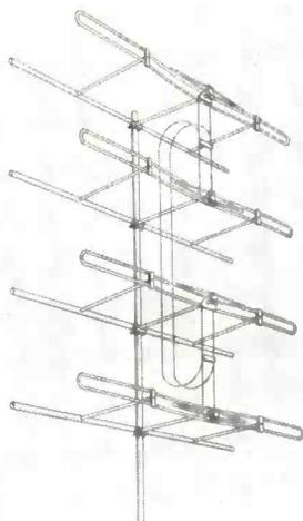
from the station. "Fidelity Phasing" eliminates the necessity of matching harnesses to correct impedance mismatch. The Model F-4 is ideally suited for color and has extremely flat frequency response—less than 1 db. variation in frequency response on any channel. All-aluminum, weather-proof construction. Pre-assembled. The Finney Company, Cleveland, Ohio.—TECHNICIAN (Ask for No. 4-24)
