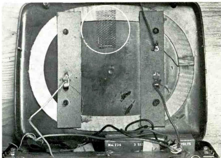
Fig. 2—How a strip of screen is used to tune loop antenna. Metal strips may also be used.
