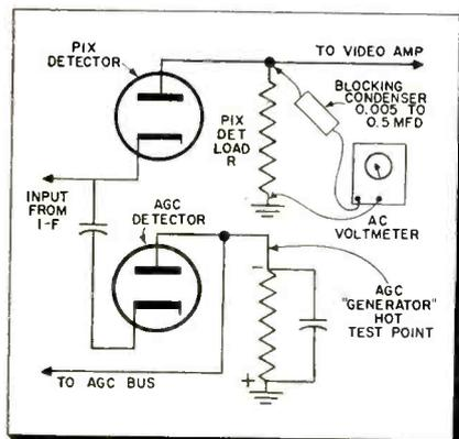
Fig. 2—Set-up for monitoring agc output.
