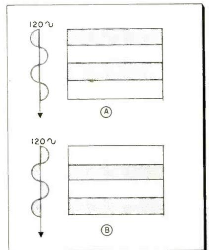
Fig. 3—Two solid bars means 120 cps hum.
