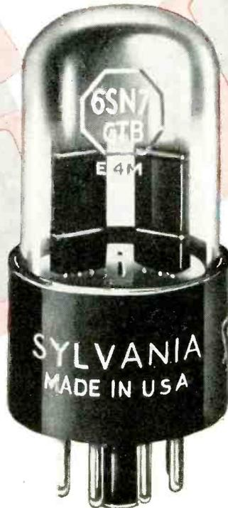
\* In a 15-tube series string, analysis proved that 99.7% of all probable combinations of Sylvania types operated within 2% of the heater-current design center. Sylvania's tight heater-current limit is one of the most important contributions to tube performance for series string operation.
