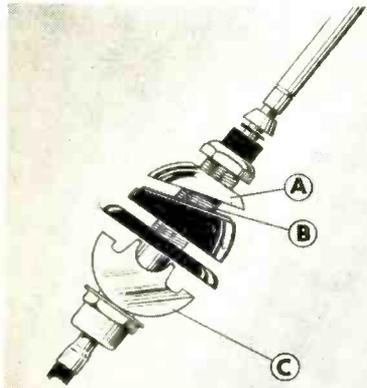
base which permits mounting on any curved surface with a slant of up to 35° from horizontal. Only one hole is required for installation, and the entire job can be done from the outside of the car. All exposed metal parts are heavy brass, triple chrome plated. The "Baseball" antenna is sold completely assembled, with a 56-in. replaceable telescopic whip, and either a 36-in. lead or a 54-in. lead. The Antenna Specialists Company, 12435 Euclid Ave., Cleveland 6, Ohio.—TECHNICIAN (Ask for No. 4-28)
