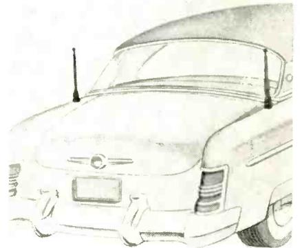
from the ignition system. The two 3-section staffs are 13½ in. high when collapsed, and 27 in. high when extended. They are easily mounted on the rear fenders and are adjustable to 180°. They are available in the swivel type (RD-8 and in RD8B for country and low signal area reception) and in the ball and socket type (RD-9 and RD-9B). Snyder Mfg. Co., 22nd & Ontario Sts., Phila., Pa.—TECHNICIAN (Ask for No. 4-38)
