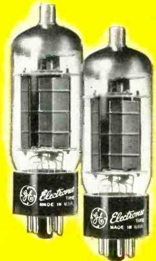
● Prototypes gave arc-over trouble, causing horizontal TV-picture streaking. In the new sweep tubes, brand-new mica design corrects this fault.
