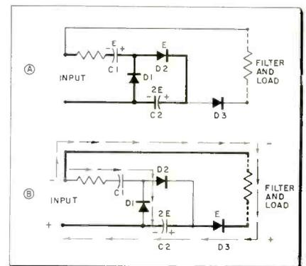
Fig. 3—Operation of the half-wave tripler.
