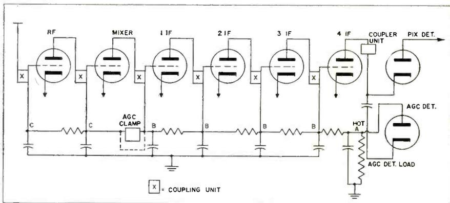
Fig. 3—Skeletonized diagram showing agc detector and stages that may be controlled by it.
