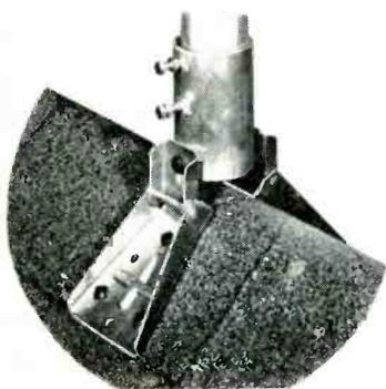
feature extremely thick sleeve walls and embossed rib construction for greater strength. An exclusive self-locking feature permits the mast to be completely self-supporting when it is swung into a vertical position. The serviceman is then left with both hands free to secure the guy wires and tighten the bolts. Channel Master Corp., Ellenville, N. Y.—TECHNICIAN (Ask for No. 4-2)
