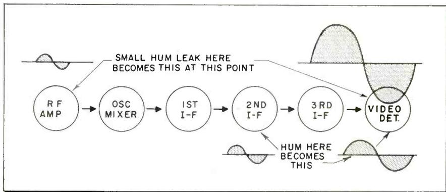
Fig. 4—Hum originating at the front of the receiver is amplified by succeeding i-f stages.
