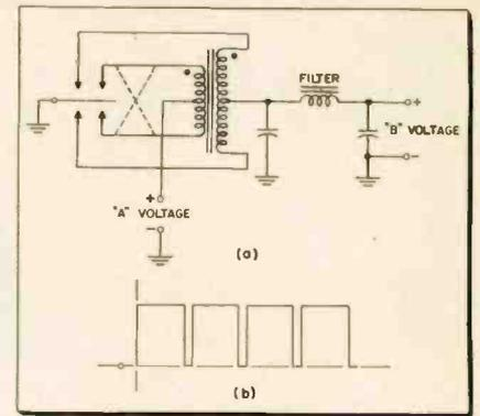
Fig. 5A—Circuit of synchronous or self-rectifying vibrator. B—Pulsed output waveform.
