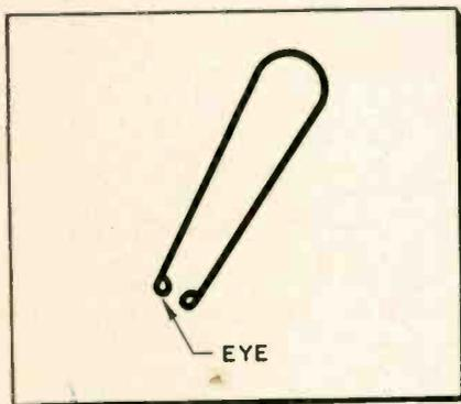
Home-made tweezers lift ball bearings easily.
