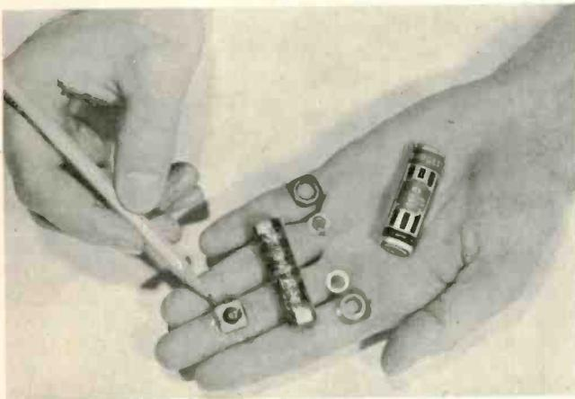
13 midget wafer cells (l) go into new 22½-v. Burgess battery (r). Cell consists of manganese dioxide mix between discs of zinc and carbon. Old carbon rod has been replaced by small piece of conductive carbon. These smaller, improved units are a result of automation
