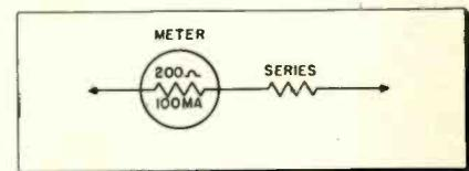
Fig. 4—Series resistor for voltmeter use.
