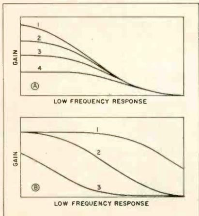
sake of simplicity, by arrows. Adjusting the value of capacitor  $C_1$  (or selecting another value with the switch) varies the frequency at which bass-boost action begins, known as the turnover point. Three different values of capacitance, for example, will produce the three different curves of Fig. 2B.
