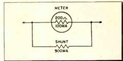
Fig. 3—Determining value of shunt resistor needed to increase meter's current capacity.
