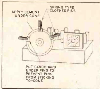
Fig. 2—Cementing loose speaker cones quickly.
