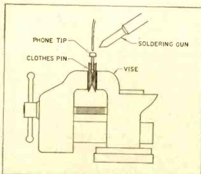
draws off heat applied by the iron. This idea is particularly useful when soldering the wire from a test prod or headphone into a phone tip—a job that is often necessary.
