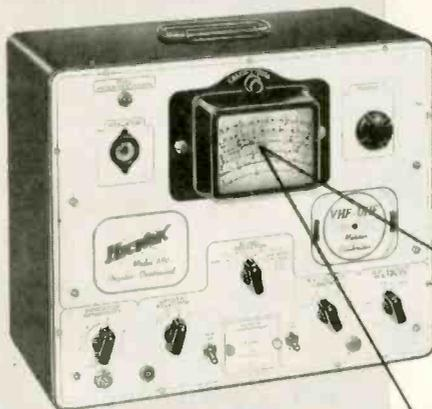
This unit features another HICKOK FIRST—A Non-Parallax shadow type dial provides a 300% magnification of scale, permitting exact settings for most accurate readings, and can be viewed from any angle without error.
