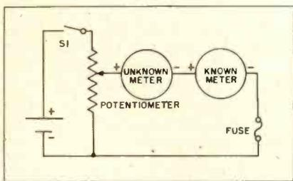
Fig. 1—Set-up for finding maximum current capacity and calibrating current readings.
