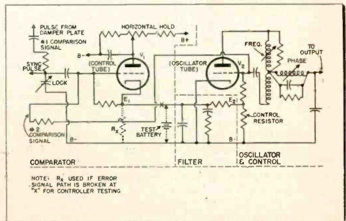
and note if a change has taken place in the meter connected to the discriminator output. Preferably, however, we break the feedback line carrying  $E_2$  to the corrector grid, connect it with a resistance to ground (or any bias required) as in Fig. 2, apply a voltage (say from a flashlight cell) to this grid and observe our meter (on dc, of course) monitoring  $E_1$ . The point for the break and the connections for the test battery are shown in Fig. 2 and in Fig. 1 in dotted lines.
