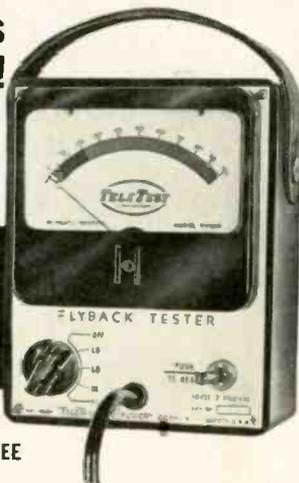
Engineered for the cost-conscious serviceman, here is the first and only flyback tester that reveals even one-turn shorts without a reference transformer for comparison!! This reliable test unit indicates true flyback condition under full operating voltage—100% of the time!
