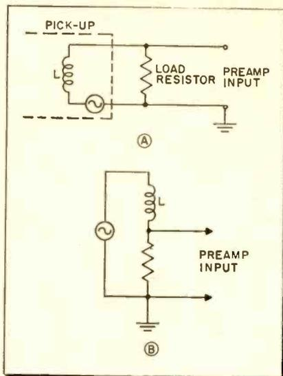
Fig. 6—Load resistor plus cartridge inductance provide roll-off in magnetic pickups.
