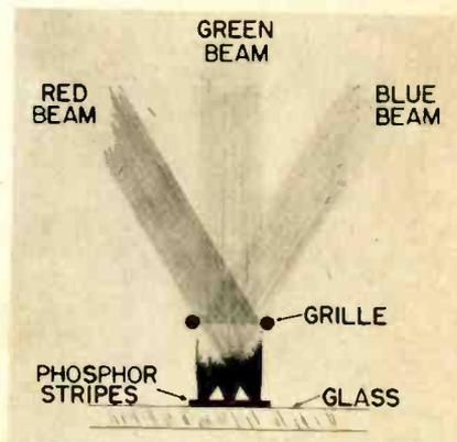
Fig. 2—How grille wires act to spot-focus color beams on appropriate phosphor stripes.
