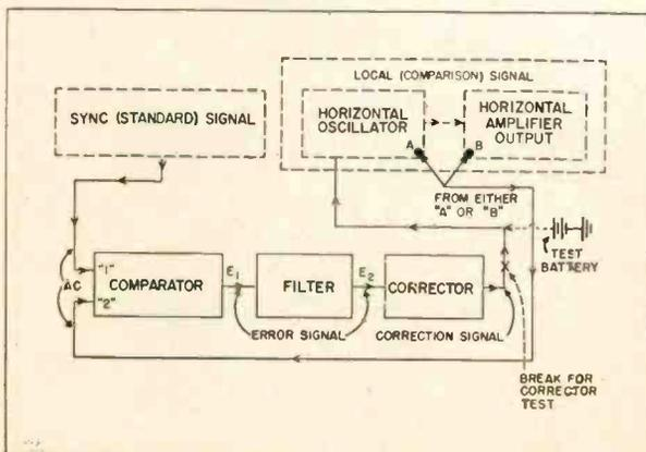
Fig. 2—The synchrolock system analyzed into units for troubleshooting.
