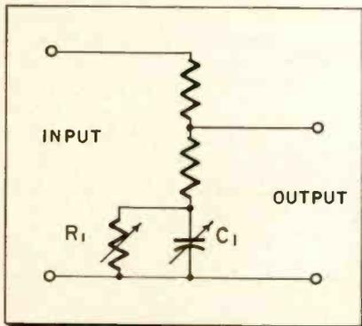
Fig. 1—Typical bass-boost equalizer network.
