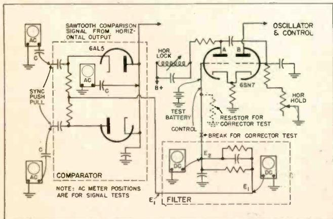
Fig. 4—Functional units of the synchroguide or pulse-width system.
