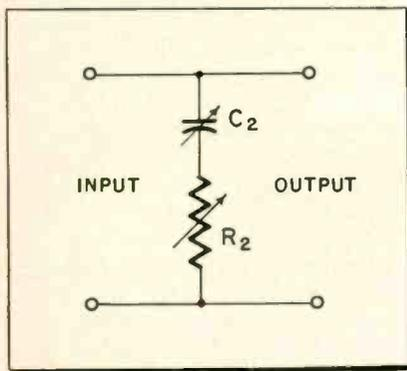
Fig. 3—Typical treble roll-off equalization.
