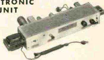
Unit above wires into set. Raster control unit (separate) reduces large pictures to 14" size when color is telecast. Switch restores original size for black and white viewing.
