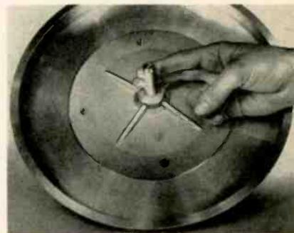
Fig. 2—Lubrication of the turntable shaft.
