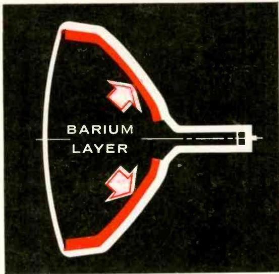
← "Silver Screen 85's" new barium "picture-guard" process deposits a lining of barium over the tube's inside walls. Increased "getter" action keeps the vacuum pure, protecting the screen and electron gun from contamination. The result: Silver Screen 85 gives a brighter picture for a longer time.
