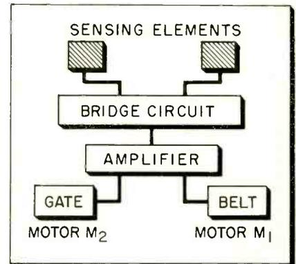
Fig. 2—Functional diagram of components involved in ore loading operations.
