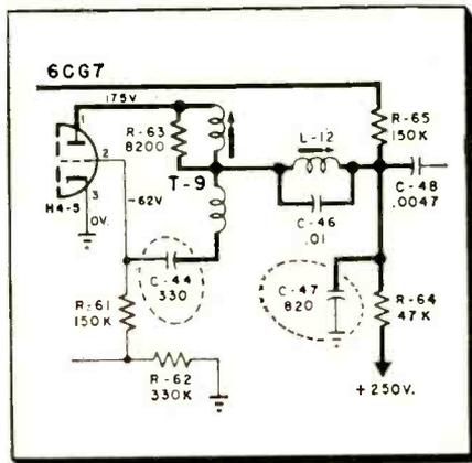
Fig. 1—Horizontal drift is often traced to a defective 330 or 820 μmf capacitor.
