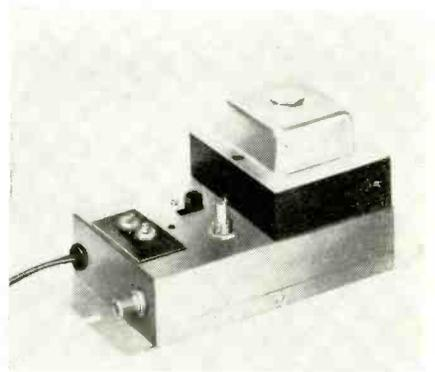
4.5 db maximum for low channels and 6 db maximum for high channels, eliminates snowy pictures in fringe areas. A newly designed power supply incorporates a switch for adjusting the voltage for various cable lengths. \$79.95. Jerrold Electronics Corp., 15th & Lehigh Aves., Philadelphia 32, Pa.
