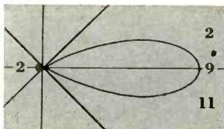
A dramatic breakthrough in TV antenna performance! The T-Bird provides extra-gain on every channel for snow-proof pictures, *plus* a directivity pattern that has no side lobes—clean as a whistle—for the sharpest, clearest pictures ever seen on any TV set...
