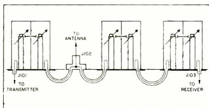
Fig. 8—Antenna multiplexer enables simultaneous transmission and reception on one microwave antenna.
