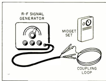
Fig. 3—Aligning a midget transistor radio can be simplified by using a three or four inch scramble-wound loop made of 12 to 18 turns of insulated wire to loosely couple r-f from a signal generator into the radio.
