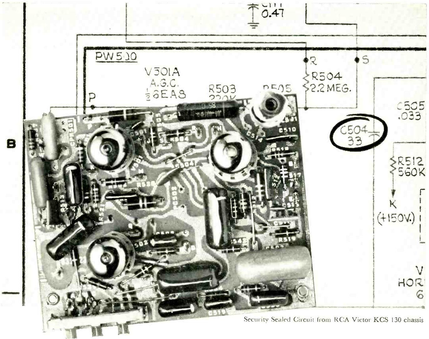
Security Sealed Circuit from RCA Victor KCS 130 chassis
