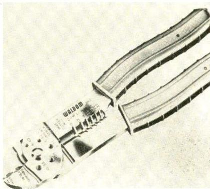
through 10; cuts wire; strips wire; and shears bolts and screws in sizes 4-40, 6-32, 8-32, 10-24 and 10-32. The tool cuts screws clean and ready for use without deburring. \$4.25. Waldom Electronics, Inc., 4625 W. 53rd St., Chicago 32, Ill.
