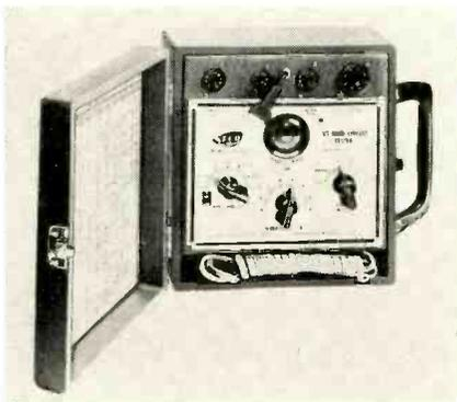
grid emission, leakage, shorts and gas in one operation; and indicates results instantly on a 6AF6 eye indicator. Two additional testing features: cathode continuity check; and complete inter-element short test, with shorts identified to pin numbers. GCT-9S shown, \$32.95. GCT-9W, \$34.95. Seco Electronics, Inc., 5015 Penn Ave. South, Minneapolis, Minn.
