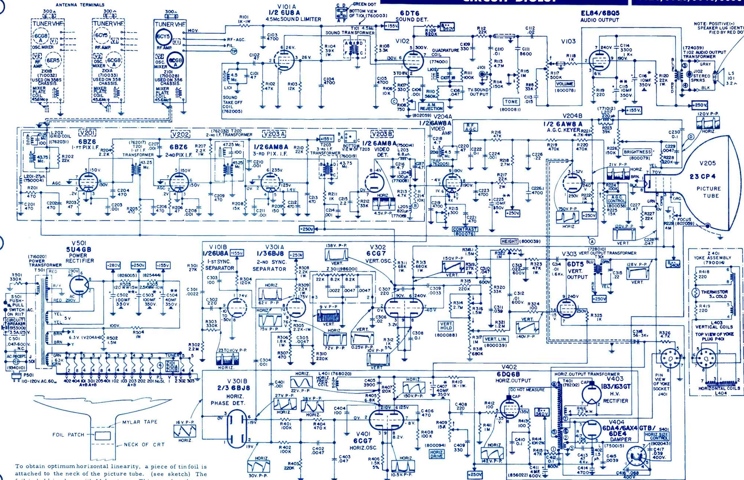
To obtain optimum horizontal linearity, a piece of tinfoil is attached to the neck of the picture tube. (see sketch) The foil is held in place with Mylar tape. This tape has the required high voltage breakdown potential. The foil should be removed from the old picture tube and placed on the neck of the new replacement picture tube, before the replacement tube is installed.
