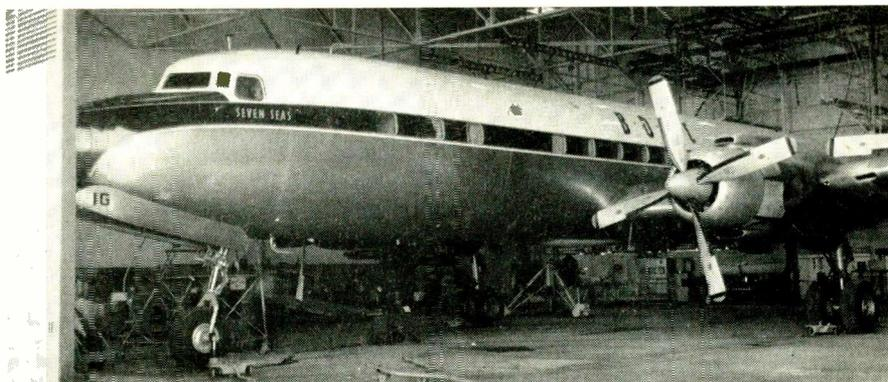
Fig. 4—Heavy aircraft is weighed by mounting strain gages on ram jacks under each wheel. Aircraft's center-of-gravity can also be determined in a similar manner.
