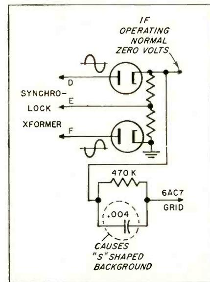
most exact" replacement. A technician making an earlier repair may have juggled the vertical plate load resistors and capacitors to get optimum sweep and linearity. Watch the components in old sets.
