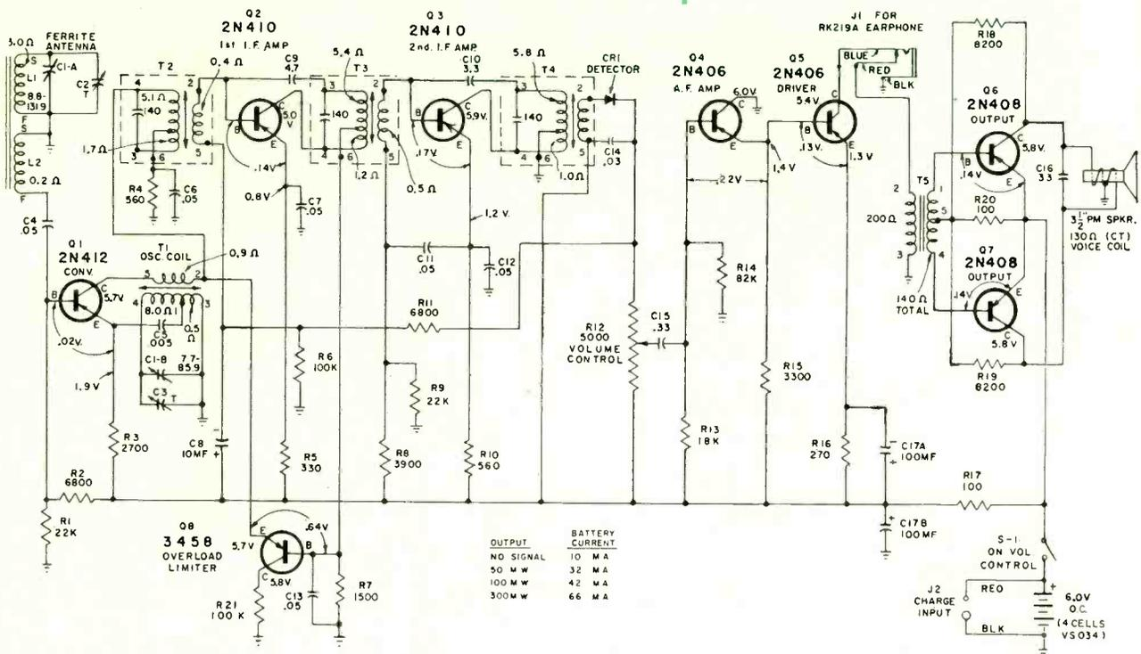
Fig. 1—Schematic of a deluxe-type portable transistor radio. Unit has a 300 mw push-pull output and uses a total of 8 transistors plus one diode as detector. Many transistor radios employ modified versions of the RCA circuitry shown here.
