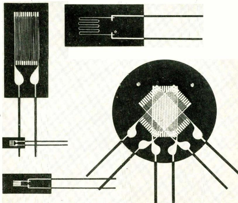
bridge's measurement arm due to temperature variations will cancel an equal change in resistance occurring in the strain gage in the second arm of the bridge. When the load bearing strain gage, and the "dummy" strain gage are exposed to the same temperature variations, the bridge will remain balanced even though the measuring strain gage may develop apparent strain because of ambient temperature variations. Thus, bridge output will be a true reflection of
