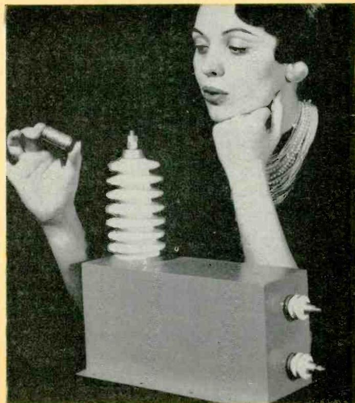
The attractive young lady is comparing a smaller resistor with what is claimed to be the largest precision resistor voltage divider built, according to the manufacturer, Resistance Products Co. The giant 30 meg, 100 to 1 divider operates at 30 kv with 0.05 accuracy. Ratio division was maintained within 0.01%.
