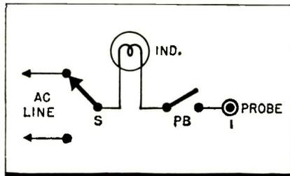
Fig. 1—"Hot chassis" checker helps unmask those 115 volt electrodes. Parts list: Ind.—3-watt, 115v bulb; J—probe jack; S—SPDT toggle; PB—normally open, press-to-close switch.
