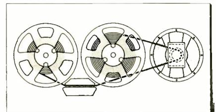
Fig. 3—Using the permanent magnet in a PM speaker to erase tape information.
