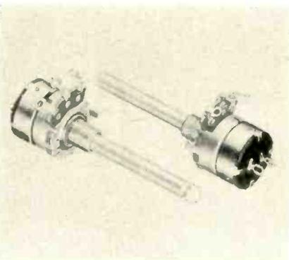
on many single-section and dual-section Stackpole variable resistors; and operates from the same shaft that controls the resistor. Single-pole, single-throw contacts are well isolated from solder flux and the entire mechanism is free from lubricants. Rating, 5 amperes at 125v a-c. Stackpole Carbon Co., St. Marys, Pa.
