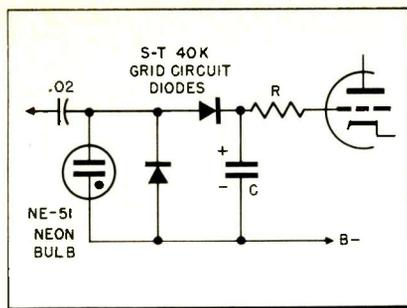
Fig. 3—Grid circuit modification for release delay. If "C" is very large with respect to the input capacitor, a start delay will produce a loss of part of the incoming signal.
