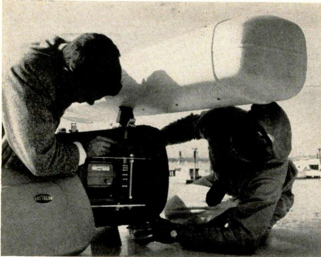
Fig. 1 (l)—Antenna unit mounted on open pedestal houses converter. Fiber gear is removed when tuning klystron.
