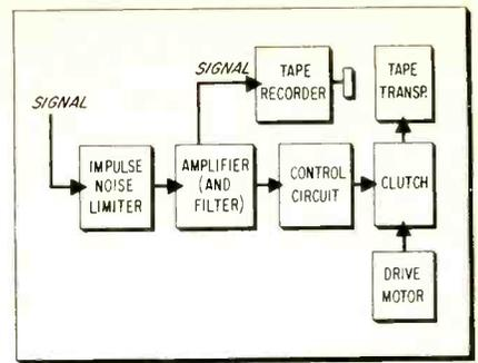
Fig. 1—Block diagram of signal-operated clutch drive circuitry.
