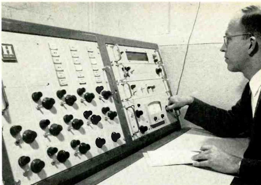
Fig. 2—Analog computer rapidly selects ice cream raw materials in correct proportions.
