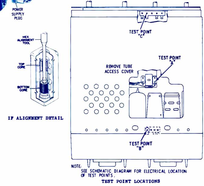
\* TO REMOVE TUBES AND SHIELDS INSERT SCREWDRIVER IN SLOT & PRY UP.
