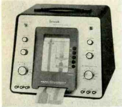
each analog channel. Sensitivities down to 10 mv per millimeter of pen excursion. Power source, 12v internal. Full scale deflection from center  $\pm 200$  mv. Measurement range, from 0.010 to 400v. Frequency response, from d-c to 100 cps. Price \$1450.00. Brush Instruments Div., Clevite Corp., 37th & Perkins, Cleveland 14, Ohio.
