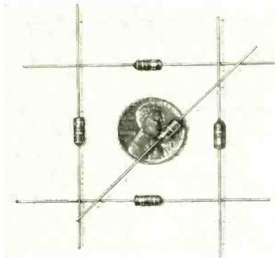
amperes over the operating temperature range from -65° C to -130° C. Peak reverse voltage range, from 225 to 600v. Capable of high temperature operation, 150 ma current output at 100° C. \$0.75 to \$1.75 in quantities of 1-99. International Rectifier Corp., 1521 E. Grand Ave., El Segundo, Calif.
