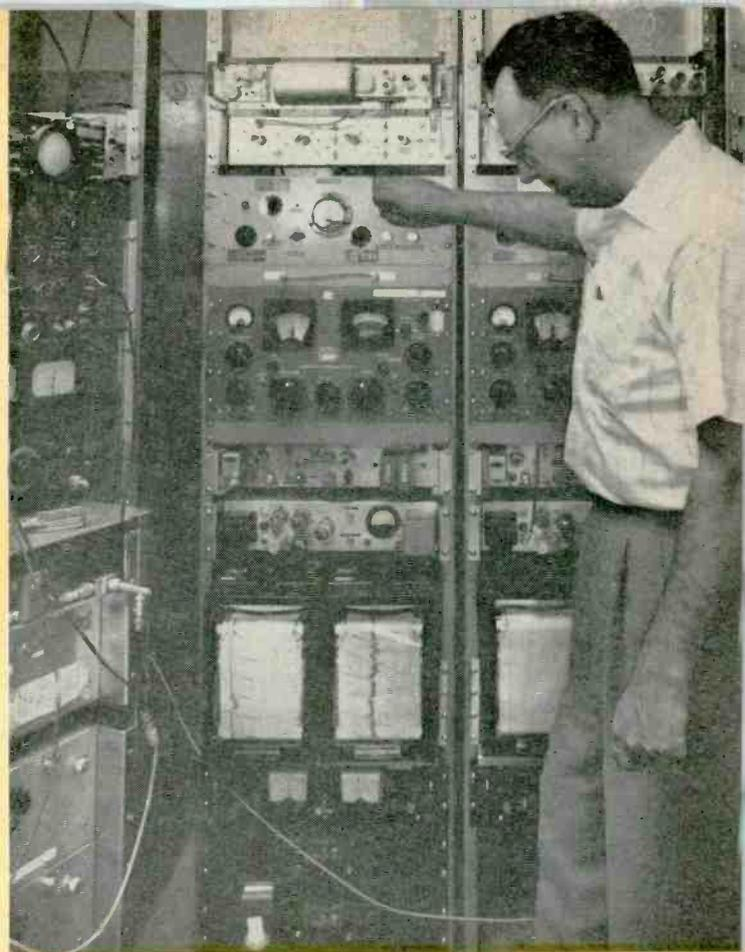
Modulation systems engineer, Harry Patrie, adjusts fading rate recorder developed at National Bureau of Standards. A strip chart records received radio signal fade-rate, the number of times per second that a signal envelope crosses the average level with a positive slope.
