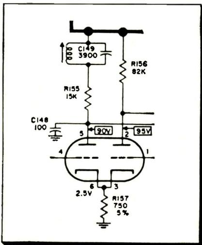
Fig. 3—Resistors changing value in multivibrator cathode coupled sync circuits play havoc with hold range.
