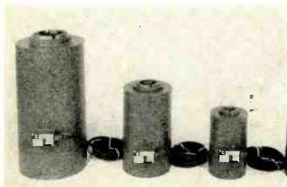
Fig. 6—Three sizes of strain gage load cells with terminal blocks and cables attached.
