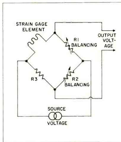
Fig. 7—When weight is applied to the strain gage (as one bridge arm), the bridge becomes unbalanced and its output can be employed for measurements or for initiating a variety of control operations.
