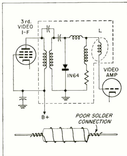
Fig. 1—Cold solder connection on peaking coil caused intermittent video, but, did not disturb 4.5 mc sound output.
