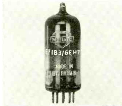
low microphonics; internally shielded; and proven reliability and trouble free performance. Characteristics of EF183/6EH7, a variable-mu r-f pentode: transconductance, 13,000 micromhos; plate voltage, 200v; plate current, 12 ma; heater voltage, 6.3v; and current .3 amp. International Electronics Corp., 81 Spring St., New York 12, N. Y.
