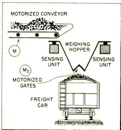
Fig. 1—Strain gages under ore hopper stops conveyor belt when proper ore weight is reached. Hopper discharges ore automatically and loading cycle is repeated.
