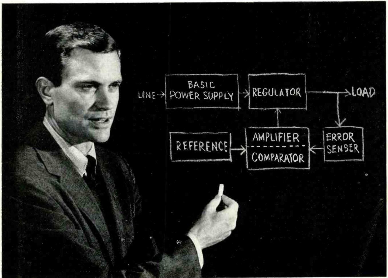
**P**ICTURED above is a block diagram of an electronically regulated power supply. It's the subject of the latest issue of Tung-Sol's monthly series for the industrial serviceman, *Tung-Sol Tips*. And it's must reading if you're going to deliver fast and efficient trouble shooting service to your customers. Or if you work with dc supplies in your laboratory. That's because Issue #11 of *Tips* delivers quickly and clearly the ins and outs of modern dc power supply equipment.
