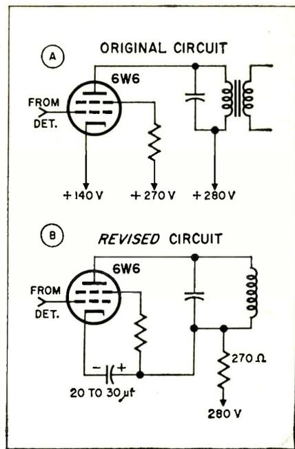
Fig. 5—(A) Hum and buzz in this audio output circuit could not be reduced. (B) When circuit shown above was modified as shown here, hum and buzz were reduced.
