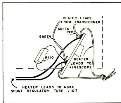
ering the cathode temperature of the CRT. The resistor is only effective if placed in the circuit simultaneously with the replacement 21CP22 CRT.
