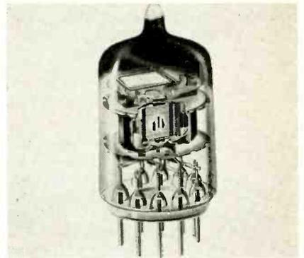
quency range 50-2,000 cps. Type 7308 is a high gain, twin triode, similar to the 6922, designed for use in radar, oscilloscopes, computers, broadband amplifiers and critical airborne applications. Transconductance, 12,500 micromhos. Amperex Electronic Corp., Semiconductor and Special Purpose Tube Dept., 230 Duffy Ave., Hicksville, L. I., N. Y.
