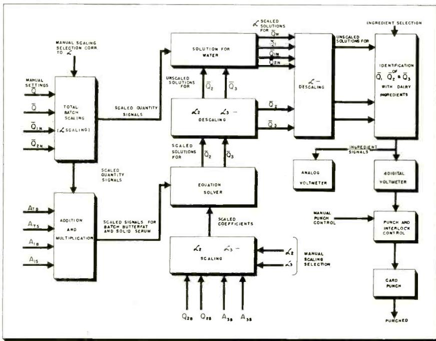
Fig. 3—Functional diagram of computer, including digital card punch control section.
