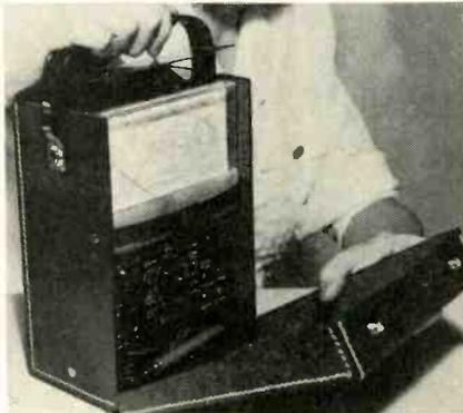
meter in factory-wired or kit form. The case has an optional user price of \$4.95. Features of the WV-38A include a 20,000 ohms-per-volt meter movement and separate 1v and 0.25v d-c range. Radio Corp. of America, 30 Rockefeller Plaza, New York 20, N. Y.
