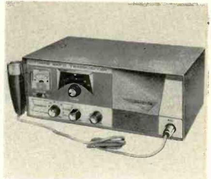
trolled transmit positions. Also included: adjustable squelch control; automatic series gate limiter; push-to-talk ceramic microphone and relay; and illuminated dial. \$99.50. Lafayette Radio Electronics Corp., 165-08 Liberty Ave., Jamaica 33, N. Y.
