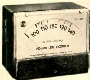
**POWER LINE MONITOR RCA WV-120A** Provides a constant check on incoming line voltage. Responds to every voltage fluctuation. Highly accurate ( $\pm 2\%$  at 120 volts). Gives true rms reading. 5" wide meter. \$14.95\*
