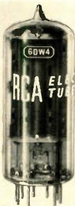
A half-wave no-var vacuum rectifier tube, 6DW4, is designed especially for damper service in horizontal-deflection circuits of color and BW TV sets. It is rated to withstand a maximum peak plate current of 1300 ma and a maximum d-c plate current of 210 ma. Has insulation between heater and cathode to withstand negative peak pulses between the heater and cathode of 4500 v with a d-c component up to 900 v RCA, Electron Tube Division.
