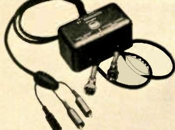
**RF MODULATOR RCA WG-304B** Used to check overall frequency response of TV receivers, including COLOR. Permits modulation of a signal from a marker generator by a signal from a sweep generator. \$12.50\*
