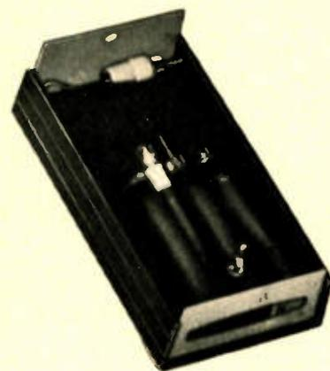
The model HM-10 is a departure from dip meters in that a tunnel diode is the oscillating element. The instrument uses meter indication which is driven by a three-transistor amplifier. Batteries power the unit so it can be used anywhere. A temperature restriction is placed on the instrument, however, it will not
