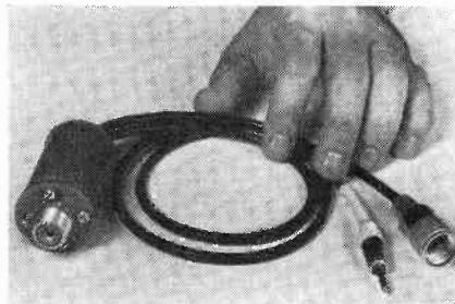
a standard a-m automobile radio. Designated the CBC-1, the coupler reportedly has extremely low insertion loss. Tests have shown maximum loss to be less than 0.3 db between transceiver and antenna. The antenna cable is connected to a SO-239 input plug that is completely potted for long life. A lead with a PL-259 plug is connected to the CB transceiver. A conventional am radio jack-plug connects the other lead to the standard broadcast receiver. Price: \$7.20 each. B & K Div., Dynascan Corp.
