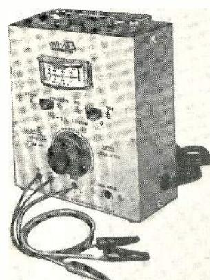
to the manufacturer, it features a bias tap control fully adjustable from 0 to 6 v, and provides complete filtering. Rated at 0-20 v, the continuously adjustable unit delivers a full 150 ma at this output. At 100 ma, it can deliver voltages as high as 24 v. An edge-reading meter with red pointer reads either output voltage (0-24 v) or output current (0-100 ma). Price: \$19.95. Electro Products Labs., Inc.
