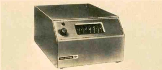
sets the number of the second telephone in a series of thumb wheels and switches the 'diverter' on. It then automatically dials the pre-set number—whether it is in the same building, another part of town, or in a distant State.
