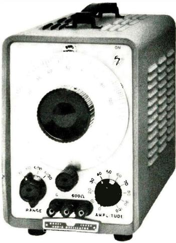
This audio oscillator uses traditional RC Wien-bridge circuit.
