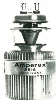
tetrode of the 3 kw plate dissipation class designed for use as an RF amplifier for frequencies extending throughout the VHF range. Both the control grid and screen grid connections are made to ring-type connectors brought out through the tube envelope. This facilitates operational performance by eliminating discontinuity in the impedance versus frequency characteristics. Amperex.
