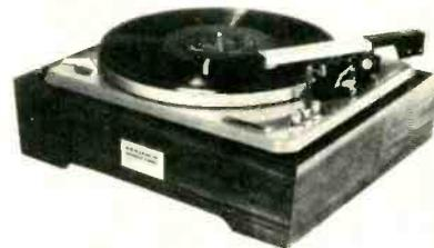
turntable platter and transcription arm. The 18H carries a suggested retail list price of \$119.50 — less cart-ridges and base. Specifications listed are: rumble -55db; wow and flutter, less than 0.1%, and stylus force gauge, 1 to 5 g. Benjamin Electronic.
