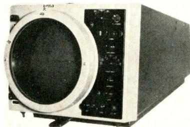
away. The unit has six range markers with variable intensity controls on all seven ranges:  $\frac{1}{2}$ , 1 $\frac{1}{2}$ , 3, 6, 12, 20, and 48 miles. Raytheon.
