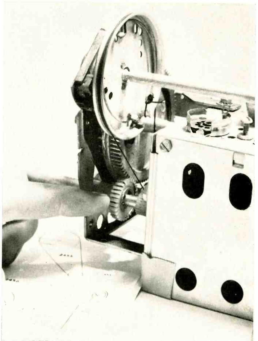
Replacing dial cord and plastic gear drive on Sylvania UHF/VHF tuner.
