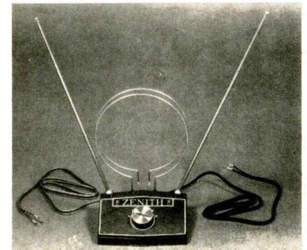
behind the other. These loops are inter-connected through a broad band, hybrid isolating network which phases them through the entire UHF spectrum. The VHF and UHF elements of the antenna have a chrome plating; the base, a brown color with silver color trim. Zenith.
