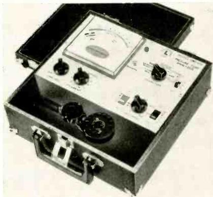
minimum emission. This provides a method of comparing the three color guns, simulating the actual operating conditions of the color set in use. Lectrotech.
