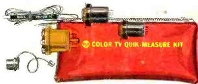
The RCA Color TV "Quik-Measure" Kit (1A1569)—Helps you measure both voltage and current at any tube pin in a color set without pulling the chassis from the cabinet or unsoldering leads. The kit contains 7 and 9 pin socket adaptors for miniature tubes, an 8 pin socket adaptor for octal tubes, a top cap extension lead and a current measuring probe.
