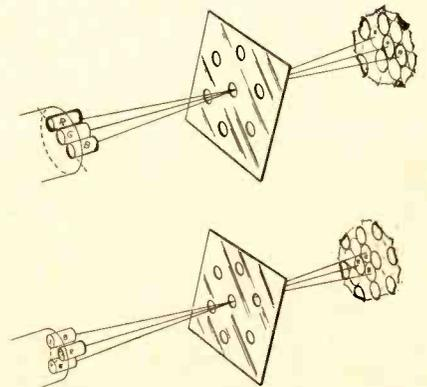
(Top) In-line gun arrangement of G-E 11SP4 color CRT. (Bottom) Gun arrangement in conventional color CRT
