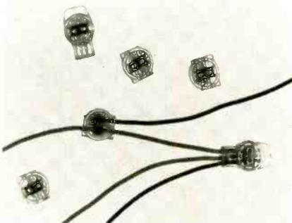
The pigtail connector is designed for connecting two or three wires. The tap connector is designed for making bridge splices on a "run" wire without interrupting or breaking the circuit. 3M.
