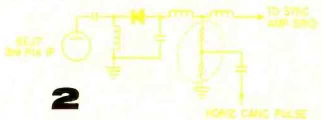
Fig. 3—Simplified typical blanker circuit.
