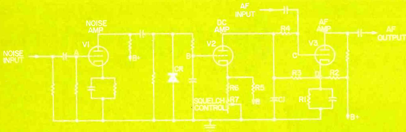
Fig. 4—Typical squelch circuit in two-way communications receiver.
