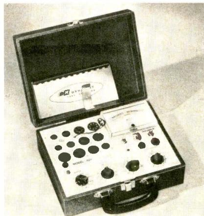
for shorts, grid emission, leakage, gas and cathode emission under simulated load conditions. Each section of multi-section tubes is checked. A reference index supplied with the tester contains a complete tube listing. B&K.
