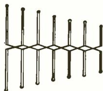
This unique system providing high gain, high front to back ratio was developed by Kay-Townes in 1954 and is the most copied system used in antenna design today, having been renamed by other manufacturers as LOG-PERIODIC, etc. Incorporated in this system is a solid rod, all-aluminum, one-piece construction with special insulator at every crossover point eliminating possible shortouts.
