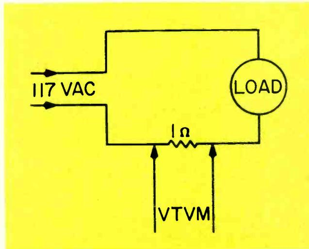
Fig. 2—Method of measuring current in an ac circuit.
