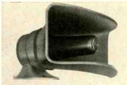
ance, 16Ω. Frequency response, 275-8000cps. Sound level, 127db measured 4 ft on axis, rated power. Dispersion, 120 deg x 60 deg. Dimen-
