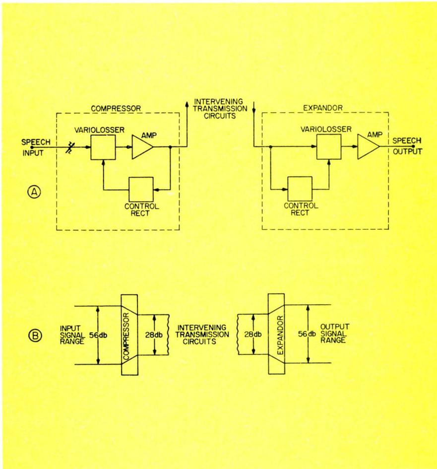
Fig. 2—The Comparator. (A)—Compressor and expander sections. (B)—How signals are compressed and expanded.
