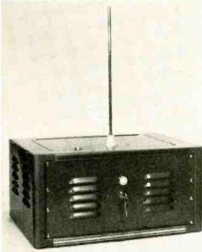
amplified and used to trigger an alarm which can be heard from some distance away. The microwave signal remains stable when no human movement in the area. The unit can also be used to trigger an alarm at a police station or detective agency. Radar Devices.
