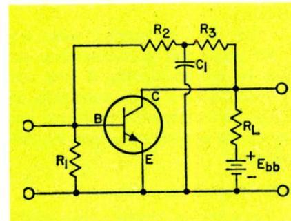
Fig. 2(A)—Bias network in common-emitter circuit uses emitter stabilizing resistor. (B)—Common-emitter circuit using split-voltage-divider bias network.
