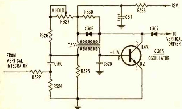
discharged below the cut off point, the transistor once again conducts and another cycle is started.
