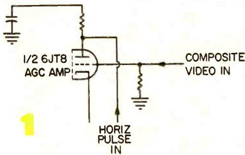
Fig. 1—Simplified typical AGC circuit.
