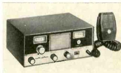
transistors, 8 diodes, and 2 Zener regulators. During receive operation the drain is 0.2 amp and when transmitting the maximum drain is 1.1 amp. Hallicrafters.
