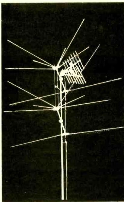
Fig. 2—A well-mounted UHF corner reflector gave poor reception because of losses in ordinary twin-lead.
