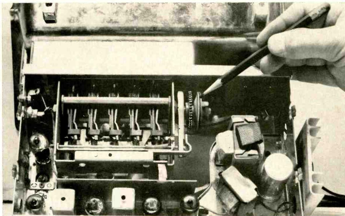
Check tension of slippage on sliding- and push-button car radios.
