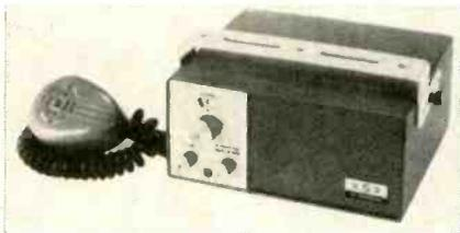
transmit/receive channels. The "SSS" has solid-state circuitry throughout (25 silicon transistors, 5 diodes and 1 zener diode). Low battery drain, less than 200ma dc on receive. The "SSS" is 8 x 3½ x 7 in. and weighs less than 4 lb. Squires-Sanders.
