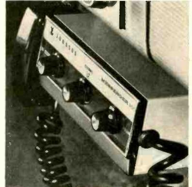
ceiver 6 3/16 x 2 1/3 x 8 1/2 in. It is suited for mobile use in connection with the nationwide H-E-L-P (Highway Emergency Locating Plan) program. E. F. Johnson.
