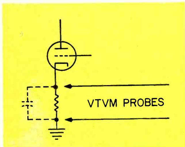
Fig. 1—Measure dc voltage across the cathode bias resistor and use ohm's E/R formula to determine approximate current.
