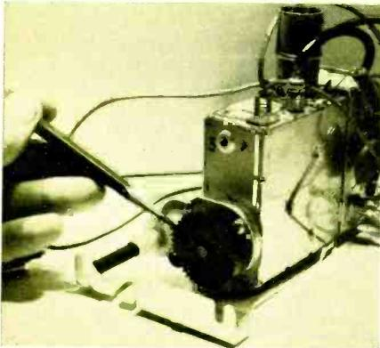
Stripped plastic gear on RCA UHF tuning assembly.
