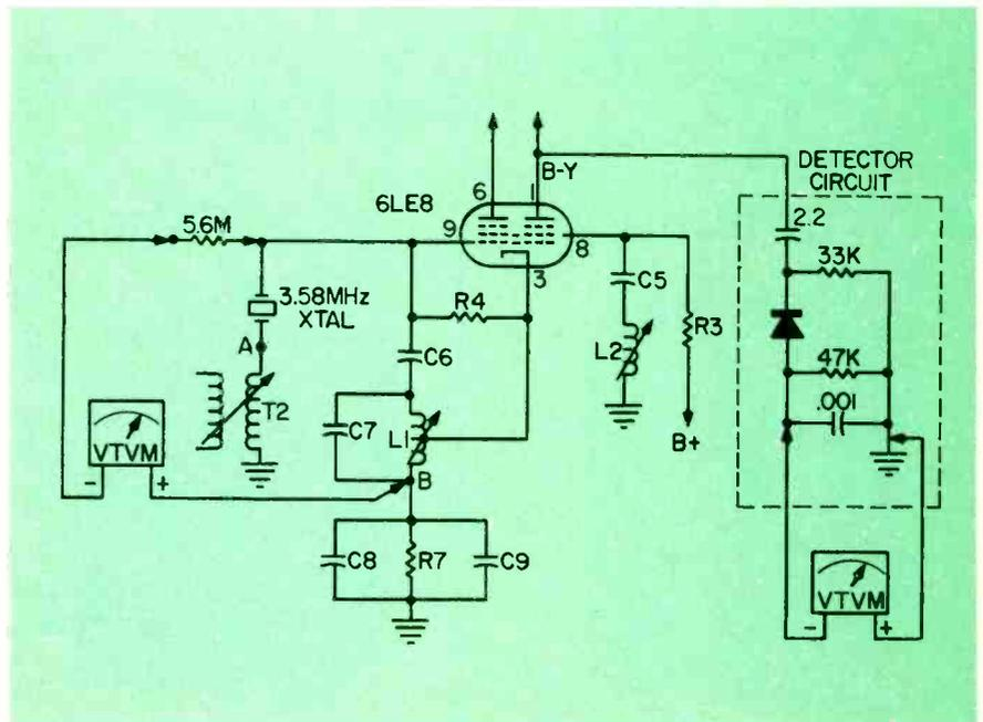
Fig. 2—Detector circuit used for aligning 3.58MHz trap in demodulator outputs
