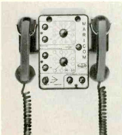
Control unit for multi-channel VHF/FM marine radiotelephone by Comco.
