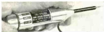
ity in low frequency testing and low impedance circuits. Has 10-capacity section to trace wave forms in high impedance circuits, reduce distortion and frequency discrimination. Lo-capacity section provides 10 to 1 attenuation when used with scope having input resistance of 1.3M. Far Hills.
