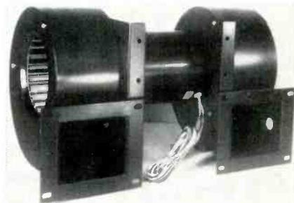
computers, consoles or systems is announced. Motor and blower can rotate to blast in any direction. Motors may be mounted on right or left side of blower and are available in clockwise or counterclockwise rotations. McLean.
