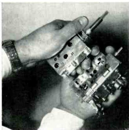
Transistorized UHF and VHF tuners. Strange looking units compared to their electron tube counterparts.
