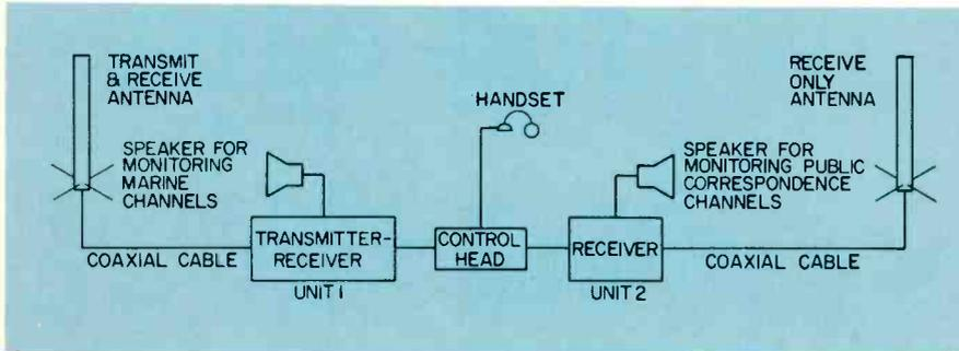
Fig. 2—Combination simplex and duplex marine radio system.
