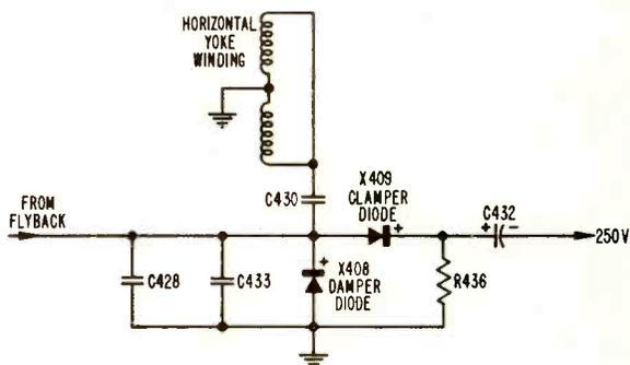
The entire pulse lasts for about 22μsec of the total horizontal scan time of 63μsec. This time, then, represents the "on" time of the oscillator.
