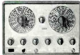
**Model 369** Sweep/Marker Generator for easiest, fastest visual alignment of color or B&W TV and FM RF and IF circuits. Five sweep ranges from 3-220mc. Four marker ranges from 2-225mc. Crystal marker oscillator. Post injection of markers. **\$89.95** kit, **\$139.95** wired.
