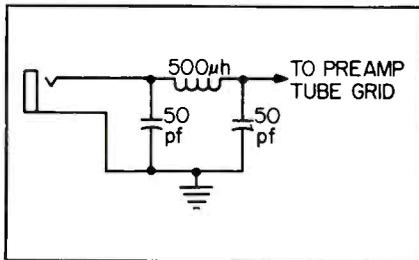
Fig. 4—Pi-trap inserted between mike cable jack and 1st preamp grid.
