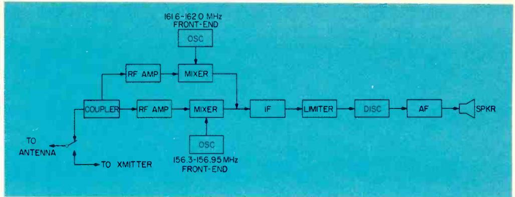
Fig. 1—Some VHF receivers have two front ends.
