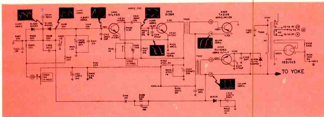
Some horizontal systems look foreign in transistor sets. The output transistor generally feeds the yoke directly.
