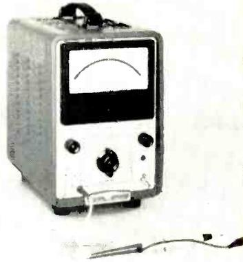
Fig. 3—Pico-ammeter and micro-voltmeter has a full-scale dc current range of 10pa. The current of 10pa is measured as a voltage drop of 10 $\mu$ v across an internal 1M resistor. Hewlett-Packard model 425A.
