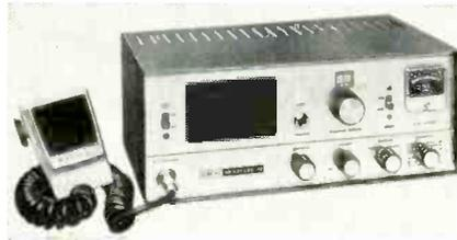
noise limiter, plus switches for 3.5w public address use, spotting and Part 15 operation, are all incorporated. Transistorized dual power supply operates from 12vdc and 117vac. Eico.
