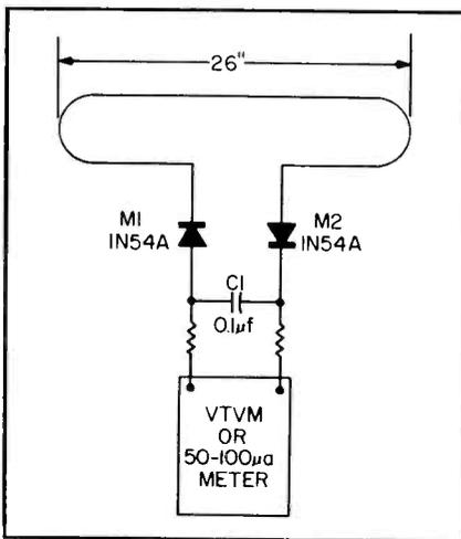
Fig. 5—Simple strength meter for measuring intensity of radar signal.
