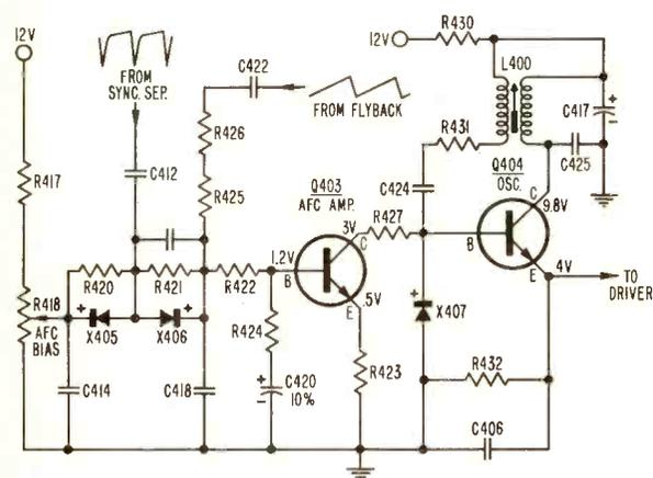
voltage which is direct-coupled to the base of AFC amplifier, Q403. The network of C422, R426 and R425 reshape the sawtooth waveform being fed back from the flyback for use by the AFC network.
