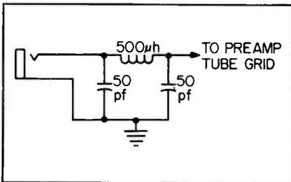
Fig. 4—Pi-trap inserted between mike cable jack and 1st preamp grid.
