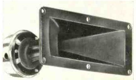
with 8Ω impedance and Alnico v magnetic driver unit. Frequency response is between 1.5 and 20kHz. Crossover frequency is 2kHz. Oxford.
