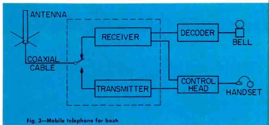
Fig. 3—Mobile telephone for boat
