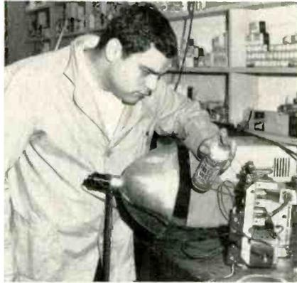
Marty Brown's 'heat-lamp/quick-freeze' checking is fast and efficient.
