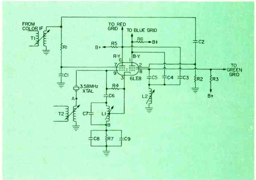
Fig. 1 — Oscillator-demodulator circuit employing 6LE8
