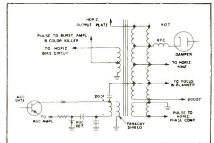
Fig. 3—Horizontal output transformer circuit details
