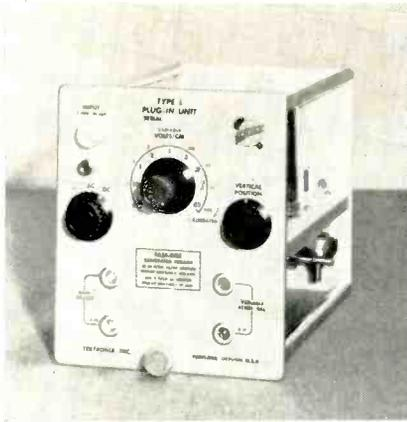
Fig. 2—Fast risetime preamp plug-in unit for scope vertical amplifier. Has risetime of 6 nsec. Tektronix, type L.
