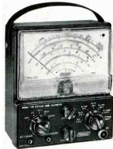
frequency response ( $\pm 5\%$ ) 30Hz to 500kHz; dc ranges; 0-1.5, 5, 15, 50, 150, 500, 1500v with input impedance 11M shunted by 2pf  $\pm 2\%$ ; resistance ranges: 0-1K, 10K, 100K, 1M, 10M, 100M, 1000M  $\pm 3\%$ . Mercury.
