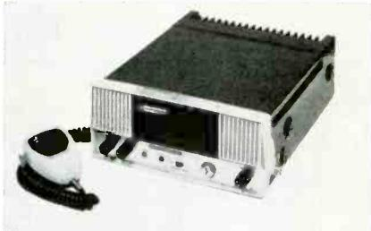
output is 5w with less than 5% distortion. Plug-in channel elements provide one through four channels. The tone-coded squelch option reduces the possibility of hearing other systems that share a channel. The radio is also designed for easy field conversion to split-channel operation when such changes are required. Motorola.
