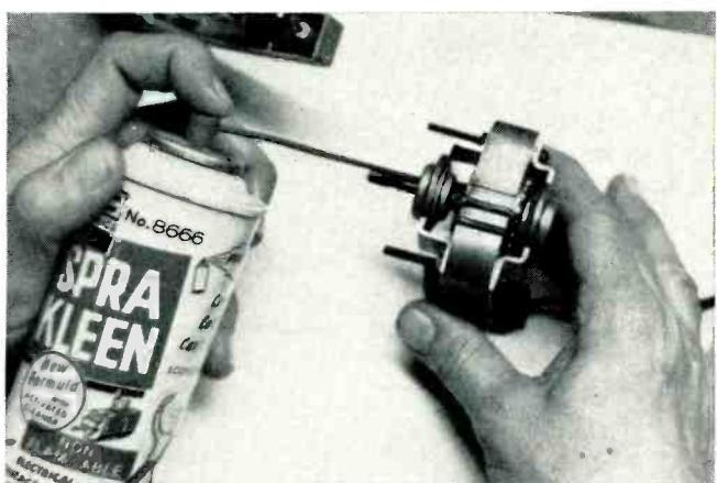
Cleaning motor bearings with bearing-plate removed.
