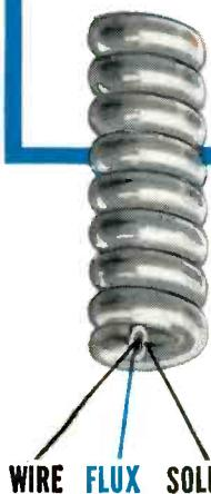
The KWIKETTE SOLDERING AID is not just another wire spring connector! It has a Copperweld wire inner core, an intermediate layer of flux, and an outer jacket of solder . . . *all you need is heat!*
