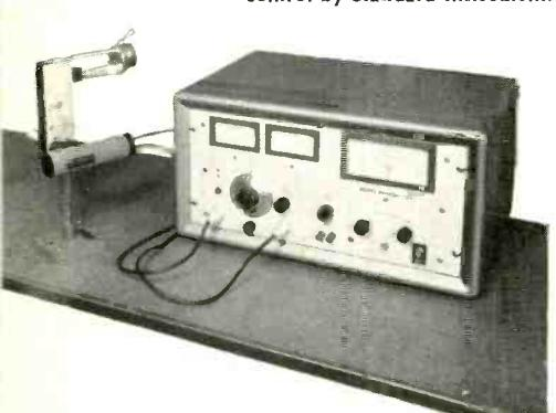
A photometer, one of many instruments that use photoelectric sensing. Courtesy Modern Electronics.
