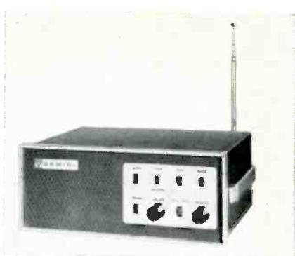
is announced. As an FM alerting receiver, the unit remains on silent standby until activated by a tone signal transmitted from headquarters. It can then receive voice messages at full sensitivity. The receiver is offered in the low (30 — 50MHz) or high (150 — 174MHz) bands with other frequencies available on special order. A number of optional features are available. Viking Inst.
