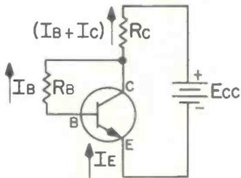
Fig. 7—Collector-to-base feedback improves transistor stabilization.
