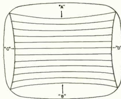
tical sweep current and a horizontal sinewave current supplied by the current generator. The amplitude of the correction current is highest at the beginning and end of the vertical scan period and will progressively decrease to zero as the vertical sweep current passes through zero — which is coinci-
