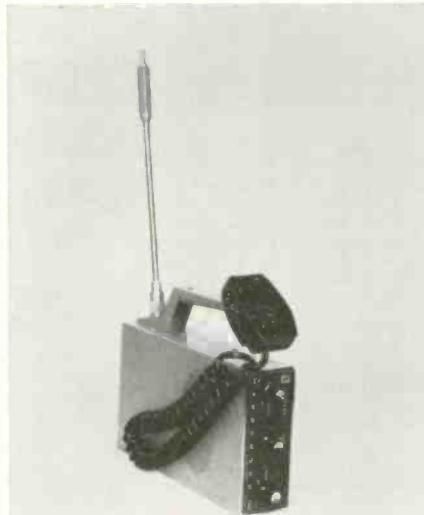
provides up to 8 hours of full power, portable operation before the nickel cadmium battery requires recharging. The unit adds 3 inches to the over-all length of the transceiver. Price is \$69.95. Johnson.
