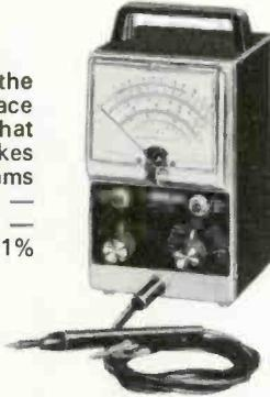
**Complete Service / Laboratory Transistor Analyzer** ... the Heathkit IM-30 provides thorough DC analysis of PNP & NPN transistors. Test for shorts, DC gain (Beta 0-300) (Alpha 0-0.9967), Leakage (Icbo, Iceo), and diode forward & reverse current. Requires 7 "D" cells for internal power — provisions for external power.
