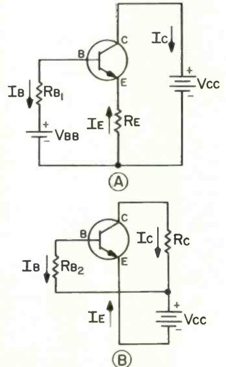
Fig. 2 (A and B)—Common-emitter voltage sources are combined by increasing  $R_B$ .
