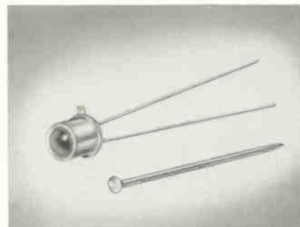
current output at 500 footcandles is  $180\mu a$ . The spectral response peak is at 0.85 microns. Speed of response,  $1\mu s$ . Temperature range,  $-60^{\circ}C$  to  $+125^{\circ}C$ . Price \$2.25. National.
