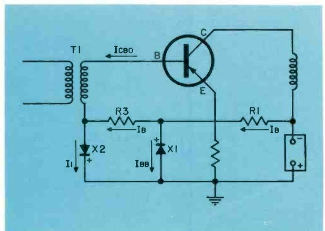
capability of X2 also increases so that the diode is able to pass additional current. Since current through X2 consists of a portion of  $I_b$ , more current flows through R1 and R3 —increasing the voltage drop across both. This reduces the amount of voltage available for forward bias. This reduction in forward bias, of course, decreases transistor current and keeps the transistor operating within its normal limitations.
