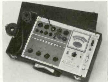
for proportionate screen brightness by qualitative measurement of the electron beam. The central area of the picture tube cathode is checked in addition to the controlling action of the first grid. The instrument weighs 8lb and measures 16 x 9 x 4¾ in. Net price \$92.95. Precise.
