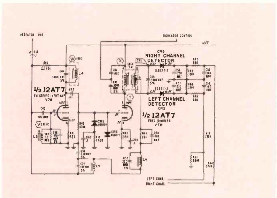
Fig. 4—Typical electron tube stereo multiplex circuit.
