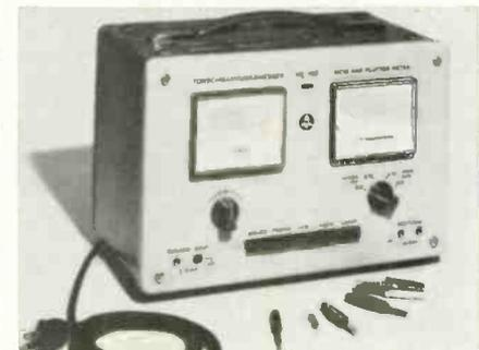
production testing and service work. The instrument is designed to read tone fluctuations from  $\pm 0.02$  to  $\pm 2.5\%$  or from  $\pm 0.01$  to  $\pm 0.75\%$ . A "drift" indicator measures up to  $\pm 4.5\%$  frequency deviation of the recorded tone from 3150Hz. The unit measures 7 x 8 x 11 $\frac{3}{4}$  in., weighs 11 lb. Prices range from \$375 to \$395. Gotham.
