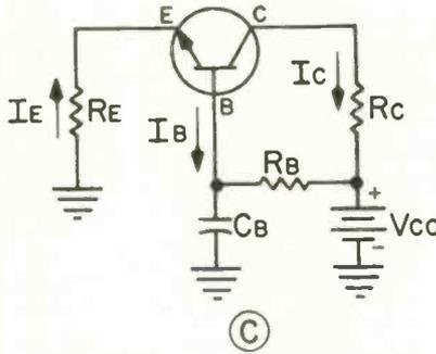
Fig. 4 (A, B and C)—Common-base circuit can be modified for single voltage source.
