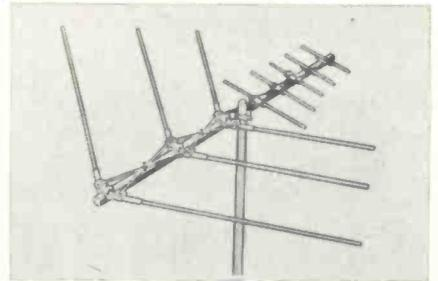
dwellers. It has three driven V dipoles that cover both VHF bands and three active dipoles plus three directors for UHF gain. The frequency response is flat within  $\frac{1}{2}$ db on any channel and a sharp forward lobe in the polar pattern assures unidirectional pickup with high front-to-back ratio on all channels, the announcement said. An indoor VHF/UHF splitter divides the signals for the TV set from the single download. Price \$17.50. JFD.
