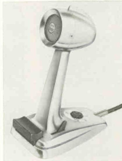
two stage silicon transistor amplifier built into the base provides a dual output impedance of 150 or 600Ω. The microphone is rated at 60Hz to 10kHz with less than 1% distortion. List price \$75. Turner.
