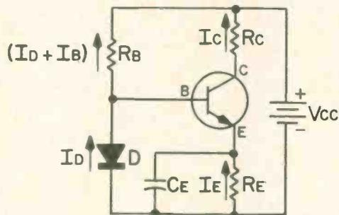
Fig. 11—Diodes compensate for relatively large temperature changes in transistors.
