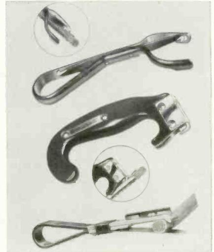
used for slitting most types of cable jackets, especially the outdoor heavy-duty types; stripping the jacket from all sizes of inside types of plastic and fabric covered cable; and "ring" cutting the sheathing of inside types plastic, fabric or rubber covered cable. The cut through the sheathing is limited to 1/32 in. for protecting the wires. P. K. Neuses, Inc.
