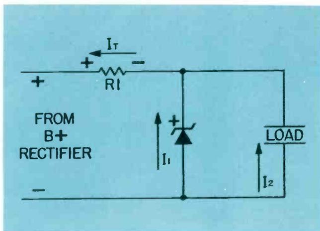
Fig. 5—Zener diode being used as a voltage regulator.
