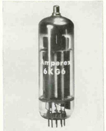
design characteristics developed to eliminate Barkhausen oscillations. As a result, the manufacturer claims snivet-suppression circuits can be eliminated, resulting in lower circuit costs. Maximum peak plate, 7000v. Maximum plate dissipation, 34w. Peak anode current, 1.4a. Ampex.
