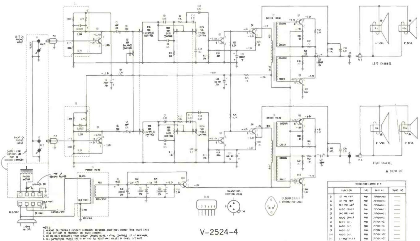
Fig. 4—Schematic of V-2524-4 Westinghouse stereo phono amplifier.
