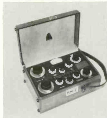
accuracy of 3% from 535 kHz to 1605kHz. The signal generator is said to have a calibrated output from 10mv to 1v with an accuracy of  $\pm 1\%$ , and frequency range of from 535kHz to 1605kHz with a readout accuracy of  $\pm 3\%$ . The monitor receiver is designed for sensitivity of better than 5mv, weight, 12 lb. Wilkinson.
