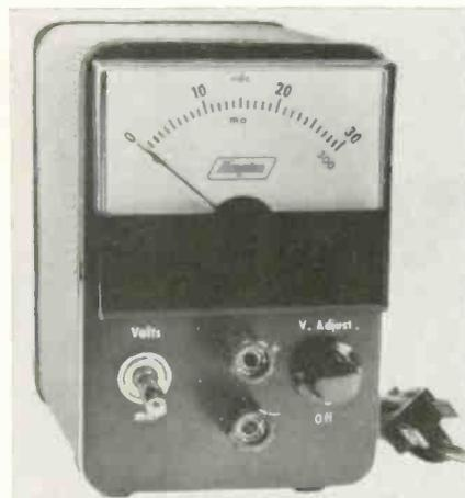
300ma over a range of 1.25 to 30vdc with a load regulation of ±0.5% or 50mv, whichever is greater; has a 10mv line regulation over a range of 105 to 125v and a full load ripple of 1mv RMS. It stands 5¾ in. high and weighs 3 lb. Acopian Corp.
