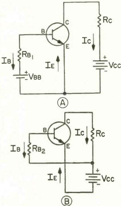
Fig. 3 (A and B)—Common-collector voltage sources are combined by increasing  $R_B$ . emitter amplifier (Fig. 3B). By increasing the base resistor ( $R_B$ ), the same emitter-to-base voltage ( $V_{EB}$ ) and base current ( $I_B$ ) can be obtained from the higher collector-to-emitter voltage source ( $V_{CC}$ ).
