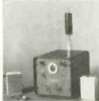
A 27MHz wireless cuing system for TV and radio studios is now available. The transmitter includes a simple 3ft whip antenna, covers up to 8000 sq. ft. studio areas and can be remotely operated with a
