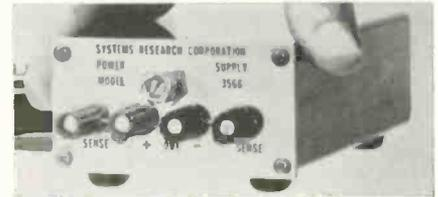
voltage is adjustable at the front panel from 4 to 25v at 200 ma. Price \$79. Systems Research.
