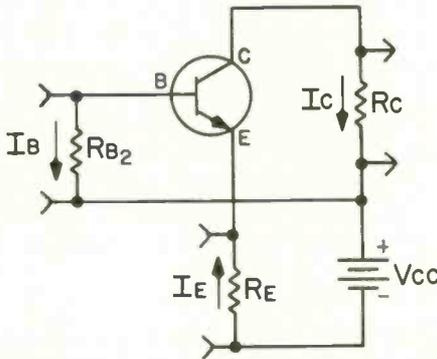
Fig. 5—The compound circuit can be modified to use a single voltage source.
