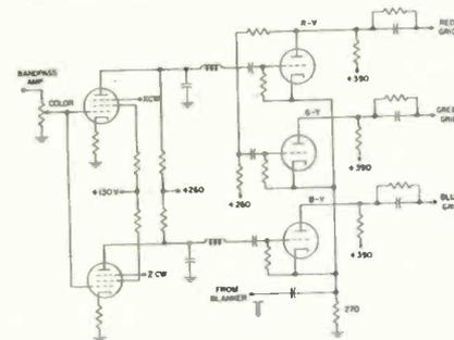
blocks the relatively low frequencies of the luminance signal. The chrominance signal is then coupled to the bandpass amplifier grid through the chroma take-off coil. This coil is broadly resonant to 3.58MHz and allows the color information to pass while attenuating all frequencies that are outside the passband.
