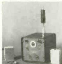
A 27MHz wireless cuing system for TV and radio studios is now available. The transmitter includes a simple 3ft whip antenna, covers up to 8000 sq. ft. studio areas and can be remotely operated with a
