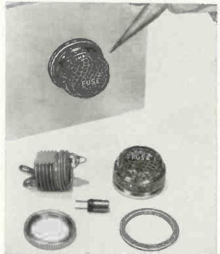
pregnated see-through molded plastic lens and a mesh imbedded silicon gasket that fits between the lens and the mounting surface of the chassis panel. When the fuse blows, under overload conditions the indicating light in the ember lens goes on alerting the user of the equipment. Price \$5. Littelfuse, Inc.
