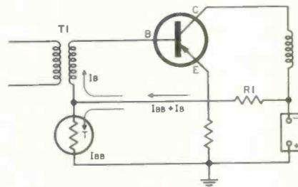
Fig. 3—Thermistor compensating circuit.
