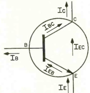
Fig. 6—Transistors contain various currents that are effected by temperature.
