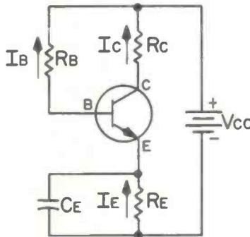
Fig. 8—Transistors can be stabilized with an "emitter swamping" circuit.
