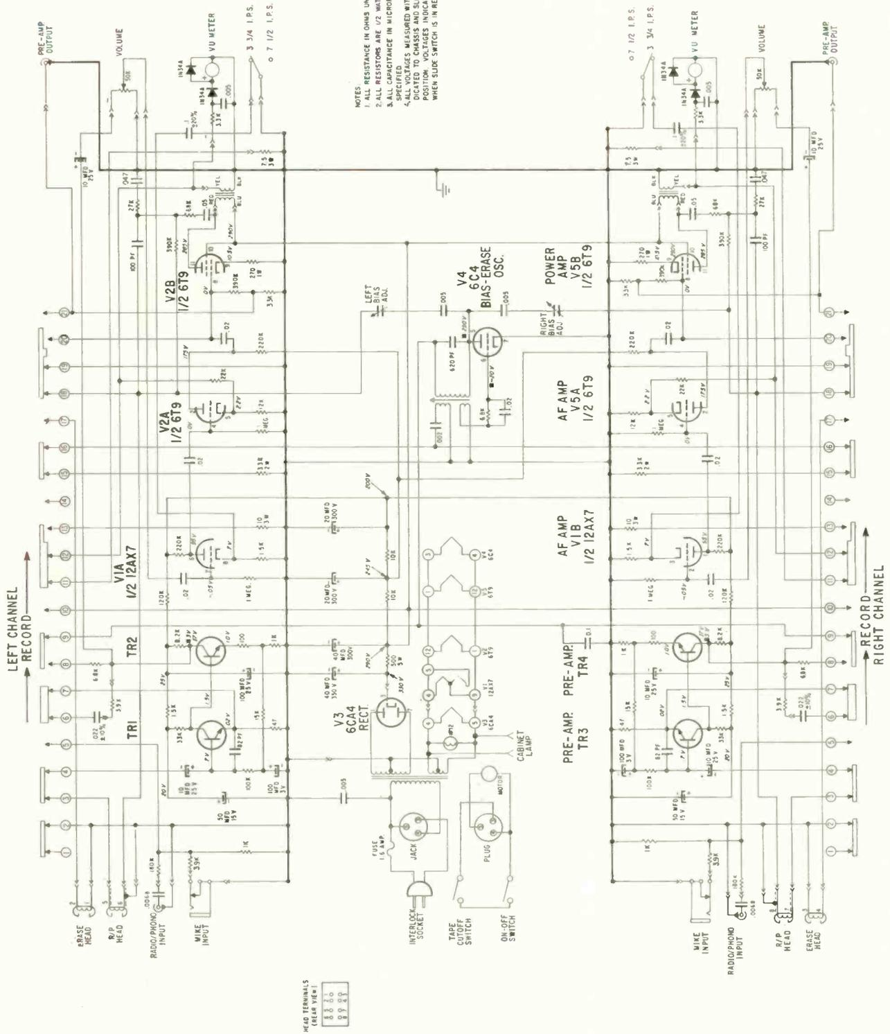
Fig. 1—Schematic of Zenith 81Z stereo and monophonic hybrid tape recorder.
