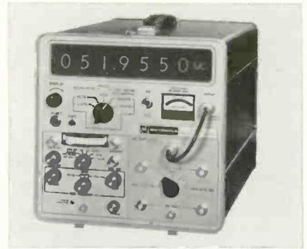
plays a seven digit in-line read-out with four automatic decimal points and indicates whether the read-out is in Hz, kHz or MHz. Motorola.
