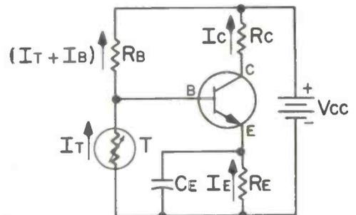
Fig. 10—Thermistors compensate for transistors over limited temperature range.
