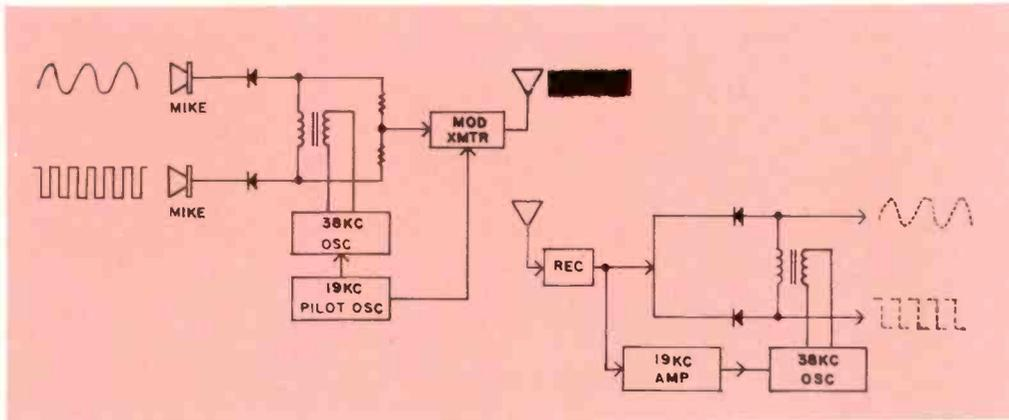
Fig. 3—The complete stereo system shows the relationship of all signals.
