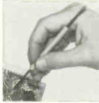
This very small size soldering aid is designed for sub-miniature work in the electronics field. The blades are made of a non-magnetic steel to which solder will not adhere and are set firmly into a hex shaped turquoise plastic handle. The over-all length is 6 in. with a handle 1/4 in. dia. by 3 in. long. Net price 75¢. Hunter.
