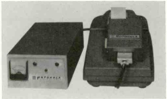
Central office equipment in the Motorola remote alarm system includes the digital decoder (on left) and printer (right). Signals transmitted from remote location are received by base station, decoded by the decoder and printed out five times on tape by the printer.
