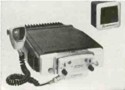
sitivity and  $\pm 2 \times 10^{-6}$  stability. The transmitter has an RF output of 110w. Radios with one, two or up to four-frequency capability can be provided for individual systems. Motorola.
