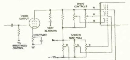
The blanking pulse is also amplified by each triode and serves to blank the CRT at the horizontal scanning rate. The blanking pulse is negative-going at the CRT grids since a signal inversion does not occur in a cathode-driven amplifier.
