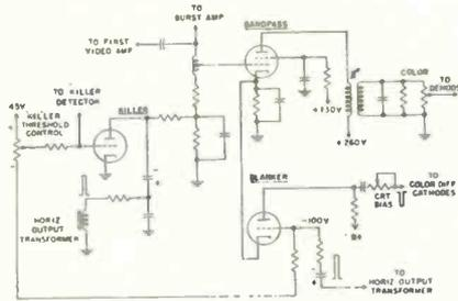
bandwidth on each side of the 3.58Mc sub-carrier. The 3.58Mc burst signal must also be extracted for synchronizing purposes. These frequencies are coupled through an 18pf capacitor to the chroma circuits. The small size of the coupling capacitor allows the chroma information to pass but
