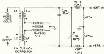
tion is needed at points "A" and "B" toward the outer edges of the picture tube screen. The top- and bottom-pin-cushion corrector circuit consists of a two-current generator connected in series with the vertical coils of the deflection yoke.
