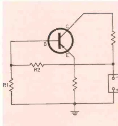
Fig. 2—Voltage divider bias circuit.
