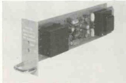
equalization control is provided to compensate for tape head response variations. The output impedance is reportedly less than 10% of normal load with 20Hz to 20kHz power bandwidth. Weight, 18oz. Dimensions, 1.6 x 3-15/32 x 11in. Melcore.
