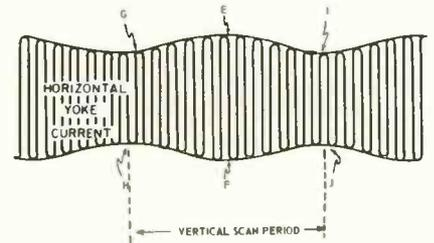
inductively coupled to T108's secondary winding where it will shock excite the series resonant circuit, causing it to ring at 15,750 Hz. The correction voltage fed to the deflection yoke's vertical windings is the voltage that appears across C141 and R176. This ac voltage will cause the vertical yoke current to vary slightly at a horizontal rate.
