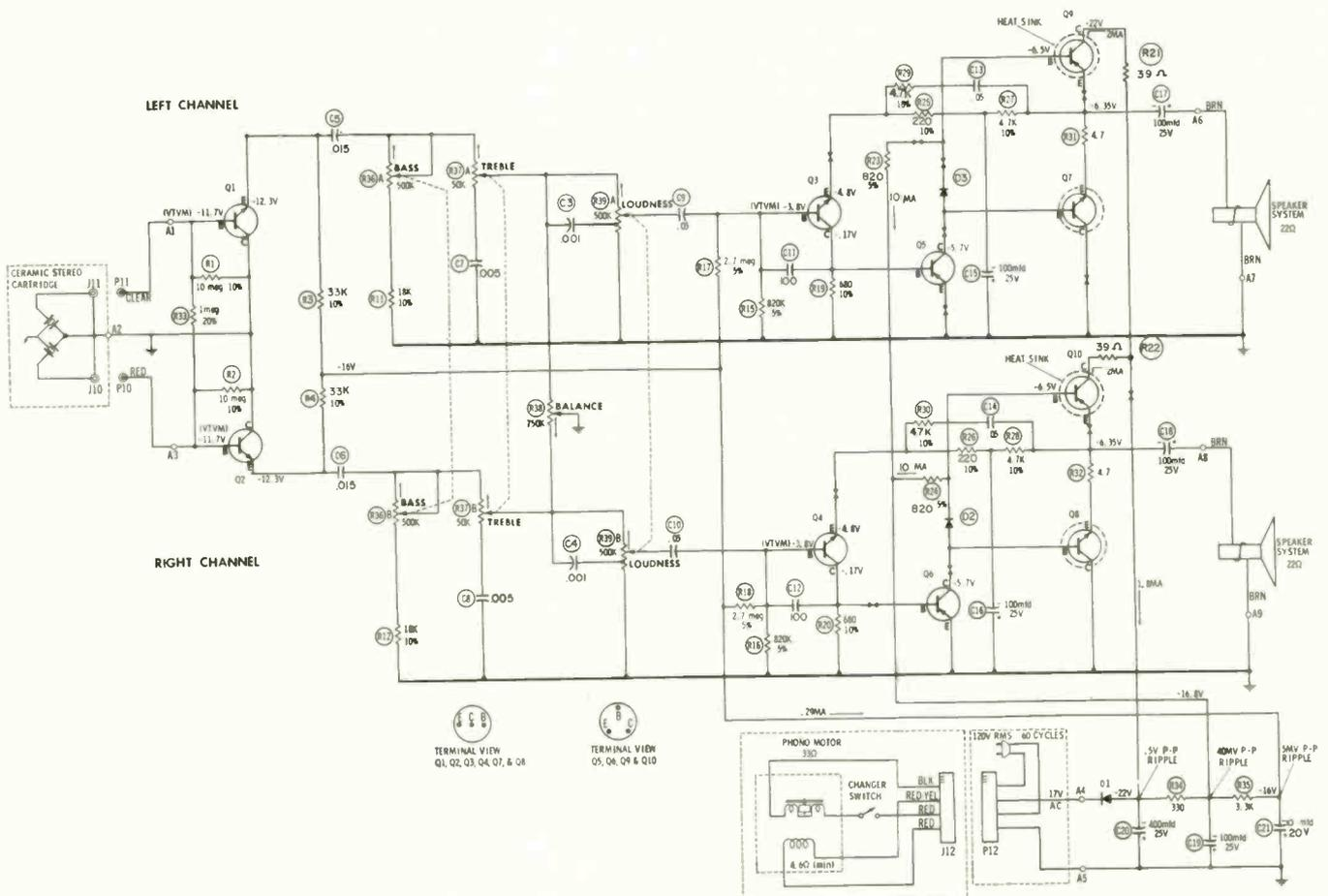
Fig. 5—Schematic of T2C solid-state stereo phono amplifier.
