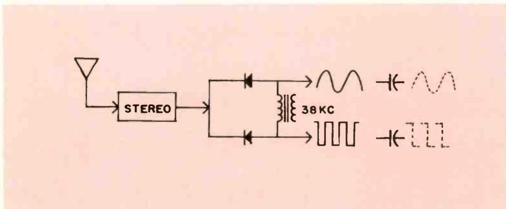
Fig. 2—The stereo receiver functions to re-direct left and right signals to their respective channels.
