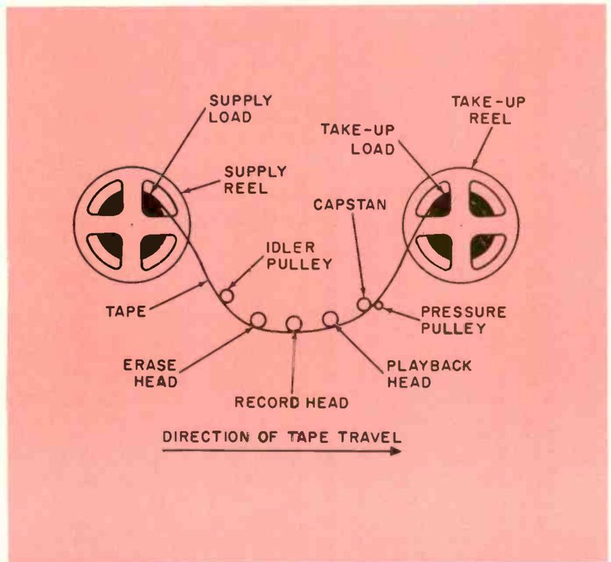
the drive to both reels—supply and take-up — and the pulleys are made so the take-up reel will move slightly faster than necessary at the innermost edge of its diameter. The spring tension allows slippage so the reel can rotate only at the speed of the tape past the capstan. Drive to the supply reel is generally released from the main drive and the spring slippage acts as a drag since the drive pulley is anchored.
