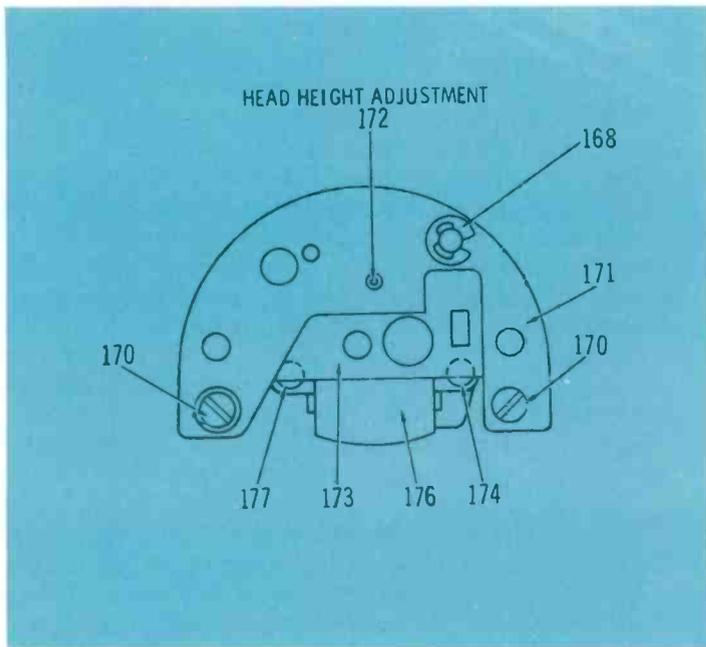
Fig. 3—Head assembly adjustment points.
