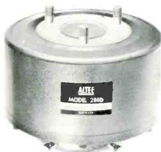
reinforcement and paging systems. The 288D may be used with any of the Altec multicellular horns and is said to provide a response from 500Hz to 16kHz. It has a 16 Ω impedance and is therefore adaptable to all existing Altec power amplifiers. Altec Lansing.
