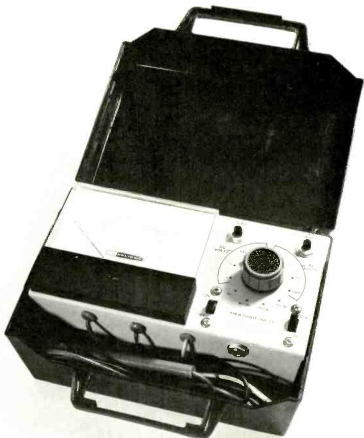
Heathkit Model IM-17 Solid-State Voltmeter.
