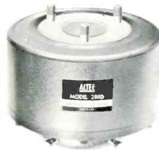
reinforcement and paging systems. The 288D may be used with any of the Altec multicellular horns and is said to provide a response from 500Hz to 16kHz. It has a 16  $\Omega$  impedance and is therefore adaptable to all existing Altec power amplifiers. Altec Lansing.
