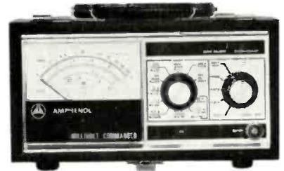
The new Model 870 Millivolt Commander from Amphenol is a low-cost, field-effect transistor instrument; it's designed with the needed low ranges for servicing transistorized equipment. Never before have such sensitive measuring capabilities been available in an instrument under \$100.
