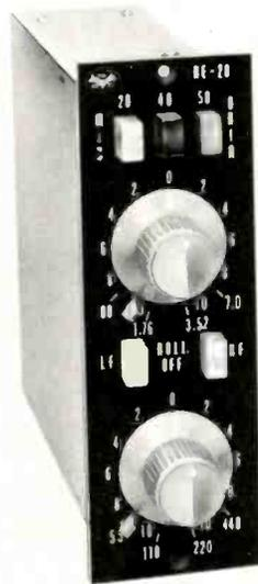
use. The preamplifier portion is said to have a low noise transformer input stage with variable gain switching of 20, 40 and 50db. The equalizer employs a bridged tee notch filter switched from the feedback loop to the input for boosting or dipping at the selected frequency.
