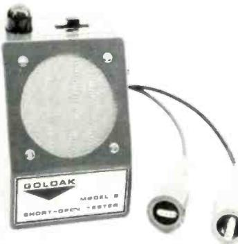
the equipment or operator in the event that the leads are placed across a source of high voltage. The model 8 is said to completely eliminate the use of buzzers and ohmmeters and continuity is indicated by a 600 cps tone from the speaker in addition to a light for visual indication. A separate Tel-tone signal provides individual circuit identification in conjunction with a loud speaker or headphones. Power is supplied by two standard 1½ v "D" cell batteries. Weight 18oz. Goldak.
