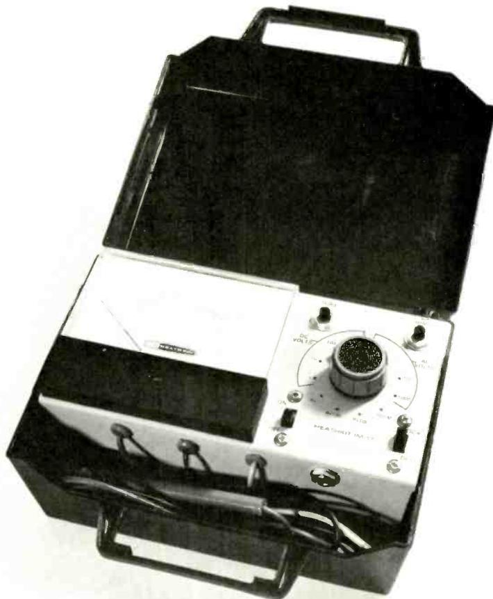
Heathkit Model IM-17 Solid-State Voltmeter.
