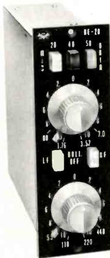
use. The preamplifier portion is said to have a low noise transformer input stage with variable gain switching of 20, 40 and 50db. The equalizer employs a bridged tee notch filter switched from the feedback loop to the input for boosting or dipping at the selected frequency.
