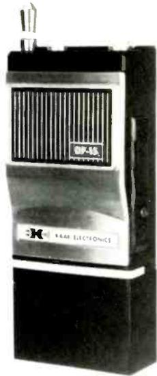
for 12db SINAD. Adjacent channel selectivity is indicated at better than -80db for 20db quieting. The unit contains plug-in block circuitry to provide quick and easy maintenance; average repair time is said to be 8min. The transceiver has a built-in telescoping antenna with provision for a flexible whip or railroad spiral antenna
