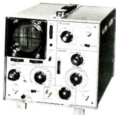
with the trigger level and sweep expansion controls, the waveform's smallest details can be carefully studied. Calibrated sweep provides time-frequency measurements that are accu-
