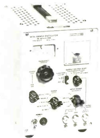
Thermistor stabilization in conjunction with negative feedback is said to achieve a good waveform, good stability (better than 0.1%) and signal amplitude uniformity within  $\pm$  db (ref. 1kHz) over the entire frequency range without resetting the level control. Three outputs are provided direct,
