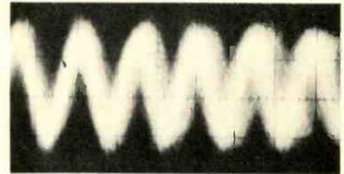
Fig. 11. Output of the ratio detector at points A and B, Fig. 9.
