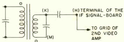
filled capacitor was added between the (K) terminal of the vertical output transformer and the (H) terminal of the IF signal board.
