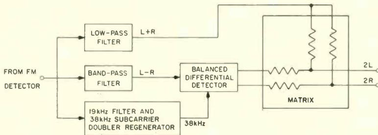
Fig. 3. Block diagram of a matrix type FM receiver.
