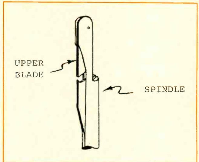
To dissolve the rust inhibitor particles, wipe the spindle with a soft cloth soaked in alcohol. Check the movement of blade for correct vertical travel; it must fall freely of its own weight. See illustration.
