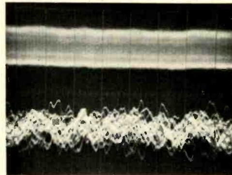
Fig. 14. The top trace shows the signal at the cathode of CR301 (Fig. 10.). The bottom display is the audio output taken at point D in Fig. 9.
