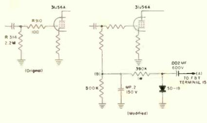
—40v. When the shunt regulator is not working, the voltage of point (A) increases. This voltage increase at point (A) causes the minus voltage at point (B) to increase.
