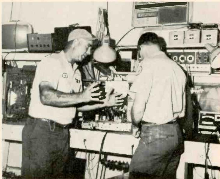
Reduce call-backs and get the best in performance by checking the cathode current of horizontal output tubes
