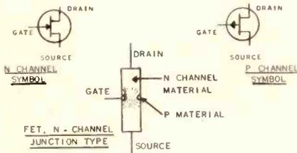
arrow points in on the Gate for the N-channel type. FETs normally operate with reverse bias like a vacuum tube. The amount of reverse bias required to stop electron flow through the FET is called the Pinch-Off Voltage.
