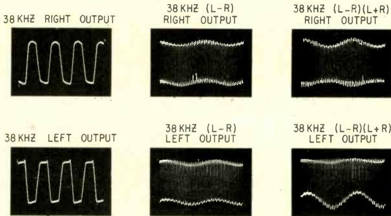
Fig. 2. Output of balanced modulator shows left and right channel outputs with 38kHz carrier.
