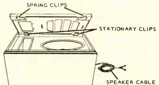
A dull-edged knife blade can also be used, but use care to avoid scratching the cabinet. The speakers are mounted from the front of the baffle board and sealed with caulking compound. The crossover network is mounted inside the cabinet. Therefore, the bass speaker must be removed to gain access to the network.
