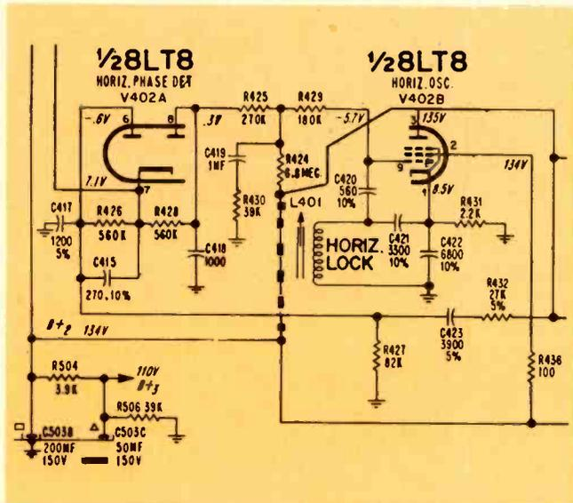
end of R424, which is now connected to B+2, to the plate of V402B, the oscillator. This modification will provide more starting current. This revision has been made in production.
