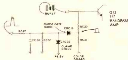
put transformer. The positive pulse will forward bias CRC19. CRC32 has its cathode connected to a 6.5vdc source causing horizontal pulses over 6.6v to forward bias it. The pulse amplitude above 6.6v is clipped off and is not passed by CRC19. The pulse that gets to the base of the 1st bandpass amplifier is sufficient to turn on the transistor.
