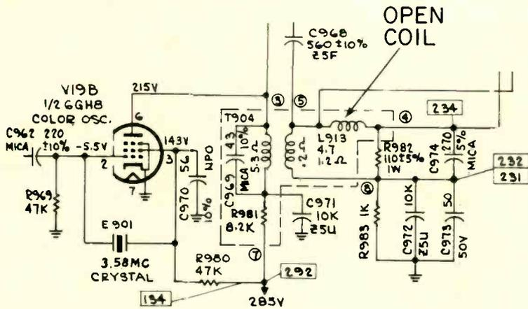
Fig. 1--Partial schematic of Motorola's TS908/Y color chassis showing open reference coil which caused no green color.
