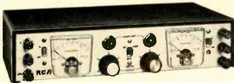
The RCA WP-700A and WP-702A Power Supplies are extremely reliable, solid-state, constant voltage DC power supplies that provide 0 to 20 volts dc at current levels up to 200mA. WP-702A is actually identical to WP-700A, except it is a dual unit with two complete power supply sections. WP-700A IS ONLY \$40.00\* in quantities over five, and WP-702A IS ONLY \$73.00\* in quantities over five. Prices on less than five units are \$48.00\* and \$87.00\* respectively.
