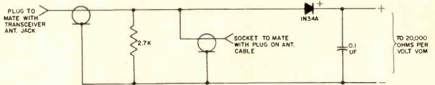
Schematic diagram of peak reading probe.
