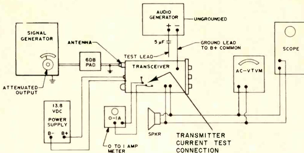
Block diagram of test instrument connections for receiver troubleshooting and alignment.
