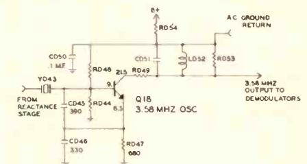
The inductance of the crystal itself with CD41, CD45 and CD46 forms an oscillator tank circuit which resonates at 3.58MHz. Working together, these components comprise a step-up effect between emitter and base. Since the base-emitter circuit of Q18 behaves as an oscillator, the emitter-collector circuit will amplify the 3.58MHz base signal.
