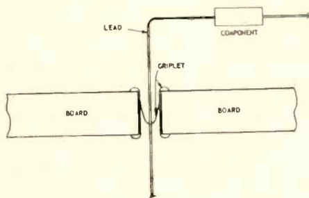
Fig. 1--The "Grip-let," similar to an eyelet, has a grip inside holding components during the solder operation at the factory.
