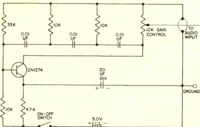
Schematic diagram of simple audio generator.
