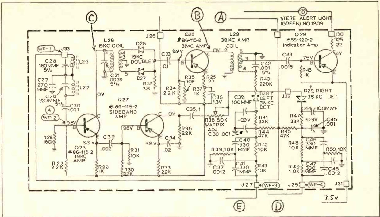
Fig. 9. Multiplex circuit of the matrix type.
