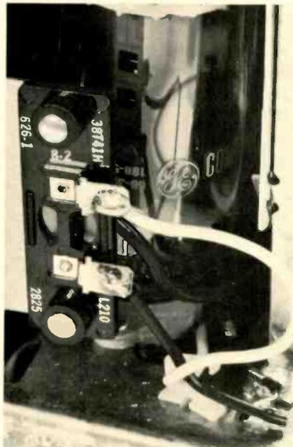
rectifier diodes. CR110 functions from the potential existing between terminals 1 and 3. Current flow for one half cycle would then be from terminal 2 through CR110, RL2 and CR107 to terminal 4. In like manner on the other half cycle, current flows from terminal 3 through CR109, RL2 and CR105 to terminal 1.
