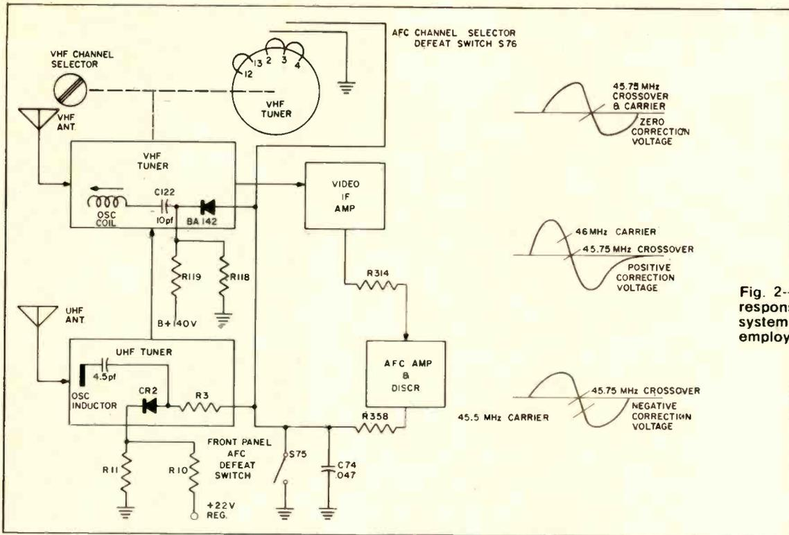
Fig. 2--Block diagram and response curves of the AFC system employed in the KE chassis.
