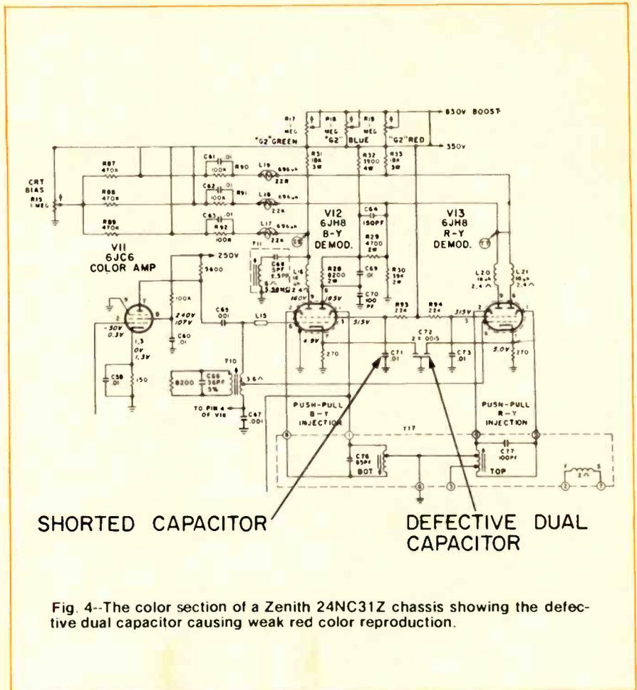
Fig. 4—The color section of a Zenith 24NC31Z chassis showing the defective dual capacitor causing weak red color reproduction.
