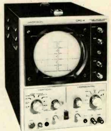
Acceleration voltage is 1500v and horizontal sweep-frequency range is 5Hz to 500kHz. In addition, it is a complete vectorscope with inputs at the front panel and with truly simplified vector-scope calibration facilities to insure the all important horizontal/vertical vector-scope pattern proportions. Rear inputs include Z-axis modulation and direct access to the deflection plates. Instruction manual includes extensive applica-
