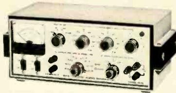
range continuously variable from 1Hz to 100kHz using one multiplier, two selector switches and a vernier control. It features eight output voltage ranges from .003 to 10v RMS with an external load of 10K or more, and six output ranges from .003 to 1v RMS (-62 to +22 db) using the built-in 600Ω load on an external 600Ω load.
