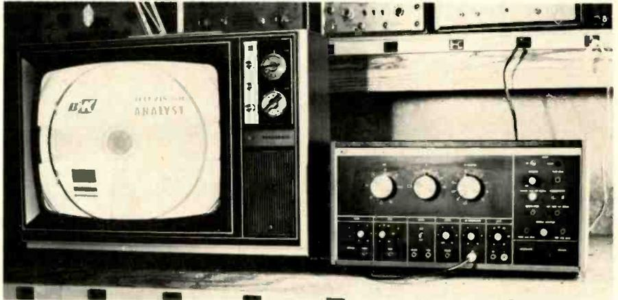
B&K Model 1077 television analyst, showing test pattern produced.
