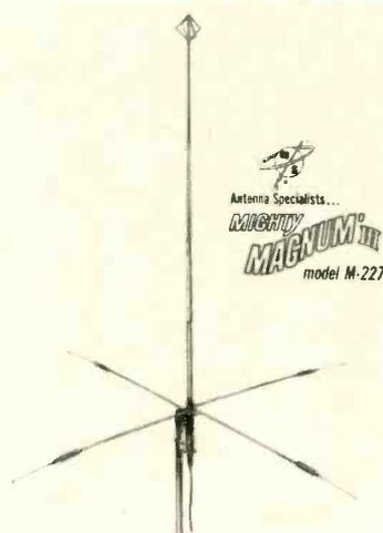
loading coils which electrically lengthen the radials to a full  $\frac{1}{4}$  wavelength thus producing a low radiation angle and a claimed 4db of omnidirectional gain. Other construction features include a waterproof coax connector jacket, chemically welded dual phasing coil jacket, and double-interlock dipole joints. The VSWR is rated at 1.05 to 1 at centerband and 1.4 to 1 at the band edges. List price is \$36.95. Antenna Specialists.
