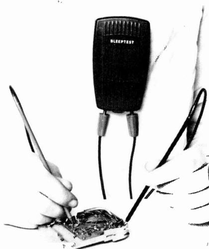
in a wide variety of production, maintenance and laboratory activities. Confirmation of a circuit continuity is obtained by an audible tone generated by a sonic signal generator. The unit as an indicator provides a low energy level through the circuit under test.
