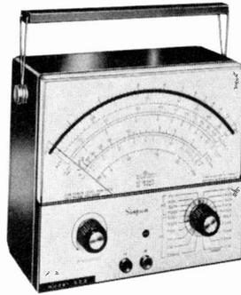
Introduced is the Model 202 ACCU-LOG VOM reportedly eliminating the need to keep readings at the high end of the scale, or worry about "percent of full scale" accuracy readings. The quasi-logarithmic scale gives consistent "percent of reading" accuracy reportedly at  $\pm 2$  percent for dc values and  $\pm 3$  percent for ac values. Zero adjustment is made on a linear portion of the low end of the scale.
