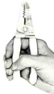
holes that are reportedly accurate and clearly marked. The cutting blade is 1/2in. long to allow cutting of copper and aluminum conductors up to No. 6 wire, also UF and Romex cable with a single snip. The nose of the tool is pointed to reach into confined areas and can also be used for reaming 1/2 and 3/4in. conduit. The handles have plastic grips and a wide span. The two halves are assembled with an adjustable "Sta-Fast" hinge bolt. Over-all length is 6in.; weight 4 oz. Holub.
