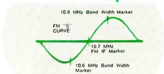
You won't be stopped with just TV alignment. You can align the IF amplifiers of the FM receivers with the 10.7 MHz crystal for maximum as indicated in service manuals. Then, throw on the scope and sweep the amplifiers and view the "S" curve if you have stereo. Two markers, 100 KHz above and below the 10.7 MHz mark the limits of the curve for good stereo. You can align the front end of the receiver too. Competitive units cover only the IFs and you find the job only half done.
