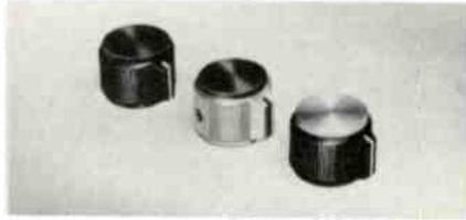
natural aluminum body with black top, and black anodized body with natural color top. Outside body diameter is 0.750in. and has a 1/4in. shaft diameter. This series includes 6-32 set screws in two places. The knobs
