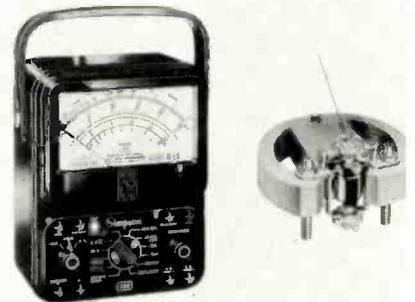
a change in repeatability of less than 0.2%. The taut band movements withstand moderate shock and vibration which cause errors in pivot and jewel instruments. The response of the taut band meters reportedly offers smoother operation and eliminates noticeable overshoot. These Volt-Ohm-Milliammeters come in a broad variety of ranges and accuracies with Add-A-Tester Adapters
