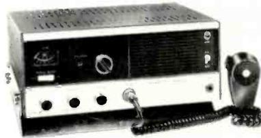
S/Prf meter, variable squelch control, TVI trap, external speaker/phones jack and a jack for Priva-Com private call unit. The unit employs 11 tubes, 2 transistors and 11 diodes. It is supplied with all crystals, vari-tilt mobile/base mounting bracket and ceramic push-to-talk microphone. Exterior design is brushed aluminum, gray and black. The unit measures 12w x 8 1/2d x 5in. h. Lafayette.
