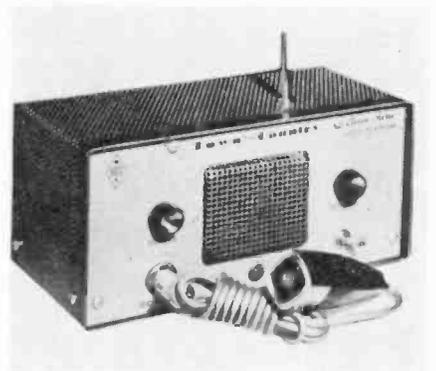
circuit minimum measurements of 3.25 watts over a 50 ohm non-inductive load; press-to-talk operation; and automatic squelch. Price, complete with 1/8th wave whip, microphones, crystals, and printed forms and brochures, \$159.50. Utica Communications Corp., 19 S. LaSalle St., Chicago 3, Ill. (ELECTRONIC TECHNICIAN 1-7)
