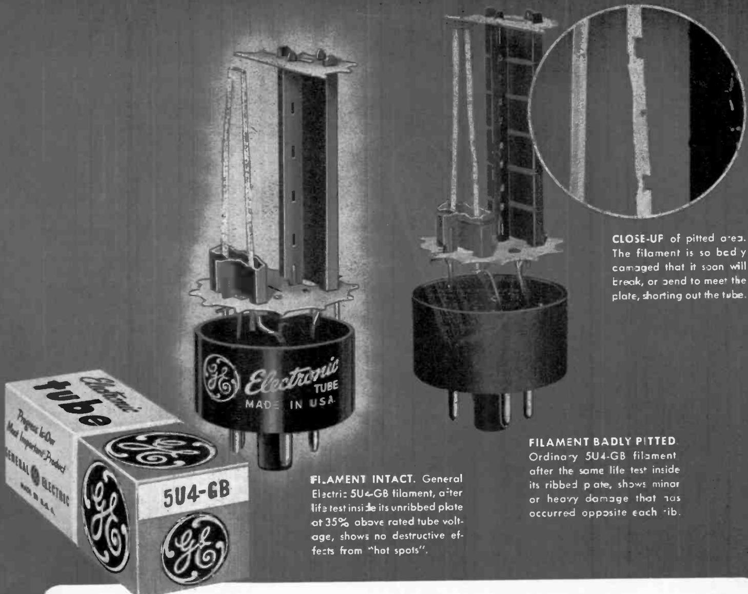
**CLOSE-UP** of pitted area. The filament is so badly camaged that it soon will break, or bend to meet the plate, shorting out the tube.
