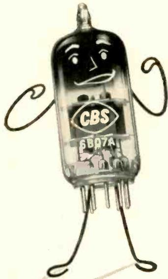
"All 6BQ7A's used to have folded heaters . . . and gave you plenty of trouble. Now, all of us CBS 6BQ7A tubes have new coil heaters for our new improved cathodes . . . and *you* don't have heater burnouts, shorts or slumping gain."
