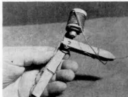
Fig. 3—Clothespin holder makes a handy solder dispenser and serves as "3rd hand."
