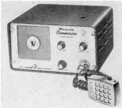
nel class D citizens band. It features the same audio circuitry as the ED-27, and has an improved transmitter. The receiver is a crystal-controlled double-conversion superheterodyne with a selectivity of 5 kc at points 6 db down and a sensitivity of  $\pm 0.3$  mv. \$189.50. Vocaline Co. of America, Old Saybrook, Conn. (ELECTRONIC TECHNICIAN 4-5)
