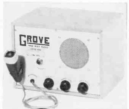
ohms antenna impedance; superregenerative receiver with r-f amplifier; tuning range of 26.5 mc to 27.5 mc; full 2½ watts audio output; and 4" speaker. Available in 3 models: G-110 (110v); G-12 (12v) and G-6 (6v) \$39.95. Grove Electronic Mfg. Co., 4103 W. Belmont, Chicago 41, Ill. (ELECTRONIC TECHNICIAN 4-2)
