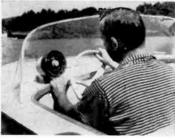
Fig. 1—Depth finder may be mounted in open cockpit boat.
