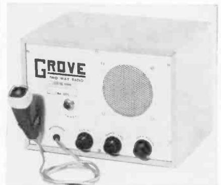
ohms antenna impedance; superregenerative receiver with r-f amplifier; tuning range of 26.5 mc to 27.5 mc; full 2½ watts audio output; and 4" speaker. Available in 3 models: G-110 (110v); G-12 (12v) and G-6 (6v) \$39.95. Grove Electronic Mfg. Co., 4103 W. Belmont, Chicago 41, Ill. (ELECTRONIC TECHNICIAN 4-2)
